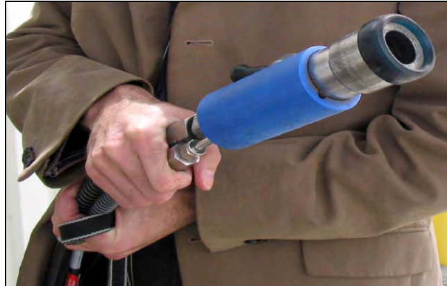
Figure 23. Compressed Hydrogen Fuel Nozzle Photo courtesy of Santa Clara Valley Transportation Authority.
