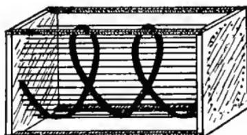
FIG. 12. — PRIMARY OF OSCILLATION TRANSFORMER.
