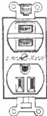
reset and test buttons
