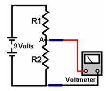
What is the voltage at point 'A'? If you feel like saying "Who cares?" then the answer is "you" if you want to understand how circuits work, because the voltage at point 'A' is vital. For the moment, ignore the effect of the voltmeter used to measure the voltage.
