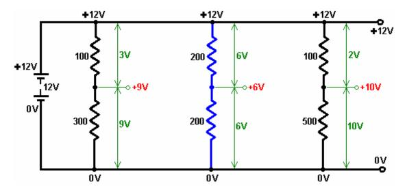
The same division of the supply voltage can be produced by positioning the slider of a variable resistor at different points by rotating the shaft of the device:
