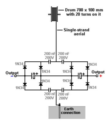
As can be seen, the addition is of four diodes and two capacitors. Presumably, using BYV27 diodes rather that 1N34 diodes would create a further enhanced output.
