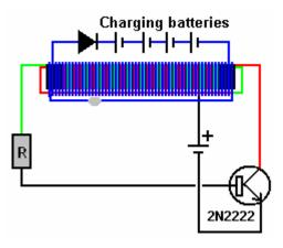
Current drawn from the second winding does not affect the current draw of the drive battery which is running the circuit.
