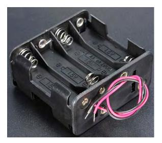
The battery box can be adapted to hold seven batteries rather than the intended eight batteries, producing a nine volt battery pack with 1.2V batteries. If three of these battery packs are used with the solar panel, then there is no need for over-charging protection as NiMh batteries can deal with overcharging current if it does not exceed 10% of the battery's milliamp-hour rating, and that simplifies the design very considerably.
