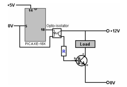
Here a high output voltage on pin 10 of the PIC chip lights up the LED inside the opto-isolator chip, causing a major drop in the resistance between the other two pins. This causes a current controlled by the resistor "R" to be fed into the base of the transistor, switching it on and powering the load.
