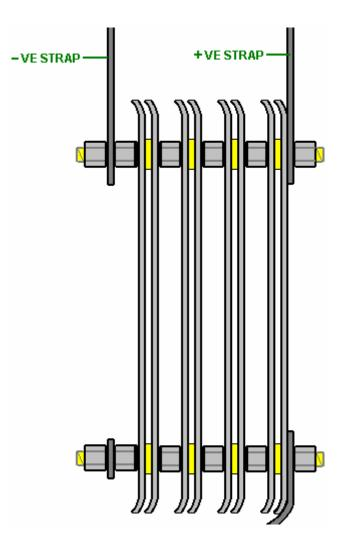
So, a compromise is reached where the current flow around and past the plates is combatted by strategic spacing of the plates:
