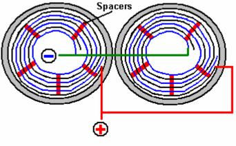
**CELLS ARE WIRED IN PAIRS (Top View)**
