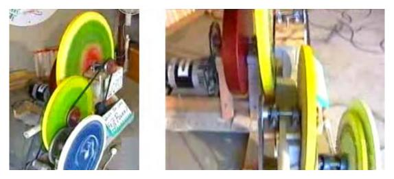
The final shaft drives a standard electrical generator and Chas found that he could power electrical equipment from that generator, electrical mains equipment which required greater current that his mains-driven motor did.
