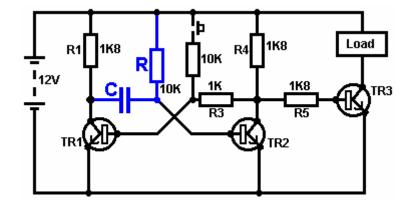
In this circuit, the ' $\mathbf{R}$ ' resistor and the ' $\mathbf{C}$ ' capacitor values determine how long the monostable will be in its unstable state. The circuit operates like this:
