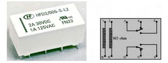
This is the electromechanical equivalent of a manual two-pole changeover switch. A brief pulse of current through the relay coil connected between the relay pins 1 and 16 locks the relay switch in one position while a brief pulse through the coil connected between pins 2 and 15 locks the switch in the other position. The current drain on the circuit would be almost zero.
