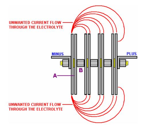
This diagram shows the way that the plates are connected. The red lines show paths of unwanted current flow which produce almost no gas. This wasted current flow is opposed by the useful current flow across gap "**A**" in the diagram.
