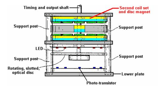
The coil switching with the additional layer of coils is shown here:
