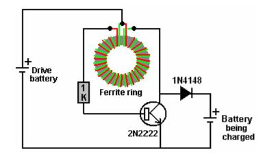
In this arrangement the LED is replaced by an ordinary diode (almost any diode will do) and the incoming power fed into a rechargeable battery. I have used this circuit to recharge a 2285 milliamphour AA size battery from 0.6 volts to 1.41 volts in one hour without running the drive battery down by any significant amount.
