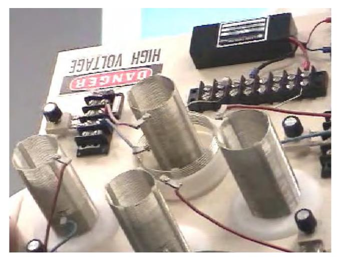
The secondary coils are constructed using Barker & Williamson's normal method of using slotted strips to hold the tinned, solid copper wire turns in place.
