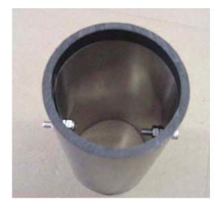
Note that the shimstock is flush with the bottom of the tube. Final assembly for the electrodes. Note that the capscrews each have stainless steel nuts inside the barrel to seat to the shimstock. The screw on the left will be used as the Negative battery connection to the cell while the screw on the right merely seats the shimstock.
