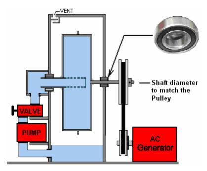
While the axle shaft can be made of two parts welded together and welded to the drum, I suggest that it is more practical to weld the incoming three-inch diameter pipe to the drum and then, choosing a bar diameter which matches the size needed for your chosen pulley wheel, that bar is welded to the other side of the drum as shown above. The part of the axle on the right of the drum is solid and provides the drive to the generator:
