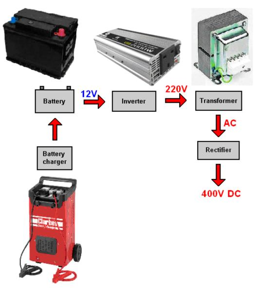
The transformer shown here is not at all easy to find as very few people want to produce 400 volts DC from 220 volts AC. One important point here is the "battery charger". It needs to supply hundreds of watts of electrical power back to the input of the inverter continuously in order to make the system self-powered. Consequently, it needs to be a professional level unit so heavy that it needs wheels and a handle to move it around.
