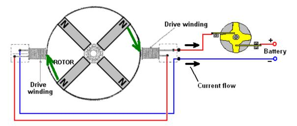
Notice that the movement of the rotor is caused by the permanent magnets being attracted to the iron cores of the drive electromagnets and **not** by any electric current. The electric flow is going back into the battery and is being caused by the movement of the rotor which in turn is being caused by the permanent magnets.
