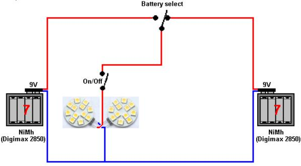
With this arrangement either battery can be selected by the top switch and the light turned on or off using the lower switch. However, it is important to select the right components for every part of this circuit. AA size batteries are used. The batteries chosen are important because there is an enormous difference in battery performance when tested under an actual load, so pick Digimax 2850 batteries:
