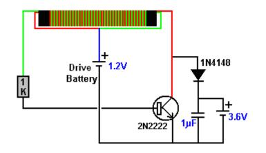
With the battery on charge removed, the voltage on the capacitor reaches 22 volts. Charging the same batteries with this circuit reached 4.14 volts and produced load results of 4.09, 4.05, 4.01, 3.98, 3.96, 3.93, 3.90, 3.88, 3.85, 3.83, 3.81 and 3.79 volts after 12 hours which is much better than the 5-hour total previously experienced. However, obviously, something better is needed.
