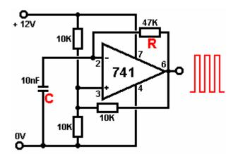
The rate of oscillation of this circuit is governed by the Resistor marked ' $\mathbf{R}$ ' in the diagram and the capacitor marked ' $\mathbf{C}$ '. The larger the resistor, the lower the rate of oscillation, the larger the capacitor, the lower the rate of oscillation.
