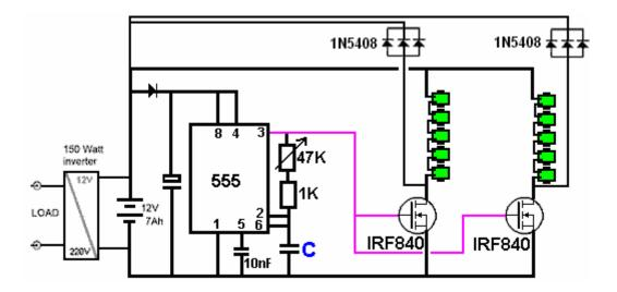
This arrangement allows for considerable alteration of the operating frequency by merely turning a knob. Experienced constructors will have their own preferred methods of construction, but we might choose to use a layout on an open board in order to make it easy to see what is happening and to give good cooling during the development stage, perhaps something like this:
