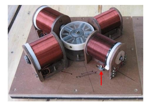
Notice the way that the coil mounts allow the distance between the coils and the rotor to be changed. The working gap between the rotor and the coils can be adjusted so that the performance can be maximised by finding the most effective gap.
