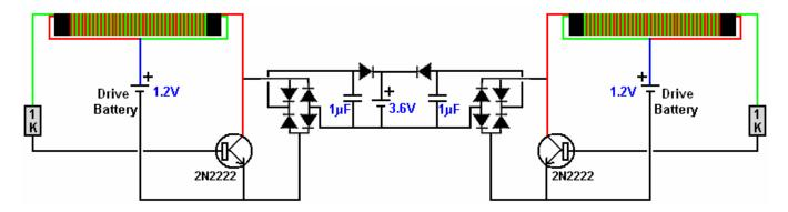
There is no need to restrict the battery on charge to a nominal 3.6 volts in any of these circuits as a single 1.2 volt drive battery can easily charge a 4.8 volt battery or larger. The value of the capacitor has a considerable effect and I suggest a one microfarad capacitor is a good choice. It has been argued that the two additional diodes on each side of the battery being charged are not necessary, although I have shown them to isolate the two circuits from each other.
