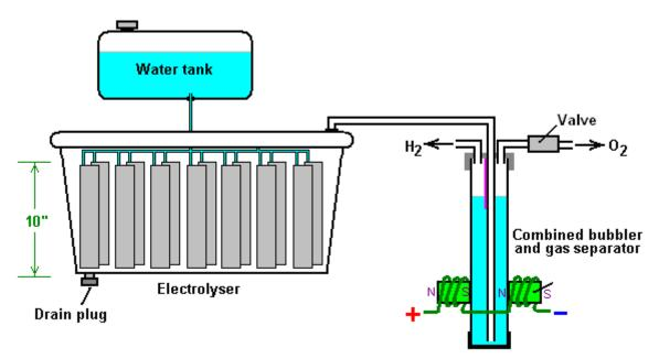
It is possible that seven sets of three or four spirals wired in parallel would be used for larger engines with their 13.8 volt electric systems. Zach uses the very simple method of allowing excess gas to be vented via the oxygen valve if gas production exceeds the requirements of the engine. When operating on a twelve volt system it might be more convenient to use a standard pressure switch which opens an electrical connection when the gas pressure rises above the value for that switch:
