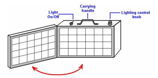
When closed over, the face of solar panel P1 faces that of solar panel P2, protecting both when the unit is being carried. An early prototype of this style of construction with the panels open, looks like this:
