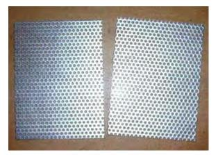
Your local steel supplier probably has some types on hand and can let you see how flexible a particular variety is. The shape shown above is for a "three plate per cell" design where there are two active plate faces. Ideally, you want two to four square inches of plate area per amp of current flowing through the cell, because that gives very long electrode life and minimum heating due to the plates.
