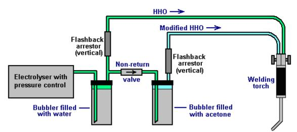
The flashback arrestors are a sand-filled design and so are mounted vertically. The gas production rate is knob controlled using this circuit:
