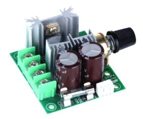
Using a commercial module like this means that no electronics knowledge is needed to build a working generator of this type.
