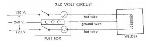
The voltage on a 240V circuit is measured by fastening a lead on the voltmeter to each of the hot wires. Voltage between either hot terminal and the neutral bar will be one-half of the voltage between the two hot wires. The number of amperes flowing can be measured by clamping an ammeter around either of the hot wires.
