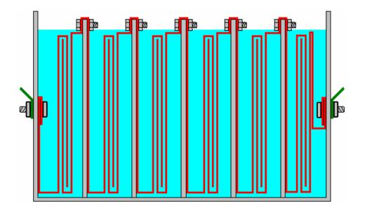
**The electrolyte** is a mix of water and an additive to allows more current to flow through the liquid. Most of the substances which people think of to use to make an electrolyte are most unsuitable, producing dangerous gasses, damaging the surfaces of the plates and giving uneven electrolysis and currents which are difficult to control. These include salt, battery acid and baking soda and I strongly recommend that you do not use any of these.
