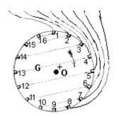
The dotted lines indicate internal electrical connections, so for example, contact 14 is connected to contact 3, but let me stress again that this unit is **not** part of the design and while it is used to "explain" the actual operation, I would not be surprised if it were not intended to misdirect people from the actual operation.
