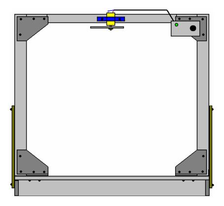
It should be explained that, with the exception of the 25 mm thick plank, all of this construction is only loaded very lightly as rotating the top of the axle shaft does not take much power or effort at all. Almost all of the rotating weight is located at the bottom of the axle shaft and that weight rests on some form of bearing which rests in the middle of the 25 mm plank.
