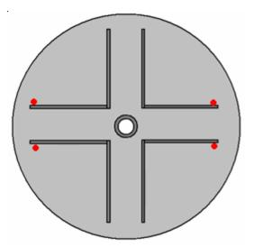
You can then turn the drum over so that all following welding is downwards and you are not liable to get hot metal coming at your hands. There is room to weld inside the drum as the pieces forming the channel walls are only 370 mm long and there is 144 mm of clearance between the drum sides.
