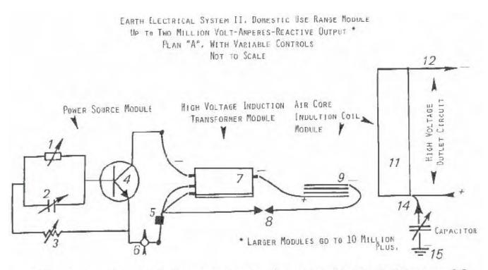
PARTS: 1. COIL. VARIABLE. 2. CAPACITOR. VARIABLE. 3. RESISTOR, VARIABLE. 4. TRANSISTOR, R.F., 5. BATTERY, RECHARGEABLE, 6. OFF-ON SWITCH, VARIABLE, 7. HIGH VOLTAGE TRANSFORMER, 8. FEED BACK WITH SPARK GAP, 9. REACTOR, INDUCTION COIL, 10. FEED BACK WITH SPARK GAP, 11. REACTANT COIL. 12. OUTPUT FOR # 12, 13, INPUT FOR ELEVEN, 14. GROUNDING FOR ELEVEN.
