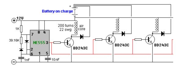
Alexkor uses preset resistors to adjust the base resistors to their optimum values. The simplicity of this circuit makes it very attractive as a construction project and using more than one coil should make for impressive performance figures. Alex says that the best results are achieved with just the one (1000V 10A) diode per transistor and not a diode bridge. Multiple transistor chargers like the one above, work best when there is a separate wire from each coil to the battery being charged.
