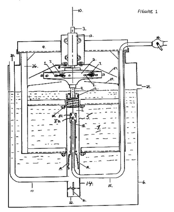
Figure 1 illustrates the invention having thrust-jets 1, rotor 2, power take-off 3, rotor support 4, fluid supply 5, and fluid reservoir 6. Thrust-jets 1 extend from rotor 2 and impart rotational thrust to rotor 2 by ejecting a stream of fluid 7 in a direction indicated by arrow "A" in Figure 4, approximately tangential to the arc described by the rotor's rotational motion.
