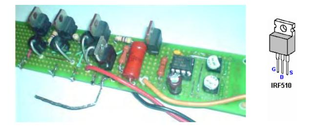
It is possible to use various different high-voltage transistors with these circuits. As some people have difficulty in working out a suitable physical construction for a circuit, here is a suggestion for a possible layout using an MJ11016 high-power high-gain transistor on stripboard.
