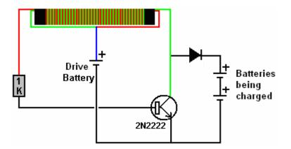
I have used a 1N4148 diode which is a silicon diode with a voltage drop across it of 0.65 or 0.7 volts and it has worked well. However, a germanium diode with its much lower 0.25 to 0.3 voltage drop is generally recommended, perhaps a 1N34A diode. It is also suggested that using two or three diodes in parallel is helpful.
