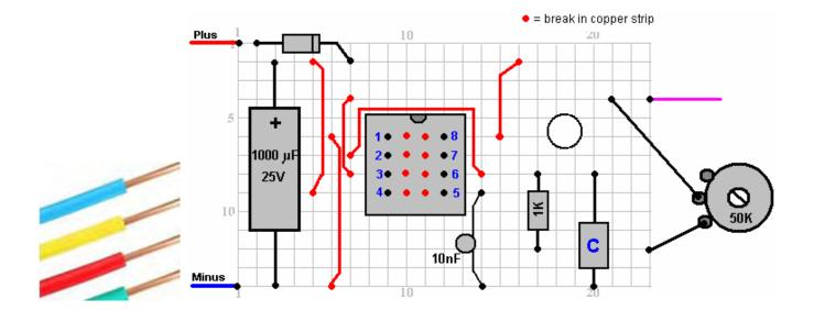
Then work from left to right, mounting the remaining components. The capacitor "C" has got a lot of spare space around it so that it can be altered at a later date if you decide that you should.
