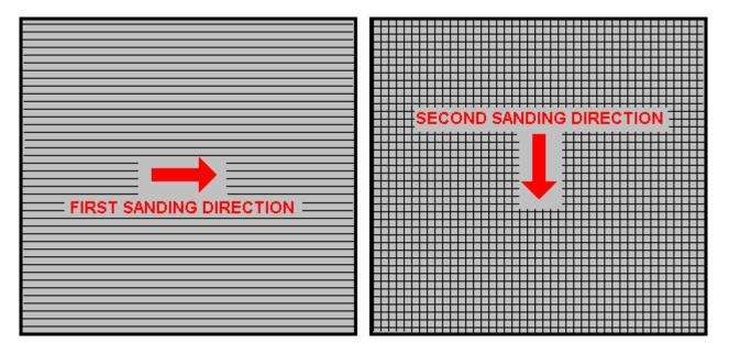
When doing hand sanding the sandpaper is drawn across the plates in **one** direction only and not backwards and forwards, as the backwards stroke always destroys the perfectly good ridges created on the forward stroke. Also, you only need two strokes in one direction before turning the plate through ninety degrees and completing the sanding of that face of the plate with just two more strokes (again, with **no backstroke**).
