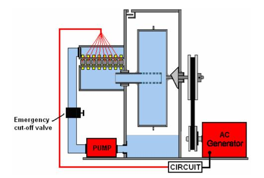
With this arrangement, if the drive belt were to break or the alternator were to develop a serious fault, then the circuit voltage would drop off and as a result, the circuit would no longer supply current to the open valves and they all would close, shutting off the generator which is exactly what is needed.
