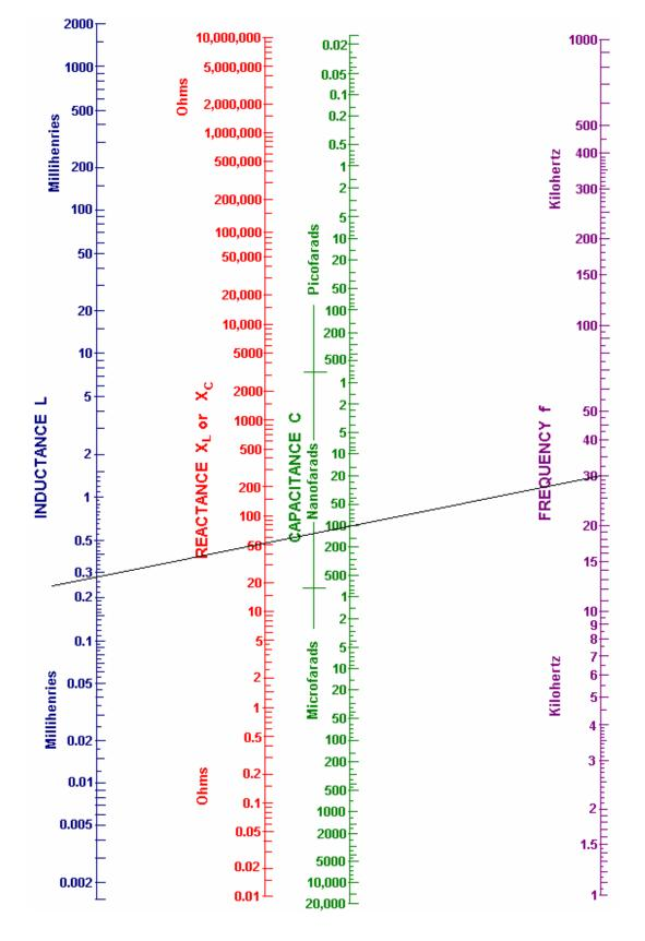
Draw a straight line from your 30 kHz frequency (purple line) through your 100 nanofarad capacitor value and carry the line on as far as the (blue) inductance line as shown above.
