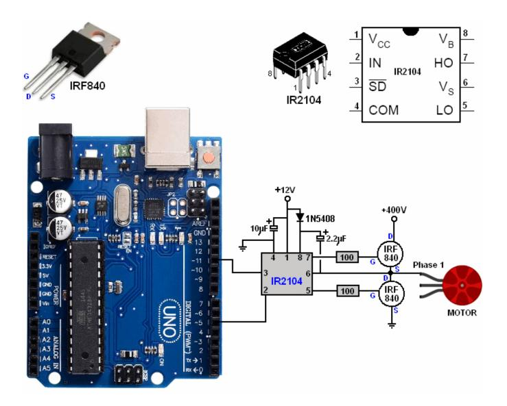
The 1N5408 diode can handle high voltages and so protect the 12 volt section of the circuit from the high voltage section feedback. The power drive for the second phase is:
