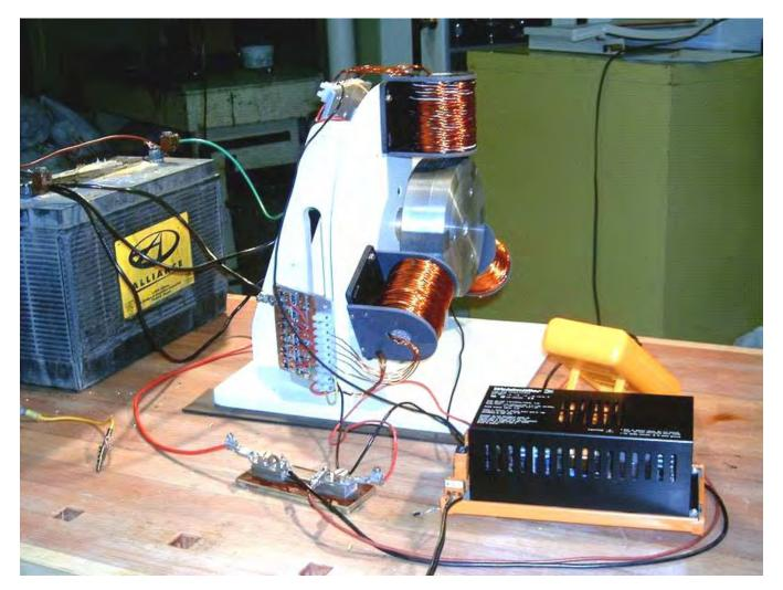
This is not a toy. It draws significant current and produces substantial charging rates. This is how Ron chose to build his device. The rotor is constructed from aluminium discs which were to hand but he would have chosen aluminium for the rotor if starting from scratch as his experience indicates that it is a
