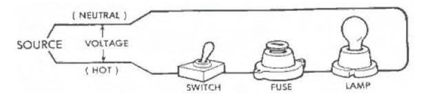
A circuit includes a "hot" wire (red or black) carrying current from the source through a switch, circuit protector (fuse or circuit-breaker), and an appliance. The neutral wire (white) conducts the current from the appliance to the source (ground).
