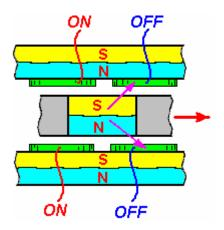
This produces a larger horizontal thrust. While this design goes for optimum performance, I suggest that a much more simple form of construction with a ring of standard circular neodymium magnets could be used instead of one large disc magnet, and ordinary circular coils placed on top of the circular magnets, and this allows large diameter rotors to be constructed, the larger diameter giving greater output shaft power:
