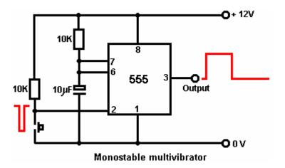
If you are not at all familiar with electronic circuits, then take a look at the beginner's electronics tutorial found in the Appendix as that explains how circuitry works and how to build any simple circuit from scratch. We can use two of these circuits, the first to give the adjustable delay and the second to give a brief pulse to the ignition circuit to generate the spark:
