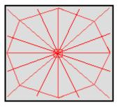
Mark 500 mm from the central point out along each of these new lines and then connect these points to form the 1000 mm diameter 16-sided drum side:
