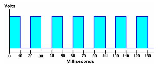
This gives an even waveform, that is, one with a Mark/Space ratio of 50:50 or a Duty Cycle of 50%. If we want the same rate of pulsing but a Duty Cycle of just 25% then the program would be:
