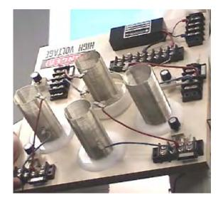
The "L1" short outer coil is held in a raised position by the section of white plastic pipe in order to position it correctly relative to the smaller diameter "L2" secondary coil.
