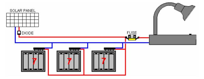
All solar panels have a diode to prevent the panel drawing current from the batteries during the hours of darkness and it is not unusual for the panel to be supplied with a diode already connected in place.
