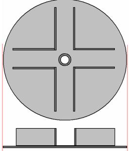
As the drum diameter is 1000 mm and 150 mm is left around the centre and 50 mm is left at each side, the eight internal walls need to be only 500 - 75 - 50 = 375 mm (14.76 inches) long. The 150 mm clearance in the centre of the disc does not need to be exact, and so cutting 370 mm from the 150 mm strip will do nicely for all eight walls.
