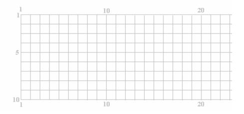
where the horizontal strips are numbered and the vertical lines of holes are also numbered. In this sketch, where the lines cross, represents a hole in the board. The sketch of a possible physical layout can then be prepared and it might look like this when seen from the top although the copper strips on the underside of the board are shown in the sketch:
