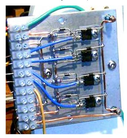
It is important to realise that the collector of a BD243C transistor is internally connected to the heat-sink plate used for the physical mounting of the transistor. As the circuit does not have the collectors of these transistors connected together electrically, they cannot just be bolted to a single heat-sink plate.
