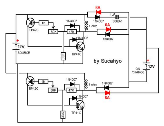
which looks rather complicated with two of the transistors connected upside down and protection diodes connected between transistor collector and base. Sucahyo says that he has used this circuit for four years now without experiencing any surface charge effects.
