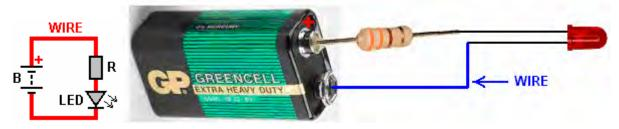
If the LED is connected the wrong way round, it will not damage anything but the LED will not light up. Poor quality connections can be made by twisting wires together. Better quality connections can be made using screw connectors:
