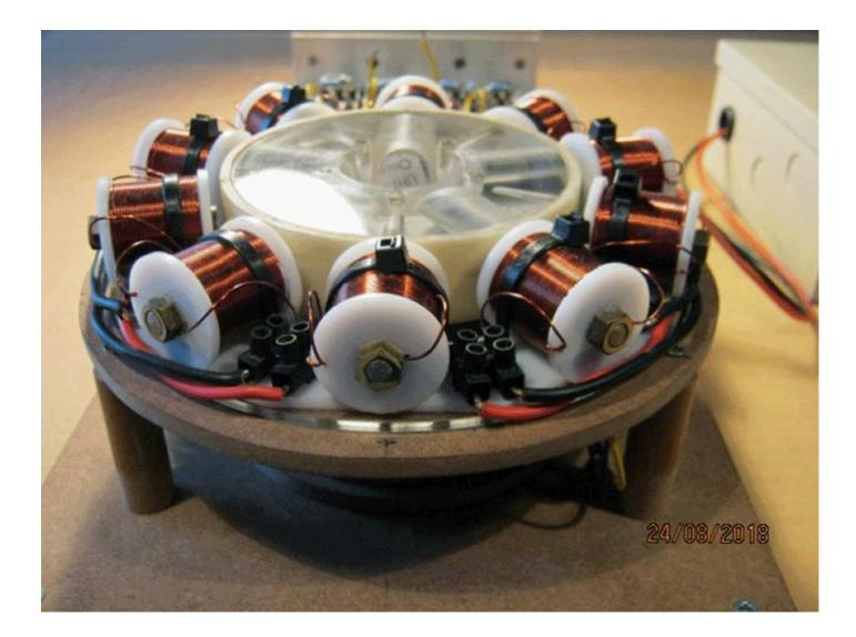
Remember that the coils are mounted on their own support ring and so can be handled as a single unit. This is very convenient.
