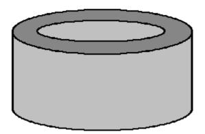
This core is then wound with thick wire – perhaps AWG #10 or 12 SWG ( $2.3 \times 2.3 \text{ mm}$  square wire). The turns of wire should be tight, side by side and sit exactly flat on the top surface as the wire there will be contacted by the sliding brush:
