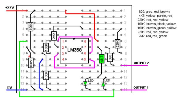
The 4.7K resistor and LEDs are only on the board for testing purposes and when the circuit is built in permanent form, then the LED chain connects to pin 1 of the jack socket so that the LEDs are disconnected during the two hours of daily treatment recommended when using the device.
