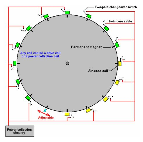
In this particular arrangement, five of the coils gather energy while ten provide the drive. For the sake of simplicity, the diagram shows the five collection coils adjacent to each other and while that would work, the wheel is better balanced if the drive coils are evenly spaced out around the rim. For that reason, this switching would actually be selected to give five sets of two drive coils followed by one pick-up coil as that gives a perfectly balanced thrust on the wheel.
