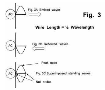
Moving to still shorter wires, the same principle also applies to any wire with a length equal to one half of an AC voltage wavelength. As shown in **Fig.3** (which includes **Fig. 3A** showing an emitted wave, **Fig. 3B** showing a reflected wave, and **Fig. 3C** showing the superimposed "bubbles"), if the wire length is one half of the wavelength, a natural and resonant standing wave will still form, with a frequency which is double the frequency of the input AC voltage.
