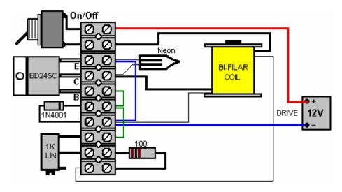
The 1K variable resistor is adjusted to give the best performance and the On/Off switch is optional. More advanced circuits can also be tried and the performance compared. Generally speaking, I would expect a three-rotor version to give a better performance than a single rotor implementation, but experimentation would be needed to verify that.
