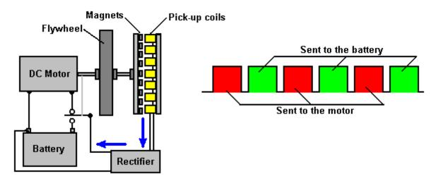
What makes this arrangement different from a standard set-up is that the battery powered motor is not connected directly to the battery but instead is fed with a rapid series of DC pulses. This has two effects. Firstly, that method of driving a motor is very efficient electrically speaking and secondly, when a flywheel is driven with a series of pulses, it picks up additional energy from the local environment.
