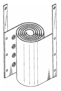
These electrodes are surprisingly difficult to make by hand but they should be very simple to construct using a 3D printer. These electrodes are then bolted to a non-conducting enclosure:
