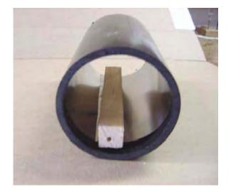
For drilling, use a strip of wood. Be sure that the shimstock is flush with at least one edge of the tube. Use the flush edge as the bottom of the electrolyser.
