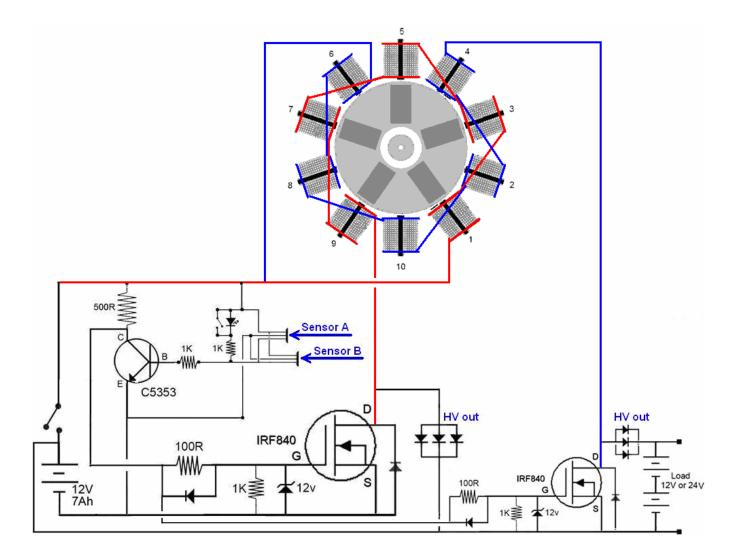
As it stands, this circuit can charge 12V or 24V batteries or power a 12V inverter connected across a 12V battery, or 24V inverter connected across a 24V battery. A version of this circuit with fewer components which works very well indeed is this:
