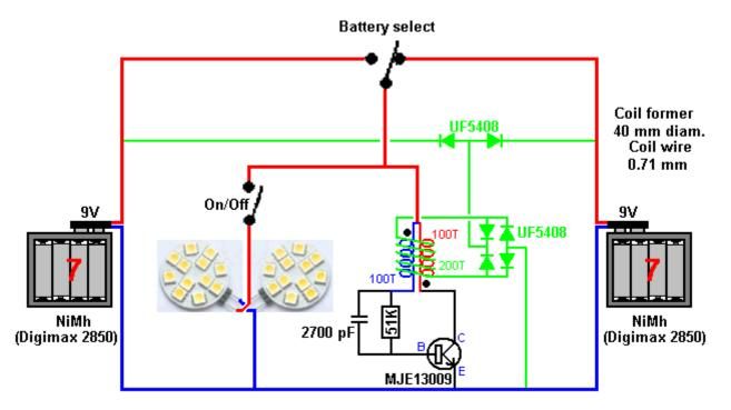
The best performance is when the transistor is a T13009 which is also sold under the name MJE13009. The 2700 pF capacitor is important as is the value of the 51K resistor. If you generally use the more basic series of resistors, then a 51K resistor can be a 47K resistor and a 3.9K resistor in series. The bridge of four UF5408 diodes can be replaced by am RS405L diode bridge if you prefer.
