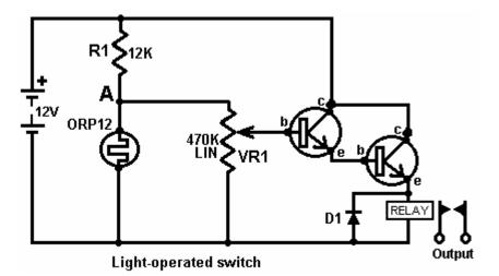
This is almost the same as the light-operated circuit shown earlier. In this variation, the transistors are wired so that they work as an 'emitter-follower' which follows the voltage at point 'A' which rises as the light level drops and the resistance of the ORP12 increases. This causes the voltage across the relay to increase until the relay operates and closes its contacts. A relay is a voltage-operated mechanical switch which will be described in more detail later on.
