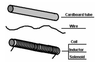
This is a very interesting device with many uses. It forms the heart of a radio receiver, it used to be the main component of telephone exchanges, and most electric motors use several of them. The reason for this is if a current is passed through the wire, the coil acts in exactly the same way as a bar magnet:
