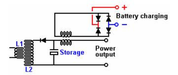
The DC output produced by the four diodes was then used to charge the driving battery, and the power level produced is substantially greater than the minor current drain from the battery. Consequently, it is
