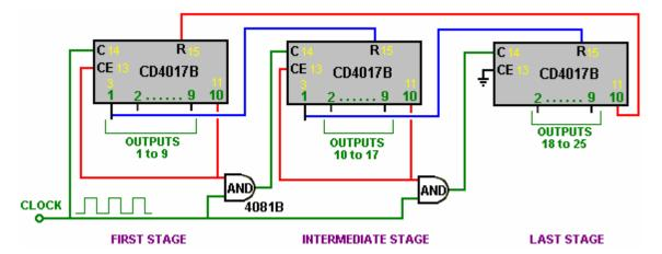
At startup, output 10 of the first stage (which is physical pin 11 of the chip) is at a low voltage. This holds the Clock Enable (pin 13) low, allowing the clock pulses to enter the first stage. Because the output 10 voltage is low, one input to the first AND gate is held low, preventing it from letting the clock pulse flow through it, i.e. the "gate" is closed to through traffic.
