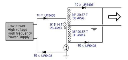
Here, the additional high-voltage diodes allow the two out of phase windings to be connected across each other.
