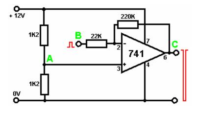
Here, the gain is set by the ratio of the 220K resistor to the 22K resistor. This circuit has a gain of 10 times, so the input signal at point 'B' will generate an output signal at point 'C' which is ten times larger, **provided** that the output signal does not approach the battery voltage. If it does, then clipping will occur with the top and the bottom of the output waveform chopped off at about a volt away from the battery voltage levels, approximately 1 Volt and +11 Volts in this example.
