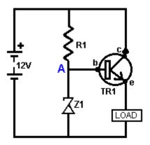
This circuit is supposed to have a fixed voltage at point "A" as the zener diode Z1 is supposed to produce a fixed voltage. That can work reasonably well if the battery voltage is fixed, but if the battery voltage alters either upwards or downwards, the voltage at "A" drifts, which means that the voltage across the load also alters. You will sometimes see this in constant-current circuits.
