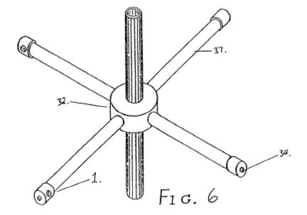
Fig.6 is a top oblique view, partially cut away, of a third embodiment of the rotor of the invention.
