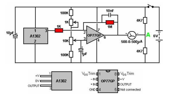
This design uses an OP77GP operational amplifier chip to boost the output signal from the A1302 chip which is a Hall-effect device. The gain of the DC-connected operational amplifier is set by the ratio of the 1K and 1M fixed resistors shown shaded in the circuit diagram, giving a gain of 1,000.
