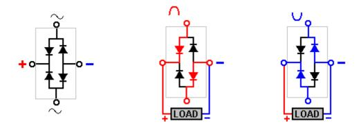
It is possible to connect the bridge in a different way and use it as a higher voltage double diode arrangement as shown here:
