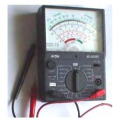
The really excellent non-battery (ex-professional) Avo meter multimeters are still available through eBay at affordable prices. These have 30,000 ohms per volt performance and are robust and accurate, having been built to very high standards.
