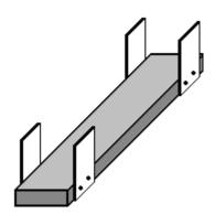
The winding handle part is at the near end and the two 50 gram spools of wire are placed side by side on a rod or dowel at the far end. The longer the plank, the easier it is to draw wire from the supplying spools as the angle between those spools and the spool being wound is smaller. The supplying spools are each just mounted on a dowel pushed through holes in the side pieces. Be sure to make those dowels horizontal so that the spools don't keep moving to one side or the other.
