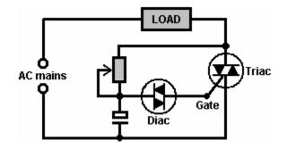
Here, the variable resistor/capacitor pair controls the point on the AC waveform that the Triac is triggered and so controls how much of each sinewave cycle is passed to the mains equipment, and so it controls the average power passed to the equipment. A very common use for a circuit of this type is the 'dimmer-switch' used with household lighting.
