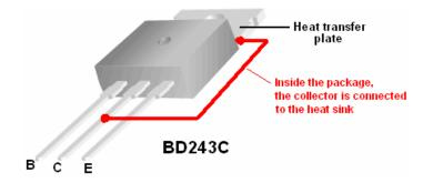
The circuit has been built on the aluminium panels so that the transistors can be bolted directly on to it, and provided with insulating strips mounted on top of it to avoid short circuits to the other components. Standard strip connector blocks have been used to inter-connect the boards which look like this:
