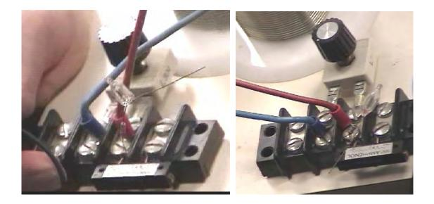
As there are very slight differences in the manufactured coils, each one is tuned to the exact transmitter frequency and a miniature neon is used to show when the tuning has been set correctly.
