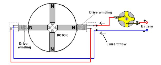
**Step 3:** When the rotor magnet has moved away far enough, the current being fed to the drive electromagnets is cut off. As happens with any coil, when the current is cut off a large reverse voltage spike is generated. That voltage spike is rectified and fed back to the battery.
