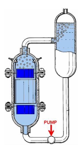
The output pipe of the electrolyser is connected to the side of the electrolyte reservoir and there, the bubbles float upwards and exit through a bubbler while the remaining electrolyte gets circulated again by the pump.
