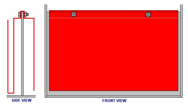
The plate shapes shown above are arranged so that there is access to the bolts from above and they can be reached by a spanner and held steady while the other nut is being tightened.
