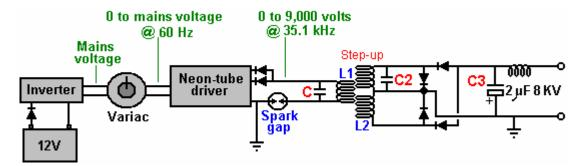
He comments: "the diodes leaving the Neon-tube Driver may need to be reversed as we want to collect the negative polarity. The spark gap will then operate on ambient inversion and the spark will look and sound totally different with a much faster crack and producing very little heat and even becoming covered in frost is possible.
