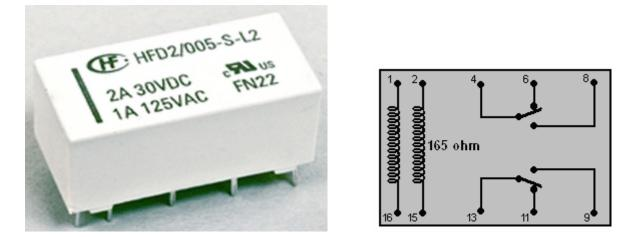
This is the electronic version of a mechanical two-pole switch. A brief pulse of current between pins 1 and 16 locks the switch in one position and later, a pulse of current between pins 2 and 15 locks it in the other position. The current drain on the circuit would be almost zero.
