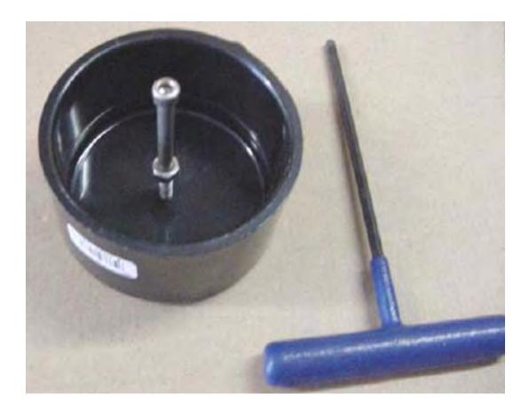
Prepare the bottom cap: Drill and tap 1/4 inch x 20 hole in the centre. Install the capscrew with a stainless steel nut. Tighten and install a washer and stainless steel nut outside.
