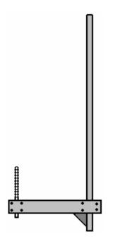
This simple arrangement allows the weight discs to be added and secured in any combination desired. As dumbbells are supplied in pairs, there are four discs of each side which allows a wide range of weight options going up in jumps of just 1 Kg which is very convenient. If the axle shaft has a square cross section, there is no tendency for the lever arm to slide around the shaft
