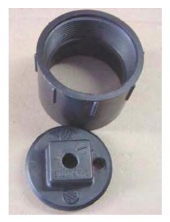
The upper component is a Threaded Adaptor DWV 3 inch HXFPT. The lower component is a 3 inch ABS Plug, clean out the threaded cap. Prepare the top cap and plug: Drill and tap a 3/8 inch diameter NPT in the centre of the threaded cap (this is the main filling plug). Drill and tap a 1/4 inch NPT on the side (to take the barbed fitting).
