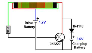
But no matter how long the circuit operated, it would not charge the output battery above 4.0 volts which is 1.33 volts per battery. The load test results were terrible with the voltages at one hourly intervals being 3.93V, 3.89V, 3.84V, 3.82V and 3.79V after only five hours of powering the load. That is ridiculous performance as those batteries managed 22 hours of load powering with the solar panel design.
