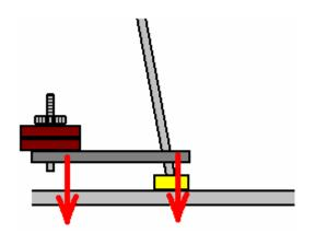
Then there is the sideways forces caused by the rotation of the (unbalanced) weight:
