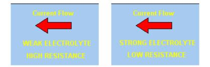
However, there is a problem with using the optimum concentration of electrolyte and that is the current flow caused by the greatly improved electrolyte is likely to be far more than we want. To deal with this we can use an electronic circuit called a "Pulse-Width Modulator" (or "PWM") circuit. These are often sold as "DC Motor-Speed Controllers" and if you buy one, then pick one which can handle 30 amps of current.
