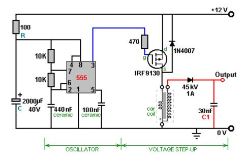
The supply for the 555 timer chip is protected against spikes and dips by the resistor "R" and the capacitor "C". The 555 timer chip acts as an oscillator or "clock" whose speed is governed by the two 10K resistors feeding the 440 nF capacitor. The step-up transformer is an ordinary car coil and the drive power to it is boosted by the IRF9130 FET transistor which is driven by the 555 chip output coming from it's pin 3.
