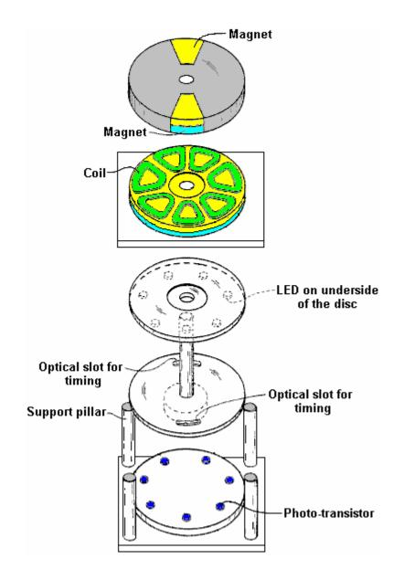
This construction is relatively simple and yet the operation is powerful. The power is provided by three magnets, shown shaded in blue and yellow. The lower magnet is in the form of a disc with the poles arranged on the large, circular, flat faces. This is the stator magnet which does not move. Positioned above it is a disc made of non-magnetic material (shaded in grey) and which has two magnets embedded in it. This disc is the rotor and is attached to the central vertical shaft.
