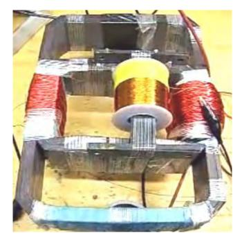
This prototype, as you can see, is fairly simple construction, and yet, given an input power of 106.9 milliwatts, it produces an output power of 403.3 milliwatts, which is 3.77 times greater.
