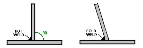
Please don't imagine that you can just push the vertical piece back into position as that isn't going to happen because the joint is instantly very, very strong. Instead, you use two quick welds of equal size, with the second one being 180 degrees opposite the first one:
