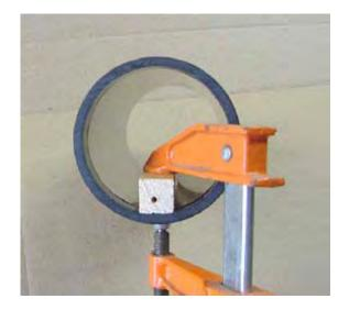
Clamp securely and drill two 0.165 inch holes, one on either side, perpendicular to each other, as best you can. These holes will be tapped 1/4 inch x 20
