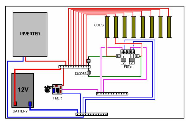
This arrangement keeps soldering to a minimum and allows for easy alterations as the circuit is extended for higher output power. The timer board can be swapped out later on if you decide to use a Divide-by-N style of operation.
