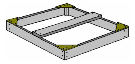
Next, two lengths of the 18 mm thick timbers about 180 mm long are epoxied and screwed to the centre of the 25 mm thick plank, leaving 70 mm clearance to the end of the plank:
