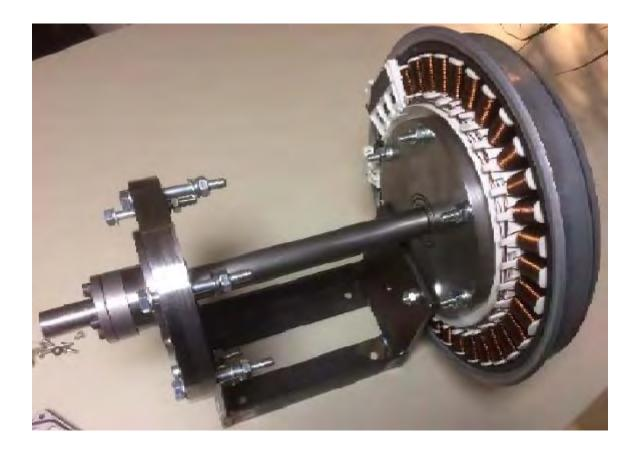
Doing that involves precision metalwork and it will probably be necessary to balance the rotor to avoid vibration when it rotates at high speed, typically 3000 revolutions per minute to drive the alternator. This metalwork can be done by a local metal fabricator business if you do not have the necessary equipment or skill to do this work.
