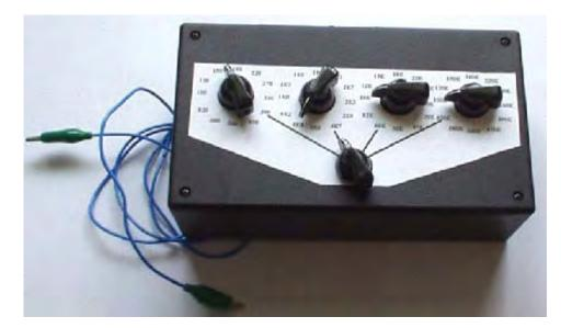
It can also be useful to have a versatile signal generator. You can easily construct your own with variable frequency, variable mark/space ratio and optional variable gating. If you do, you might as well make it with a low output impedance so that it can drive devices under test directly rather than having to provide additional buffering. It might look like this:
