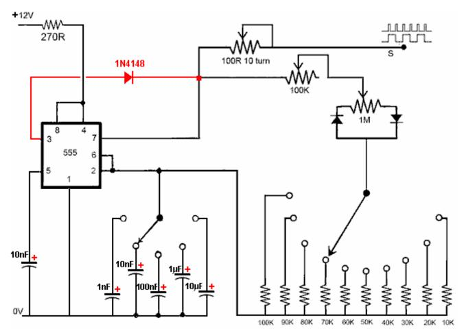
The diode marked in red **must** be a 1N4148 diode. The waveform produced is a clean rectangle no matter what Mark/Space ratio is selected.
