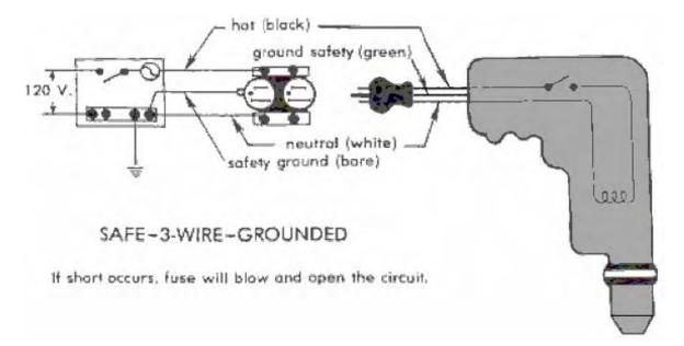
Using grounded receptacles and a safety-ground on all circuits will allow the safety-grounding of appliances when they are plugged into the outlet. An adapter must be used to properly ground appliances connected to receptacles which are not safety-grounded. If an adapter is used, the green pigtail wire must be connected to a known ground to give protection from electrical shock should a short-circuit occur.
