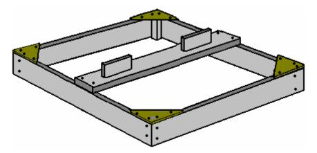
Two timber strips 1350 mm long, are cut and erected vertically, being attached by screws coming upwards through the 25 mm thick plank, and by MDF bracing triangles on one side and across the lower end of the verticals. If a spirit level is used to ensure that the vertical timber is actually vertical, then first, the four corners of the floor frame need to be weighted down to overcome any twisting and the floor frame confirmed to be actually horizontal before attaching the vertical timbers:
