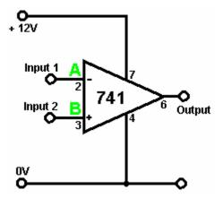
Are you sure you are up to such a difficult circuit? Bit complicated - huh! This is the basic operational form for an operational amplifier.
