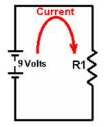
We need to be able to calculate what current is flowing around the circuit. If the circuit contains only resistors, then this can be done using "Ohms Law" which states that "Resistance equals Voltage divided by Current" or, if you prefer:
