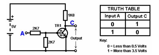
We can see that if the voltage at the input 'A' is taken high, then the output voltage at 'C' will be low. If the voltage at the input 'A' is taken low, then the output voltage at 'C' will be high. A circuit which does this is called an 'Inverter' because it 'inverts' (or 'turns upside down') the input voltage.
