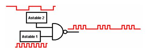
The small circle on the output side of logic devices is to show that they are inverting circuits, in other words, when the input goes up, the output goes down. The two logic devices we have encountered so far have had this circle: the Inverter and the NAND gate.
