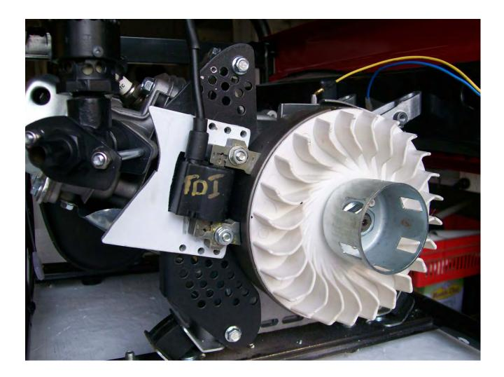
Finally, the covers and the Starter handle need to be bolted back in place.
