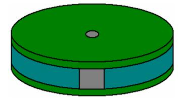
There is a "sweet spot" for the positioning of the power pick-up coils and it will usually be found that this is two or three millimeters away from the rotor. If that is the case, then there will be room for an outer band of duct tape on the rim of the rotor to provide additional protection against the failure of the magnet attachment method.
