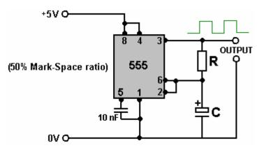
The capacitor used has to be high quality with very low leakage in order to get this waveform which is On for exactly the same length of time as it is Off. This is important if we want the two batteries to receive the same length of time powering the load as the time they receive being recharged.
