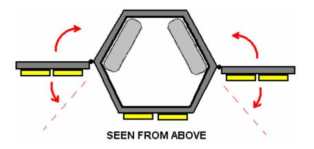
Giving a compact hexagonal shape which is strong and has the same lighting capability and open like this can be hung from the ceiling. The sides extend above the top and below the base so that the unit can stand on a flat surface either way up. The hinges need to be stiff so that they hold their position when set to the desired angle.
