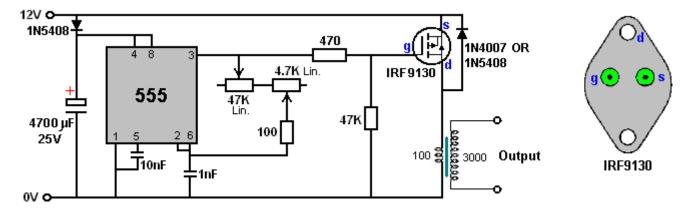
One advantage of this circuit is that the output transformer is driven at the frequency set by the 555 timer and that frequency is not affected by the number of turns in the primary winding, nor it's inductance, wire diameter, or anything else to do with the coil. While this circuit shows the rather expensive IRF9130 transistor, I expect that other P-channel FETs would work satisfactorily in this circuit. The IRF9130 transistor looks like this:
