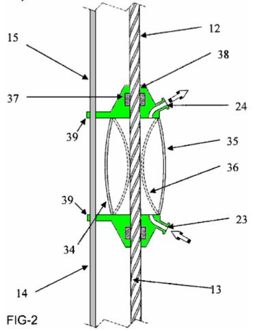
**Fig.2** shows one arrangement for buoy **14** comprising an inflatable capsule **34**. This figure illustrates the shape of the walls of the inflatable capsule **34** when inflated **35** and when deflated **36**. Air passes into capsule **34** through hose **23** and exits from the capsule through hose **24**.
