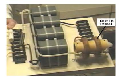
The output current flows through the left hand winding on the brown cylindrical former, and when the photograph was taken, the right-hand winding was no longer in use. Previously, it had been used to provide charging power to the battery by rectifying the electrical power in the coil, caused by the fluctuating magnetic field caused by the pulsing current flowing through the left hand winding, as shown here:
