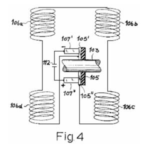
By virtue of the series-connection of coils **106a-106d** between the segments **105'** and **105"**, as illustrated in **Fig.4**, the alternating voltage induced in these coils gives rise to a rectified output voltage at brushes **107'** and **107"**. The unidirectional current delivered by these brushes to a load (not shown) may be smoothed by conventional means, represented by capacitor **112** in **Fig.4**.
