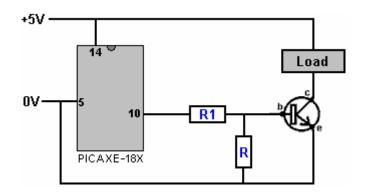
Here, the resistor "R1" limits the current fed into the base of the transistor when pin 10 goes high, but allowing enough current for the transistor to switch on fully, powering the load. The resistor "R" makes sure that the transistor switches off fully when the output on pin 10 goes low. The circuit as shown restricts the load to some piece of equipment which can operate on just five volts, so an alternative circuit could be:
