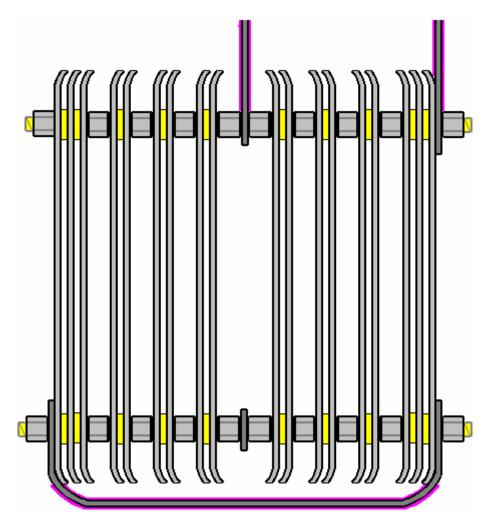
The second modification is wrapping the plate array in 4-inch shrink-wrap. This wrapping extends around the sides of the plates and helps by cutting out some of the unwanted electrical leakage paths through the electrolyte. This arrangement is shown here:
