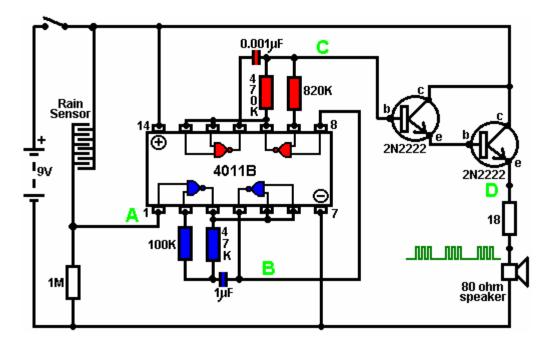
This circuit is comprised of a rain sensor, two astable multivibrators and a power-driver feeding a loudspeaker:
