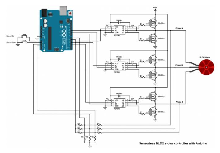
The challenge for this generator design is to modify this circuit so that the Arduino is run on 12 volts while the motor is run on 400 volts. Because the motor has no sensors, the simple-circuit people use back-EMF voltage feeds from the motor to determine its position during rotation:
