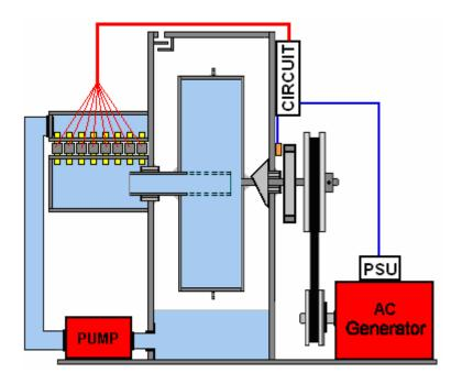
The most direct way of determining the speed of the output shaft is to connect a disc to the shaft and use a sensor to detect how often a magnet in the disc passes by. A rev counter circuit then monitors the shaft speed and switches off valves progressively if the shaft starts to rotate too fast.
