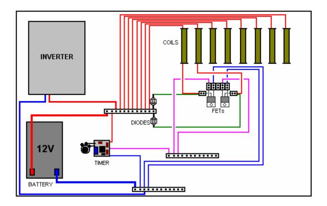
The timer board can be attached to the base board using a screw or a bolt. The board is very light and robust and a single screw is quite sufficient to hold it neatly in place. The variable resistor and the three connecting strips can be glued to the board. Some constructors hate the idea but my preferred method is to use Impact Evostick as the glue as it is very effective and after a day or so becomes very strong indeed.
