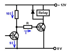
For audio work - microphone pre-amplifiers and the like – the rule of thumb is that the current flowing through the first transistor should be at least ten times the current required by the base of the second transistor in order not to drag down and distort the audio waveform.
