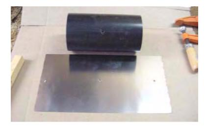
The shimstock holes need to be reamed out to accept the capscrew.
