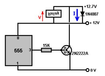
Due to the short-circuiting, the voltage can't get any higher and the current through the diode is not large, so most diodes such as the popular and cheap 1N4001 or 1N4007 types can be used.
