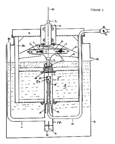
This is a much more complicated device with the rotor bearing having to support the full rotor weight as an axial drag, and there is the addition of an extra air intake, an extra valve, springs and a valve seal among other things.
