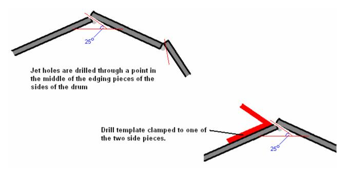
The single drill hole in the middle of the circumference wall of the drum then acts as a jet and using the template to get the drill bit angle the same every time, produces correctly angled water jets.
