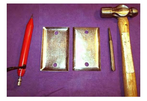
Shown above are typical hand tools used to create the indentations on the plates. The active plate surfaces – that is, the surfaces which are 1.6 mm apart – are indented as well as being sanded.
