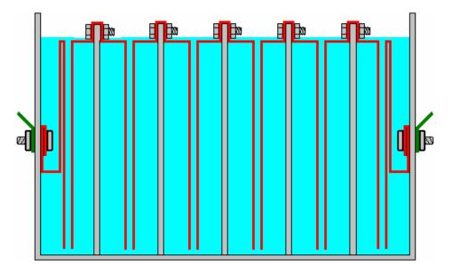
Any of these designs can be 6-cell or 7-cell and the plates can be constructed without outside help. You will notice that the electrical connections at each end of the booster are submerged to make sure that a loose connection can't cause a spark and ignite the HHO gas in the top of the housing. There should be a gasket washer on the inside to prevent any leakage of the electrolyte past the clamping bolt.
