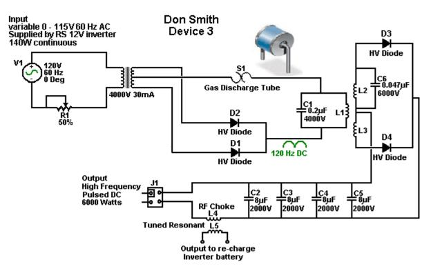
The 4000V 30mA transformer shown in this circuit diagram, may use a ferrite-cored transformer from a neon-tube driver module which steps up the voltage but it does not raise the frequency as that is clearly marked at 120 Hz pulsed DC. You will notice that this circuit diagram is drawn with Plus shown below Minus (which is most unusual).
