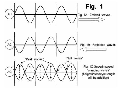
**Fig.1A** indicates an idealized wavelength of an alternating voltage, depicted by a sine wave which is being sent from an AC power supply (shown by a circle at the left end of a horizontal straight wire) into the "input" end of the wire. The voltage waves travel through the wire towards the right, as indicated by
