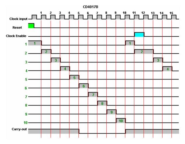
In this example, the sequence is started by the Reset pin being given a high voltage as shown by the green shading. This pushes the output pin 1 to a high voltage and all of the other outputs to a low voltage and holds those voltages as long as the reset voltage is high.
