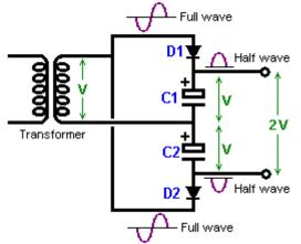
With this circuit, the transformer output is some voltage, say "V" volts of AC current. This output waveform is fed to capacitor "C1" through diode "D1" which lops off the negative part of the cycle. This produces a series of positive half-cycles which charge up capacitor "C1" with a positive voltage of "V".
