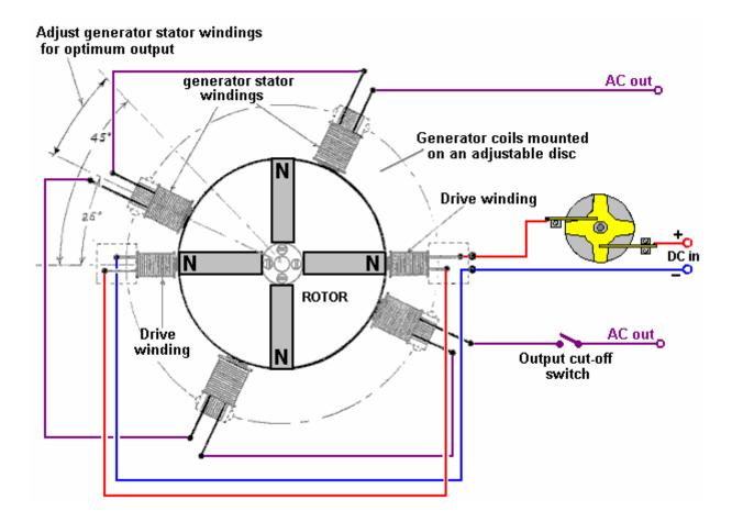
**Step 4:** Surprisingly, the output coils are switched Off for most of the time. This sounds mad but it most definitely isn't mad. With the output coils disconnected, the approaching rotor magnets generate a voltage in the output coil windings but no current can flow. As no current is flowing, no magnetic field is
