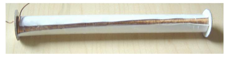
That process is repeated until all of the desired layers have been wound. Finally, the wire is cut with a few inches left for connecting the coil in the circuit, and the wire is passed through a second hole in one of the flanges:
