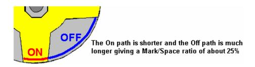
The two brushes can be on the same side of the drive shaft or on opposite sides as shown. One important feature is that the brushes touch in a position where the disc surface is always moving directly away from the brush mounting, causing any drag to be directly along the arm and giving no sideways loading on the brush. The diameter of the device is usually one inch (25 mm) or less.
