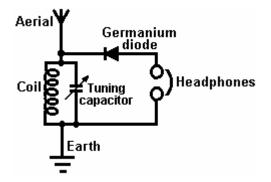
While the circuit diagram above is marked "Tuning capacitor" that is actually quite misleading. Yes, you tune the radio receiver by adjusting the setting of the variable capacitor, **but**, what the capacitor is doing is altering the resonant frequency of the coil/capacitor combination and it is the resonant frequency of that combination which is doing exactly the same job as the variable coil did on it's own.
