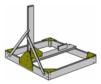
An 18 mm thick timber strip is screwed to the tops of the verticals. This deliberately positions the timber 18 mm off centre as the motor which rotates the top of the axle shaft has to be attached to the middle of this newest timber and that places the motor shaft very close to the central point of the base:
