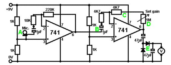
This circuit is two copies of the previous circuit. Each 741 chip has a reference voltage of half the supply voltage created by a voltage-divider pair of 1K resistors. This voltage is fed to pin 3 of the chip, which is the non-inverting input.
