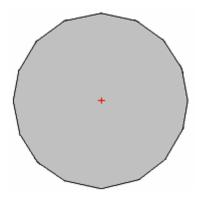
Clamp this side to another piece of 3 mm thick mild steel and mark carefully around it to get the shape and size of the second side of the drum. Cut around this new side and draw some diagonals to establish the centre point.
