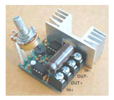
As this unit was rated at just 15 Amps maximum, Zach added another 15 Amp rated FET transistor in parallel to the output stage to raise the current capacity to 30 Amps. A fuse protects against accidental short circuits and a relay is used to control when the electrolyser is to be producing gas. The connecting wire is #12 AWG (swg 14) which has a maximum continuous current capacity of just under
