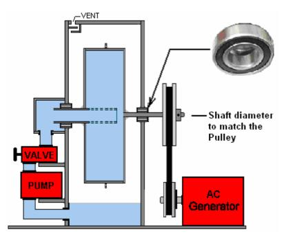
This is a very clever solution with the 3-inch diameter pipe being supported by an ordinary ball or roller bearing. If any liquid were to leak through the bearing, then it ends up in the sump, ready for circulating again.
