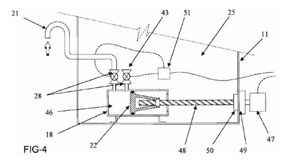
An alternative construction of the first air reservoir **18** is shown in **Fig.4**. In this embodiment, reservoir **18** is housed within a vessel **11** containing a fluid **25**. Air enters reservoir **18** through air intake **21** and is held in a chamber **46**. The reservoir has a piston **22** and the movement of the piston **22** towards the left of the reservoir **18** forces air in the chamber **46** out through air outlet **43**.
