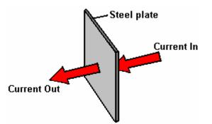
The fact that we have folds and bends in our plates has no significant effect on the current flow. Resistance to current flow through the metal electrode plates is something which can't be overcome easily and economically, and so has to be accepted as an overhead. Generally speaking, the heating from this source is low and not a matter of major concern, but we provide a large amount of plate area to reduce this component of power loss as much as is practical.
