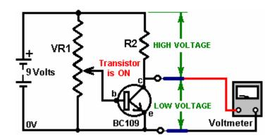
If a bulb is used instead of R2, then it will light when the transistor switches on. If a relay or opto-isolator is used, then a second circuit can be operated:
