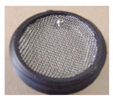
After fitting the mesh tightly into the cap, mount it with a 10/32 inch stainless steel screw on the opposite side to the 1/4 inch tapped hole for the barbed fitting. This is a flame arrestor, so make CERTAIN that the entire inside is covered tightly. Note that the sides wrap up. Turn each layer to cross the grain of the mesh in the successive layers.
