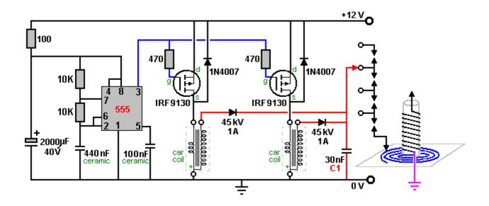
The connection to the pancake coil is by a moveable clamp and the two coils are tuned to resonance by careful and gradual adjustment of that connection, 10 mm at a time (**after** powering down and discharging the "C1" capacitor).
