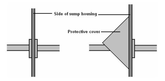
For this, two triangles of steel are cut and then welded so that most of the oil landing on them will run off without reaching the bearing:
