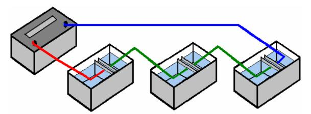
This time we are using three of our 1.24 volt sections and this gives us an electrical efficiency of 30% and three times the amount of gas, making the system nine times more effective.
