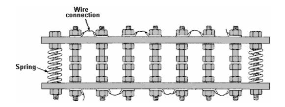
Tightening the bolts which compress the springs moves the bolt heads closer together and reduces all of the spark gaps. The electrical connections can be made to the end tags or to any of the intermediate wire connection straps if fewer spark gaps are required in the chain.
