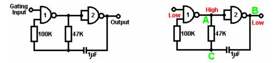
The circuit will not oscillate if the gating input is low, so assume it to be high. Take the moment when the output of gate 2 is low. For this to happen, the inputs of gate 2 have to be high. As the output of gate 1 is wired directly to the inputs of gate 2, it must be high, and for that to be true, at least one of its inputs must be low. This situation is
