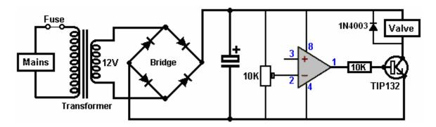
Now the last step is to provide a reference voltage which does not change if the power supply voltage increases. The approved way is to use a zener diode with a resistor in series with it and in theory, the voltage drop across the zener diode is a reliable reference voltage. I have not found that arrangement to work at all well, so I suggest using ordinary diodes such as the 1N5408 instead, like this:
