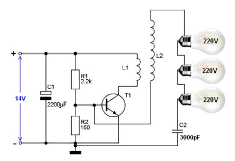
Another possibility would be to take an ordinary cheap halogen heater and re-wire it so that the three 400-watt lamps are in series rather than in parallel:
