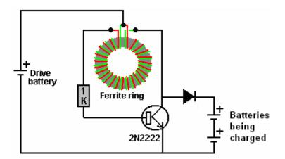
Two NiMh rechargeable batteries have less voltage than a 3-volt LED, so obviously, if the circuit can light a 3V LED it can definitely recharge two NiMh batteries.
