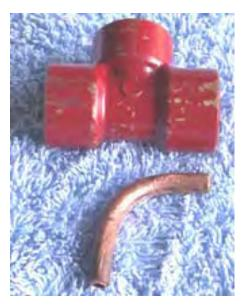
The copper pipe is then heated with a plumber's gas torch and bent very slowly and carefully to the shape shown above. Some people find it helpful to insert a length of suitable flexible material into the pipe before starting the bending – something like the coiled steel spring material used to support net curtains – as that helps to keep the copper pipe from kinking when being bent.
