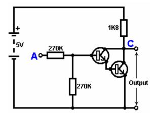
Here, The input impedance has been increased by a factor of 100 by using a Darlington pair of transistors which need far less base current, and so can have a much higher input resistor.
