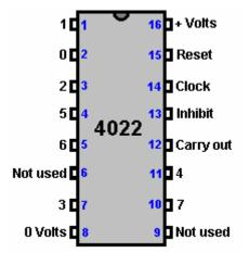
If pin 14 is provided with the output from some variety of astable multivibrator, on the first pulse, this chip sets the "0" output on pin 2 to High while the other outputs are Low. On the next pulse, the "0" output goes Low and the "1" output on pin 1 goes High. On the next pulse, output "1" goes Low and the "2" output on pin 3, goes High. And so on until on the eighth pulse, output "7" on pin 10 goes Low and output "0" goes high again.
