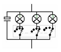
This arrangement gives Off, One panel, Two panels and Three panels of illumination, but it could also be that instead of switching off an entire panel that the switching illuminates one LED array per panel, two LED arrays per panel and three LED arrays per panel.
