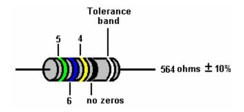
The fourth colour band coding has also been extended to include two other colours:
