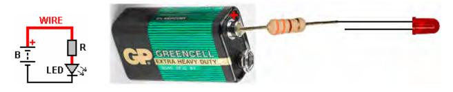
And finally, the other side of the LED is connected to the Minus of the battery:
