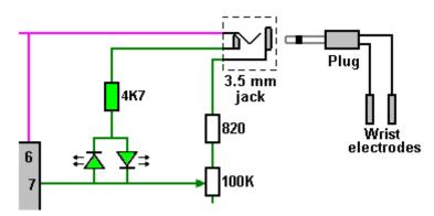
With this arrangement, the two LEDs flash alternately. In any circuit, a capacitor with a higher voltage rating can always be used if the capacitance values are the same. The Beck external circuit is completed through the body of the user, so there is just one electrode connected to each side of the output jack socket. A possible plug-board layout is:
