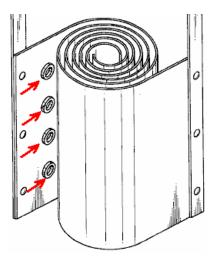
The electrolyser is connected directly to a reservoir of electrolyte and a pump is used to circulate the electrolyte which brushes bubbles off the electrodes:
