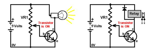
If a buzzer is substituted for R2, then an audible warning will be sounded when the transistor switches on. If a light-dependent resistor is substituted for VR1, then the transistor will switch on when the light level increases or decreases, depending on how the sensor is connected. If a thermistor is used instead of VR1, then the transistor can be switched on by a rise or fall in temperature. The same goes for sound, wind speed, water speed, vibration level, etc. etc. - more of this later.
