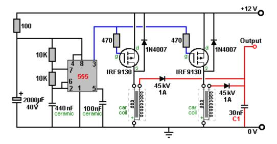
You will notice that the car coil has only three terminals and the terminal marked "+" is the one with the connection common to both of the coils inside the housing. The coil may look like this:
