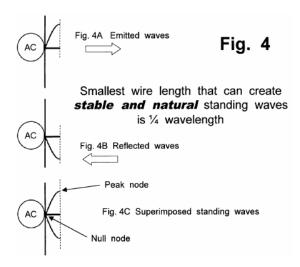
Finally, moving to a still shorter wire, the same principle also applies to any wire which has a length equal to one quarter of an AC voltage wavelength, as shown in **Fig.4A**, **Fig.4B**, and **Fig.4C** Even though it does not stretch across or cover a complete "bubble", the standing wave shown in **Fig.4C** is nevertheless a stable, natural, and resonant "standing wave", with a frequency which is exactly twice the frequency of the input AC voltage.
