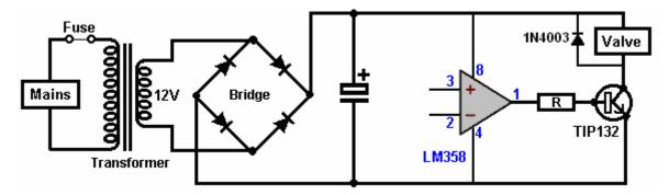
The TIP132 can handle 100 volts, 8 amps and has a gain of 1000, so if it is passing 330 milliamps through the valve winding, then it will need a base current of 0.3 milliamps. That current flows through the resistor "R" which has about 10 volts across it. Resistance = Volts / Amps or 10 / 0.0003 amps which is 33,333 ohms or 33K. However, we will increase the base current by a factor of 3 and use a 10K resistor:
