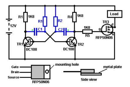
The rate of switching is controlled by the R1/C1 and R2/C2 combinations. The load's ON time to its OFF time is called the 'mark-space' ratio, where the ON period is the 'mark' and the OFF period is the 'space'. If you choose to use electrolytic capacitors which have their own polarity, then the +ve end of each capacitor is connected to the transistor collector.
