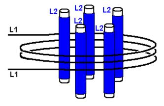
However, there can be an advantage to this arrangement in that the wire length of the L1 coil is greater, which in turn makes the wire length of each L2 coil greater (being four times longer). This gives greater flexibility when planning the turns ratio of the L1/L2 transformer. The voltage step-up or step-down of that transformer happens to be in the ratio of the turns, in spite of the fact that this is not inductive coupling and so standard transformer technology does not apply.
