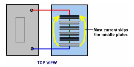
This is a disaster for us as now we will not get your six times the gas production or our massively reduced heating. Thankfully, there is a very simple fix for this problem, and that is to divide the box up into six watertight compartments using thin partitions like this:
