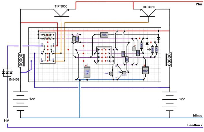
The TIP3055 transistors are there only to raise the current carrying capacity of the tiny latching relay. Let's decide to build a very simple version of the circuit but allowing for later expansion for greater output power. Let's try this circuit arrangement:
