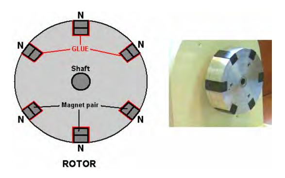
It is not desirable to recess the magnets though it is possible to place a restraining layer around the circumference of the rotor as the clearance between the magnet faces and the coils is about a quarter of an inch (6 mm) when adjusted for optimum performance. The North poles of the magnets face
