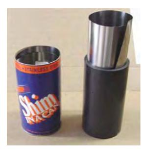
Cut and fit shimstock into ABS tubing, 11 inch works well as this gives a 1 inch overlap.
