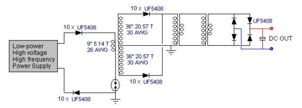
The thick earth wiring is helpful because in order to avoid the earth wire being included in the resonant wire length, you need a sudden change in wire cross-section:
