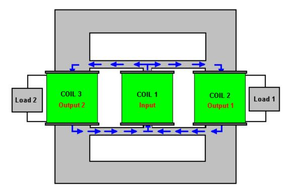
This style of transformer has got quite complicated magnetic flows when it is operating, although the diagram above only shows some of the flow paths generated when the input coil "Coil 1" is pulsed. The really interesting result is seen when that input pulse cuts off and we expect return magnetic flow from coil 2 and coil 3. What happens is this:
