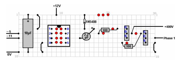
The red circles show where the copper strip on the underside of the board is to be broken. This physical layout has not yet been built and tested, and so is only a suggestion. You can make three separate boards, one for each phase or you can place all three circuits on a single board. Integrated circuits are heat sensitive so I suggest that you use a socket and solder it in place and then plug the chip into the socket when everything is cool. An 8-pin socket looks like this:
