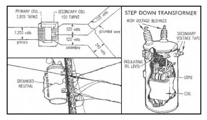
**Single Phase** - The most common type of electrical service or power available to consumers. One transformer is used between the distribution line and the meter. Usually three wires, two "hot" and one neutral, are installed to provide 120V and 240V single-phase service. Single-phase service may also be supplied with a three-phase service.
