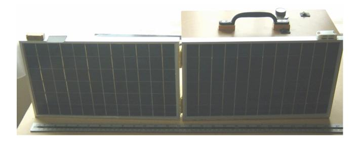
A magnetic catch is used to hold the hinged panel securely closed when the unit is being carried and a small flap is attached beside the magnetic catch to overcome the slightly excessive looseness of the hinges. The unit does not need to be as deep as this experimental model was made.
