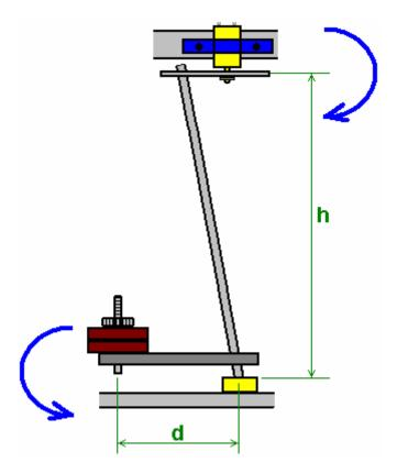
This is the position when at rest. The pull on the motor shaft at the top of the axle shaft is  $W \times d / h$  where W is the weight at the end of arm d. The situation changes immediately the top of the axle shaft is rotated and the weight W starts to swing under the influence of gravity.
