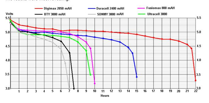
The BTY 3000 batteries do not actually claim on the battery to be 3000 mAHr (although the sellers do) and so, the "3000" could just be a trading name. The tests results for the BTY 3000 were so
