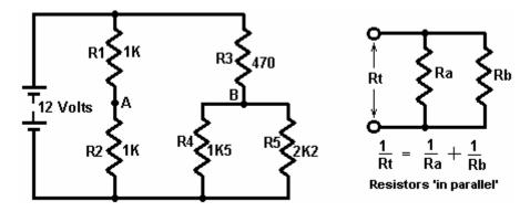
As the current flowing through resistor 'R1' has then to pass through resistor 'R2', they are said to be 'in series' and their resistances are added together when calculating current flows. In the example above, both R1 and R2 are 1K resistors, so together they have a resistance to current flow of 2K (that is, 2,000 ohms).
