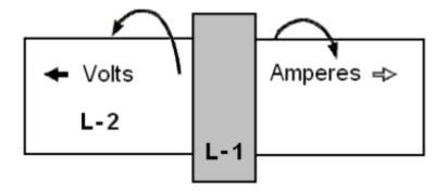
It has been suggested that a greater and more effective power output can be obtained by splitting the L2 coil underneath the L1 coil position, winding the second part of L2 in the opposite direction and
