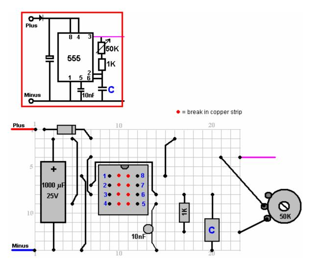
The capacitor "C" will be about 10 nF and the variable resistor can be 47K or 50K linear or a higher value could be used.
