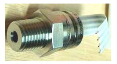
The pressure switch just mounts on one of the end caps of the pressure tank and the switch electrical connection is placed between the relay and the electrolyser. If the gas pressure reaches it's maximum value of 30 psi. then the switch opens, stopping electrolysis until the pressure drops again:
