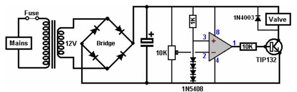
This arrangement gives about 10 milliamps flowing through the diode chain and some 2.75 volts are generated across the diodes. That voltage does not alter appreciably if the power supply voltage increases.
