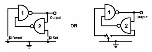
Here, the mechanical switch is buffered by a 'latch'. When the 'Set' switch is operated, the output goes low. The unconnected input of gate '1' acts as if it has a High voltage on it (due to the way the NAND gate circuit was built). The other input is held low by the output of gate '2'. This pushes the output of gate '1' high, which in turn, holds the output of gate '2' low. This is the first stable state.
