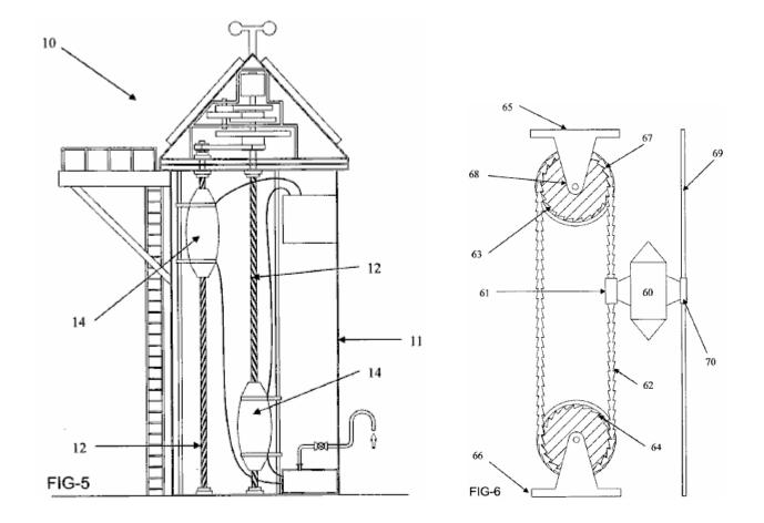
Fig.5 shows an embodiment where which a pair of buoys 14 are present. Each buoy is associated with its own shaft 12 and may move up and down inside vessel 11 independent of one another.
