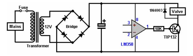
Now we need to get the LM358 to switch off, causing the voltage on pin 1 to drop low, starving the TIP132 of base current and cutting the power to the coil of the valve. For that, we need the voltage on pin 2 to rise above the voltage on pin 3 and we want that to happen if the power supply voltage rises.
