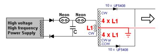
Mind you, there is one other factor to be considered when deciding what the most convenient wire length for L1 might be, and that is the number of turns in the L1 coil. The larger the ratio between the turns in L1 and the turns in L2, the higher the voltage boost produced by the L1/L2 transformer, and remember that the length of L2 is fixed relative to the length of L1.
