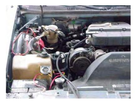
All of the 3/8 inch plastic fittings including one way valves, come from Ryanherco and are made of Kynar to withstand heat. The water trap is from an air compressor. The 3/16 inch tubing or hose is also high-heat type from automatic transmission coolant lines. I use Direct Current and limited with a thermal breaker and LYE mixture adjustment.
