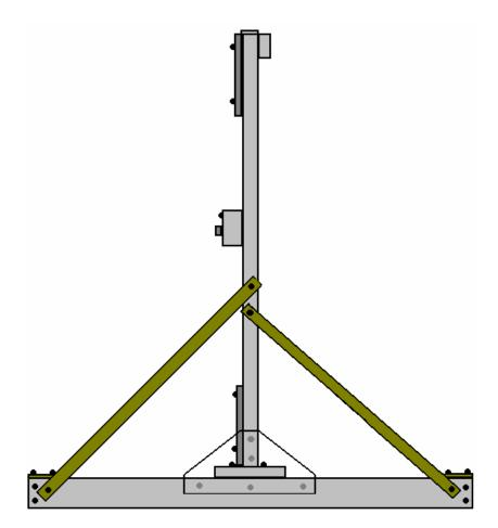
For this style of construction, four pieces of, perhaps, 70 x 18 mm Planed Square Edge timber are cut to perhaps 1050 mm and two 33 x 33 x 65 mm pieces epoxied and screwed to two of the pieces, 18 mm in from the ends:
