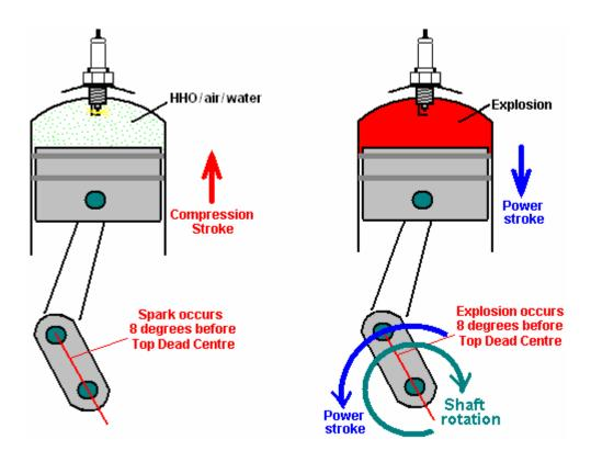
The forces imposed on the piston's connecting rod would be so high that it would be quite liable to break and cause additional engine damage.
