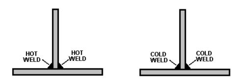
Then, as the welds cool down, they pull in opposing directions and while it produces stresses in the metal, the vertical piece stays vertical. Let the welds cool down in their own good time, taking perhaps ten minutes to cool properly. Do **not** apply water to the welds to speed up the cooling as that actually alters the structure of the steel and you really don't want to do that.
