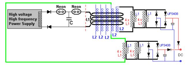
Where two of the L2 coils are shown connected together to give increased output power. This arrangement uses low-voltage inexpensive components for the output stages and there is no obvious limit to the amount of output power which could be provided. As the circuit operates at high frequency throughout, there is no particular need for additional L2 coils to be placed physically inside the L1 coil:
