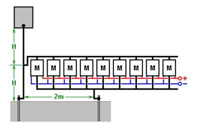
With this arrangement a single module produces around 30 volts while the original method of connecting near the earth was giving about 26 volts with two modules. Jes Ascanius has carried out further experimentation and he states that diodes with response times under 30 milliseconds produce a greater output and he recommends the use of BYV27 diodes which have a 200-volt 25nS rating as he gets three times the output from them. He also recommends using them in Joule Thief circuits.
