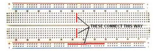
While a plastic board of this type looks as if it should be quick and easy to use, I have never found it to be so ever since the boards were scaled down in size to take the closely-spaced pins of integrated circuits ("chips"). It is generally difficult to lay the components out in the same pattern as the circuit diagram, and if they are not, then it becomes slow to follow the circuit through on the breadboard layout.
