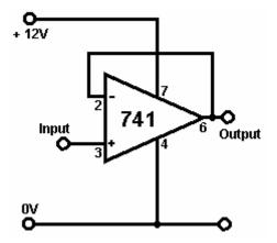
Difficult circuit - huh! Are you sure you can afford all the extra components? This circuit utilises the full gain of the 741 chip. The output follows the input waveform exactly. The input requires almost no current, so the circuit is described as having a 'high input impedance'. The output can drive a serious load such as a relay, so the circuit is described as having a 'low output impedance'.
