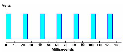
If you wanted "Output 7" (physical pin 13) to do the reverse of this at the same time - that is, when Output 4 goes high we want Output 7 to go low, and vice versa, then, for a 20% Duty Cycle the program would be:
