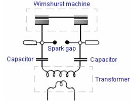
Here, the output of the Wimshurst machine is stored in two high-voltage capacitors (Leyden jars) causing a very high voltage to be created across those capacitors. When the voltage is high enough, a spark jumps across the spark gap, causing a massive surge of current through the primary winding of the transformer, which in his case is a step-down transformer as he is aimed at getting a lower output voltage. Don's circuit is almost identical:
