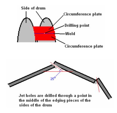
It may be necessary to lower the next circumference plate just opposite the jet exit using a grinding tool so that it does not interfere with the jet of liquid leaving the drum:
