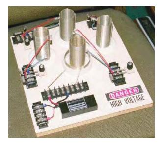
The coil in the centre of the board is a power transmitter made from a Tesla Coil constructed from two Barker & Williamson ready-made coils. Three more of the inner coil are also used as power receivers. The outer, larger diameter coil is a few turns taken from one of their standard coils and organised so that the coil wire length is one quarter of the coil wire length of the inner coil ("L2").
