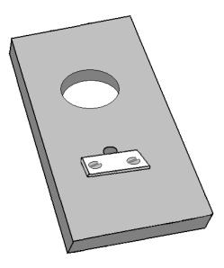
Perhaps cutting a suitable sized hole through a strip of material and using a strip of metal pressed into the flat face of the motor drive shaft (in addition to the hole being a tight push fit) would be adequate for this. A screwed collar or layer of epoxy resin holds the plate firmly to the motor as the plate is positioned below the motor and so gravity tends to pull the plate off the motor shaft at all times.
