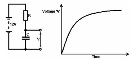
As the voltage increase tails off, it becomes more difficult to measure the difference accurately, so if the capacitor is to be used for generating a time interval, it is normal to use the early part of the graph area where the line is fairly straight and rising fast.
