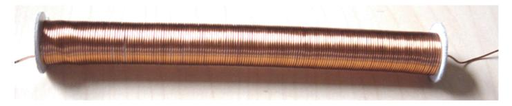
This generator can be built in thousands of variations, the main difference being the coils being used – the core material, the core length, the wire diameter, and the number of layers wound. You can, of course, start with one coil and see how your circuit performs, and later on, add one or more coils to boost the performance.
