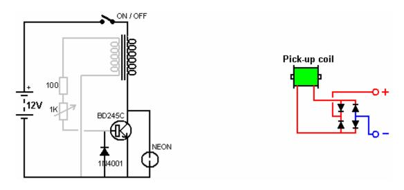
Here are two of the most simple circuits possible, one for drive and one for power collection. The drive circuit transistor is switched on by a voltage generated in the grey coil by a rotor magnet passing by. The transistor then feeds a large current pulse to the black coil, driving the rotor on its way. The neon and the diode are there to protect the transistor and a physical layout for this circuit might be:
