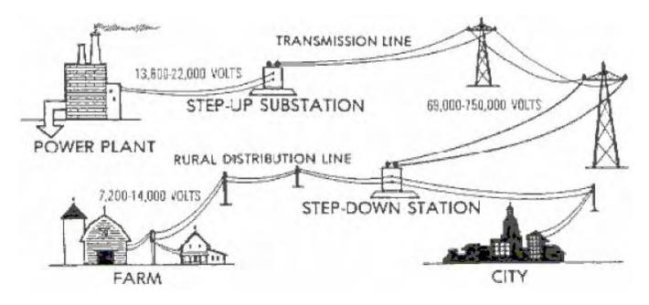
Transformers at the business or residence reduce the voltage to 120 or 240 volts to supply the meter of the customer:
