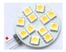
With a diameter of 30 mm and pins which are easy to connect to, these are very convenient devices which have an excellent lighting angle of 160 degrees and a light output of 165 lumens for a 1.2 watt electrical input.
