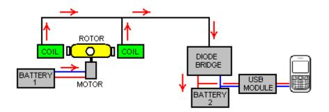
Here, Battery 1 powers the motor which spins the rotor. The powerful rotor magnets passing close by the set of eight coils generates an alternating voltage which is rectified by the diode bridge and used to charge the mobile phone battery through a 5-Volt USB module. Only two of the eight output coils are shown in the diagram above.
