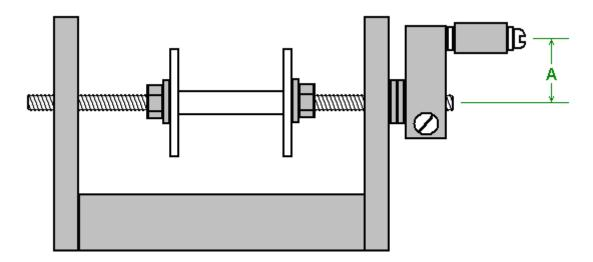
A simple drilled hole in the vertical sides works perfectly well as a bearing, but keep the length "A" short as that needs less wrist movement and with it short, it is quite easy to turn the handle four times per second. A plank around 600 mm long makes a good base for the winder:
