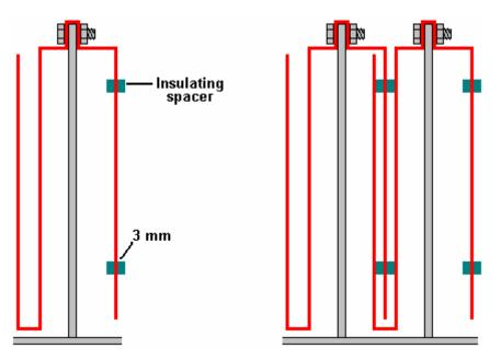
If the current is low enough, an even more simple shape which has just a single pair of active plate surfaces per cell, can be used as shown here:
