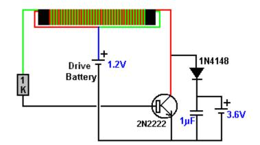
With the battery on charge removed, the voltage on the capacitor reaches 22 volts. Charging the same batteries with this circuit reached 4.14 volts and produced load results of 4.09, 4.05, 4.01, 3.98, 3.96,
