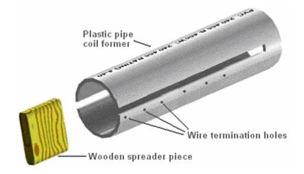
I suggest that the plastic pipe used as the coil former is twice the length of the coil to be wound as that allows a good degree of flexing in the former when the coil is being removed. Before the two slots are cut in the plastic pipe, a wooden spreader piece is cut and it's ends rounded so that it is a push-fit in the pipe. This spreader piece is used to hold the sides of the cut end exactly in position when the wire is being wrapped tightly around the pipe.
