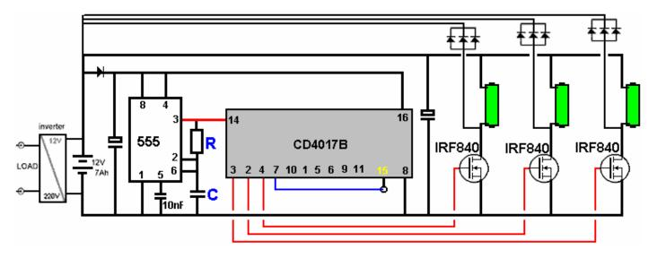
For a divide-by-4 output, pin 10 would be connected to Reset pin 15 and the fourth output would be from pin 7 and the 555 clock pulse rate increased to four times the original rate by lowering the value of "C" or increasing the value of "R".
