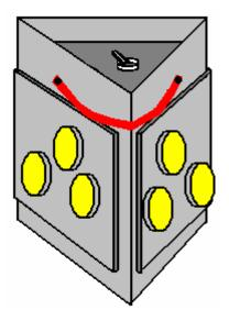
The triangular shape makes for easy construction and is very robust from an engineering point of view. It also cuts down the number of faces needed for 360-degree lighting to just three. The versatility is increased greatly if two faces are hinged:
