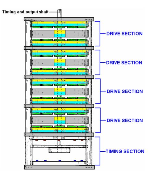
The electrical pulses to the screening coils can be synchronised by the light from Light-Emitting Diodes mounted in the timing section, shining through holes in a timing disc attached to the drive shaft of the motor. The light falling on light-dependant resistors on the other side of the disc, provide the switching for the coil-powering electricity.
