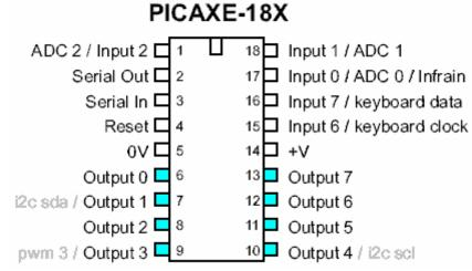
The top eight pins are for making the chip work. The next two are for providing the chip with electrical power. The bottom eight pins are separate outputs, any one of which can operate switches, timers, etc., just as the output from a 555 chip can. Having been named by computer people, instead of the eight output pins being numbered from 1 to 8 as any rational person would do, they have numbered them from 0 to 7.
