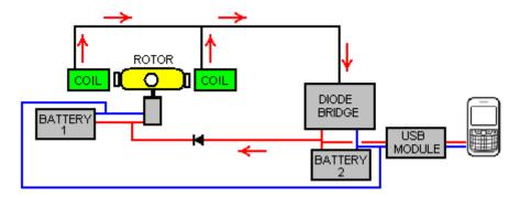
With this arrangement, Battery 2 gets most of the charging current, especially since Battery 1 always has a good level of charge on it and there is a small voltage drop across the diode, so most of the charging current will flow into Battery 2.
