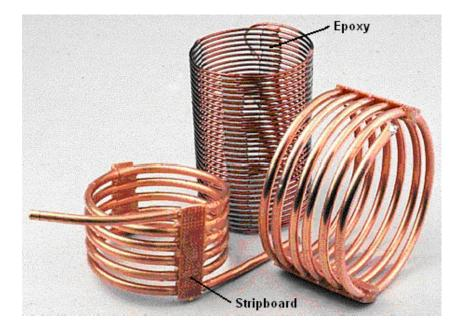
These home-made coils have excellent "Q" Quality factors, some even better than the tinned copper wire coils of Barker & Williamson because the majority of electrical flow is at the surface of the wire and copper is a better conductor of electricity than the silver tinning material.
