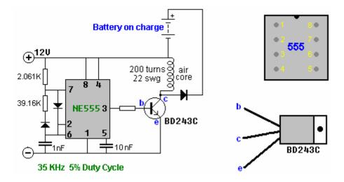
This simple circuit oscillates 35,000 times per second and it is off for 95% of the time. The coil is very simple and is just 200 turns of 0.71 mm diameter enamelled, single core solid copper wire.
