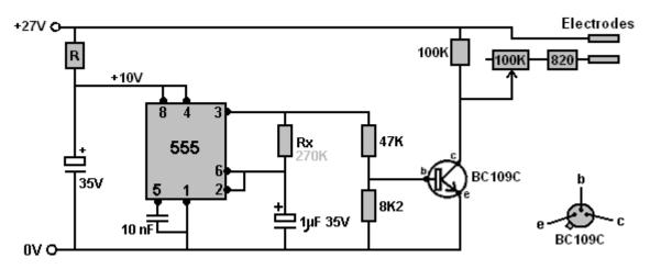
The " $\mathbf{Rx}$ " value is going to be fairly close to 270K so you can use that value when testing to find a suitable value for " $\mathbf{R}$ " (2.2K in my case). The capacitor across the NE555 chip should be as large a capacitance as is convenient, bearing in mind that the entire circuit, batteries, etc. is to fit into a small case to be strapped to a wrist. One way that the components could be positioned on the plug-board is:
