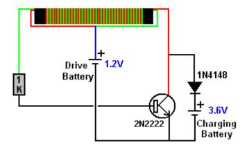
But no matter how long the circuit operated, it would not charge the output battery above 4.0 volts which is 1.33 volts per battery. The load test results were terrible with the voltages at one hourly intervals being 3.93V, 3.89V, 3.84V, 3.82V and 3.79V after only five hours of powering the load. That is ridiculous performance as those batteries managed 22 hours of load powering with the solar panel design.
