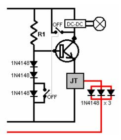
The circuit shown so far has two sets of four batteries. It would be nice to swap them over every few minutes. Batteries which are powering a load don't charge nearly as well as disconnected batteries which are being charged. However, the mechanism which switches between the two sets of batteries needs to have extremely low current draw in order not to waste current. One possibility for that would be to use a 5-volt latching relay like this one:
