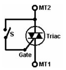
There are three connections to the device: Main Terminal 1, Main Terminal 2 and the Gate. When switch 'S' shown in the diagram is closed, the triac conducts on both positive and negative voltages applied to its MT1 and MT2 terminals. When the switch is open, the device does not conduct at all.
