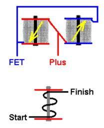
The two sets of five coils in series are connected in opposite directions as shown above. The Start of the set of coils shown in blue and the Finish of the set of coils shown in red are connected to the Plus of the battery. This causes current to flow in opposite directions in each set of five coils and if one set has a North pole facing the rotor, then the other set will have a South pole facing the rotor. The coils are alternated around the rotor like this:
