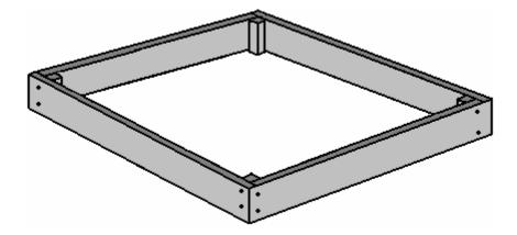
Then corner bracing triangles of MDF are screwed in place:
