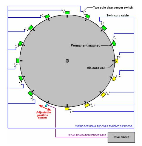
With this arrangement, if the positions the switches as shown for ten of the fifteen coils shown here, then they act as drive coils. The sensor is adjusted so that the drive circuit delivers a brief energising pulse to those coils just after the magnets have passed their exact alignment position with the coils. This causes them to generate a magnetic field which repels the magnets, thrusting the rotor around.
