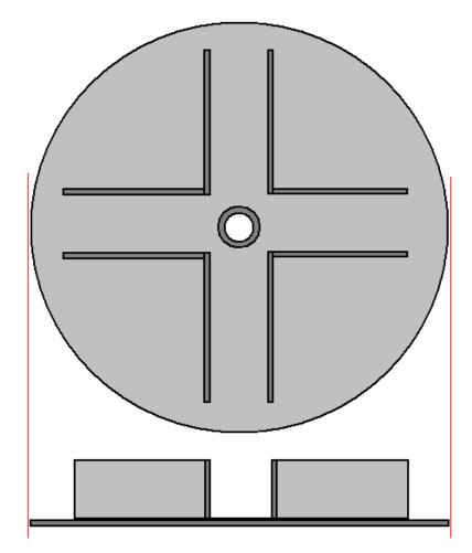
These strips are to channel the water (or other fluid such as transmission fluid) as it passes through the drum when the generator is operating. There must be at least 50 mm (two inches) clear between these plates and the edge of the disc to allow easy flow of water past the plates.
