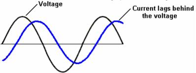
At first, this does not look like any great problem, but it has a very significant effect on the actual power in watts. To get the 37.5 watts output which we were talking about earlier, we multiplied the average voltage level by the average current level. But these two values do not occur at the same time and that has a major effect.
