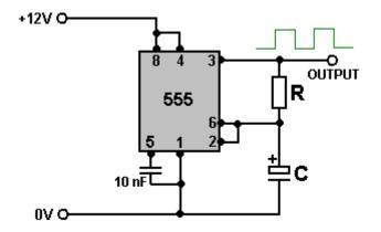
This leaves us with choosing a value for the capacitor and the resistor. We need to pay attention to the fact that the circuit will be running on 27 volts and while the capacitor will not charge up to anything like that voltage, we still will pick one which will survive 27V. Looking on the local eBay shows that a pack of ten capacitors of 1 microfarad rated at 50V can be bought for just £1 including postage, so take that as the value for "C". Looking at the 555 table of frequencies above shows:
