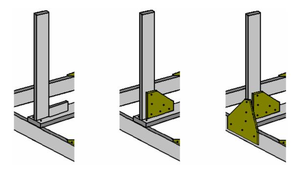
Each vertical needs to be braced on both sides with diagonal strip, either metal or timber:
