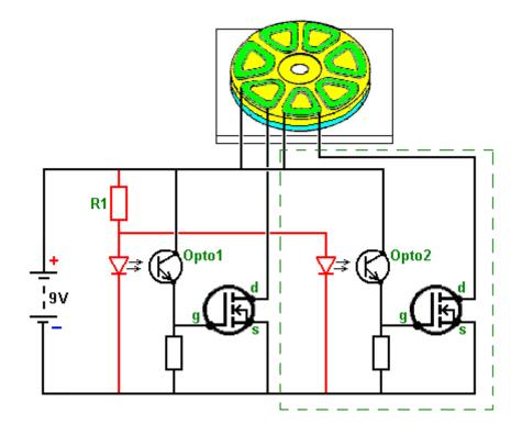
The section inside the green dashed line being the identical circuit for the second coil. This addition to the circuit is made for each coil, at which point, the motor is ready to run. If, as would be normal, several layers of magnets are being used, then the coils positioned above each other can be connected in a chain like this:
