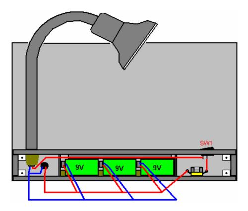
Here, the weight of the solar panel and the three battery packs give the unit stability if the lamp is bent in any direction. With four LED arrays, an excellent level of lighting results, however, I would suggest using five LED arrays as that gives an even wider range of lighting.
