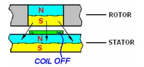
When the coil does not have current flowing through it, it does not produce a magnetic field and the South pole of the rotor magnet is attracted equally forwards and backwards by the North pole of the stator magnet. If there are two coils as shown below, and one is powered and the other is not powered, the backward pull is cancelled out and the forward pull causes the rotor to move forwards:
