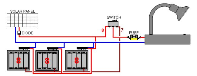
With this arrangement, the lighting unit is fed by either eight batteries or by seven batteries, depending on the position of the change-over switch. When the solar panel is charging the batteries, all eight batteries per holder get charged no matter what position the extra switch is in.
