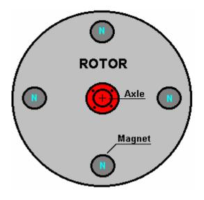
It needs to be remembered that the proportions of the magnets are for the magnet length to be more than the diameter, so in cases like this where circular magnet faces are to be used, the magnets will be cylindrical and the rotor needs to have a significant thickness, which will depend on the magnets which are available locally. The magnets should be a tight push-fit in their holes and securely glued in place.
