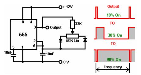
The output waveform changes drastically as the variable resistor is adjusted, but the frequency (or pitch of the note) of the output is supposed to stay unaltered. However, many builders report that this circuit does not do what it is supposed to do and that adjusting the Mark/Space ratio does indeed alter the frequency.
