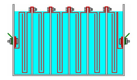
While this six-cell design may look a little complicated to a quick glance, it is really a very simple construction. Each of the plates used in the central cells is just this shape:
