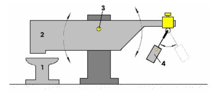
Here, the beam **2** is very much heavier than the pendulum weight **4**. But, when the pendulum is set swinging by a slight push, the beam **2** pounds down on anvil **1** with considerable force, certainly much greater force than was needed to make the pendulum swing.
