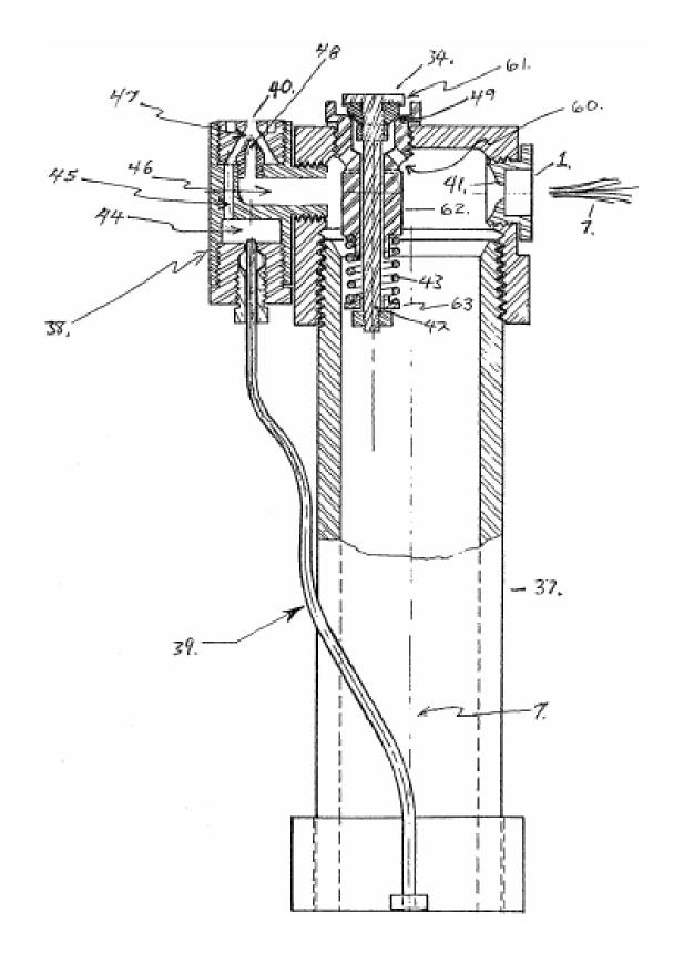
Fig.7 is a top elevation view, partially cut away, of greater detail of the outer end of a radial feed arm of the third embodiment of the rotor of the invention, showing a centrifugal-force operated, poppet type governor release valve, a pressure operated jet-siphon air purging mechanism and a correctly shaped thrust-jet.
