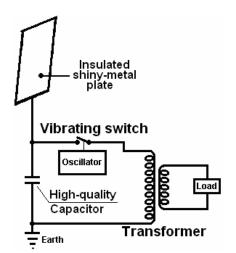
Instead of using an aerial, it is possible to use a **Tesla Coil** which produces very high currents **if** the primary winding is placed in the middle of the secondary winding and not at one end which is the usual configuration. With one method, Tesla directs the output on to a single metal plate and powers a load between the plate and the earth.
