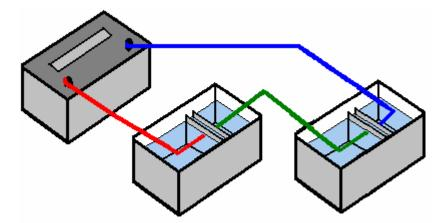
This arrangement uses our 1.24 volts twice while the twelve volts stays unchanged and so the electrical efficiency goes up to 20% and the heat loss drops to 80%. That is quite an improvement but even more important is the fact that twice as much HHO gas is now produced, so we have doubled the electrical efficiency **and** doubled the gas output, giving a result which is four times better than before.
