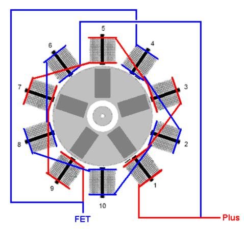
All ten coils are pulsed at the same instant and that instant is arranged to happen when a rotor magnet is between the two opposing coils. One coil pushes the magnet away and the other coil pulls that same magnet towards itself. This is very effective with the rotor spinning so fast that the developer describes it as being "scary" and he has to clamp it to the workbench because of the power being generated.
