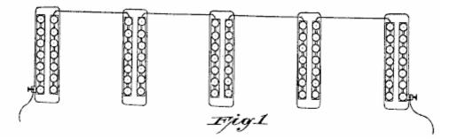
Fig.1 shows five elements connected in a chain. This view is from above with the rectangles indicating holes in the ground where each hole contains seven separate pairs of electrodes.
