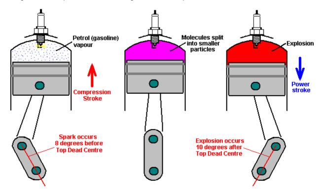
If you were to replace the petrol vapour with HHO gas, then there would be a major problem. This is because HHO gas has very small molecule sizes which do not need any kind of breaking down and which burn instantly. The result would be an explosion which occurs far too soon and which opposes the movement of the rising piston as shown here:
