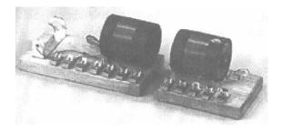
Used to demonstrate electromagnetic radiation between two UC circuits - one a transmitter and the other a receiver. When the 1.5 volt power transmitter is pulsed, the radiated signal is picked up by the remote receiver circuit which then lights up a 70 volt neon lamp.
