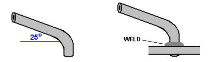
How many jets? I would suggest sixteen, but the number is not critical. It is said that the jets of water are more effective if they strike a nearby surface, so we may choose to attach a series of baffle plates to the outer housing. How many baffle plates? I would suggest sixteen. BUT these baffle plates are only effective when starting a stationary rotor and so can be omitted if you prefer.
