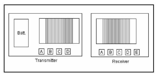
Diagram of transmitter and receiver coils
