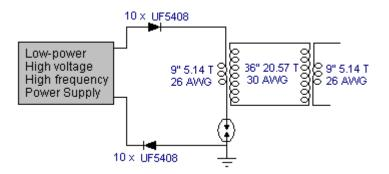
Here, an identical transformer, wound in exactly the same way, is used in reverse, to start the voltage lowering sequence. The wire length ratio is maintained to keep the transformer windings resonant with each other.
