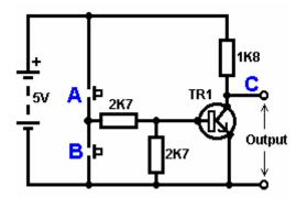
If neither of the press-button switches are operated, the transistor has no base/emitter current flow and so it is off. This places the collector voltage at ' $\mathbf{C}$ ' near the positive rail (+5 Volts).
