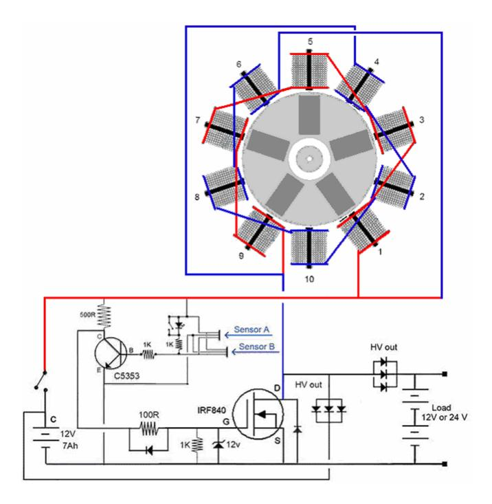
If we want to reproduce this performance without the rotor and it's magnets, then we need to apply 12-volt pulses to those two chains of coils 417 times every second. That may sound difficult if you are not familiar with electronics, but in actual fact, it is a very simple task and 417 Hz is very slow operation for an electronic circuit as they could easily generate 3,000,000 pulses per second.
