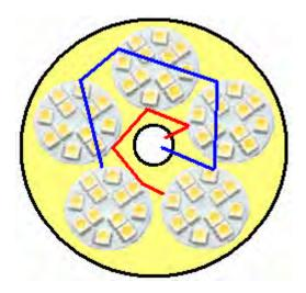
This disc is then eased through the mouth of the lamp shade where it sits about 10 mm below the rim of the shade due to the taper of the shade. Position the disc so that it is square on to the rim of the shade
