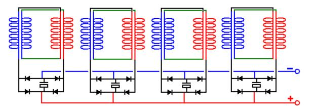
Here, each pair of coils has its own rectification and smoothing capacitor and as such, each pair acts as a small everlasting battery. An alternative to that is to use a voltage-doubler circuit for the rectification to nearly double the output voltage when powering a load:
