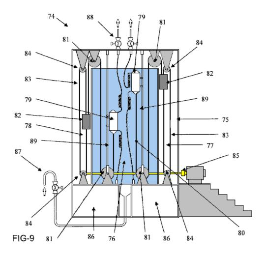
Fig.9 shows an alternative embodiment of this energy generation system 74. The system is comprised of a vessel 75 having a fluid-filled "wet" compartment 76 and one or more "dry" compartments (in this case, a pair of dry compartments 77, 78) with no liquid in them. These dry compartments may be fabricated from any suitable material, such as, concrete, steel, fibreglass, plastic or any combination of materials.
