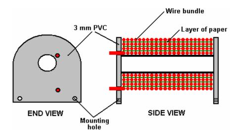
The coils are wound with the end plates attached and drilled ready to screw to their 1/4 inch (6 mm) PVC bases, which are the bolted to the 3/4 inch (18 mm) MDF supporting structure. To help the winding to remain completely even, a piece of paper is placed over each layer of the winding:
