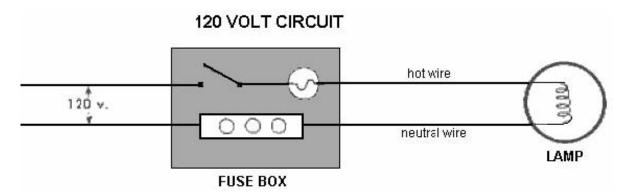
The voltage in a 120V circuit is measured with a voltmeter with one lead on the hot terminal and the other lead on the neutral bar. The number of amperes flowing may be measured with a clamp-on ammeter by encircling the hot or neutral wire with the jaws of the ammeter.
