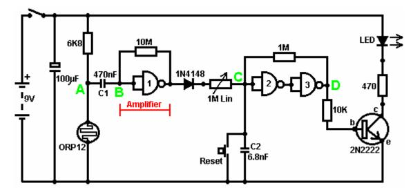
This circuit operates when there is a sudden change in light level. The previous light-level switching circuit was designed to trigger at some particular level of increasing or decreasing level of lighting. This is a shadow-detecting circuit which could be used to detect somebody walking past a light in a corridor or some similar situation.
