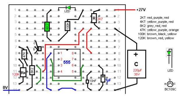
Remember that when trying various resistors for "**R**" you need to start high at about 4.7K and the resulting voltage on the capacitor shows the voltage drop across your first resistor choice and so, the actual current being drawn by your particular NE555 chip. That calculated current will allow you to calculate the resistor value needed to give 10 volts or so, allowing your next resistor to be tested to be almost exact in value.
