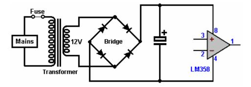
If the voltage at pin 3 exceeds the voltage at pin 2 then the output on pin 1 will be high (about 10 volts) otherwise the voltage on pin 1 will be low. We will us the high voltage on pin 1 to switch on one of the valves and we will use a high-power high-gain transistor like the TIP132 to do this:
