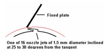
Howver, the later patent points out that while the jets always apply their thrust to the rotor drum no matter what speed it is rotating at, once the drum gets up to speed, the fluid coming out of the jets is nearly stationary relative to the sump and so these baffle plates would only be helpful when starting from stationary.
