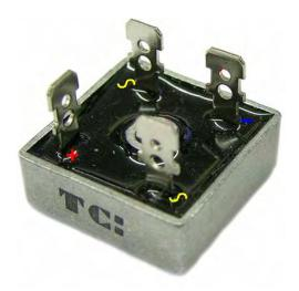
The alternating signal is connected between two opposite corners and the pulsating DC is taken off from the other two terminals. The symbols shown above are normally marked on the flat face which is not seen in this picture. The package has a hole in the centre so that the metal case can be bolted to a heat-sink in order to keep the device reasonably cool when carrying large currents. The connections inside the package are like this:
