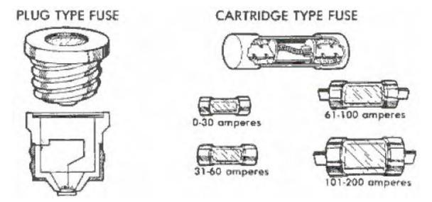
**Fusetrons** (time-delay fuses) are made to carry a temporary overload, such as the overload caused by the starting of an electric motor. The fuse, however, still provides protection for the circuit, and a short-circuit will melt the fuse link. If a common fuse is used, the fuse link will melt every time an electric motor starts. The use of a larger ampere common fuse will prevent the "blow" resulting from the temporary overload, but will not provide protection for the motor or the circuit.
