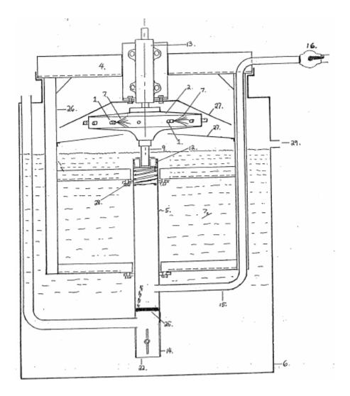
Fig.3 is a front elevation view, partially in cross-section, of a second embodiment of the apparatus showing the one-way valve in the open position.
