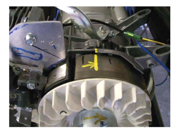
5. Next comes a bit of arithmetic. The diameter of the flywheel is 180 mm which means that it's circumference is  $3.14159 \times 180 = 565.5$  mm and as there are 360 degrees in each rotation of the flywheel, then the outside edge of the flywheel will move 1.57 mm for each of those degrees.
