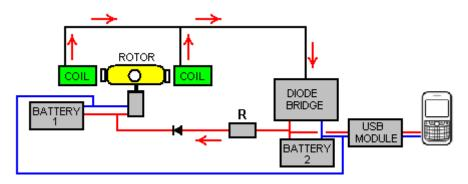
The value of the resistor "R" has to be found by experimentation with your own physical implementation, but I would expect the value to be low, perhaps 47 ohms or so. If the light is not required, then all eight output coils can be used for charging. The coils are connected in pairs and Denis has an unusual method of connecting them:
