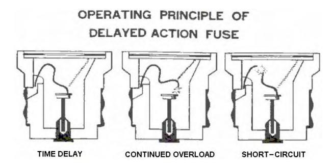
**Fustats**, non-tamperable fuses of the time-delay type, have a different size base and require a special adapter which is screwed into the standard fuse socket. After the adapter is installed, it cannot be removed. For example, the installation of a 15-ampere adapter allows only the use of 15-ampere or smaller fuse.
