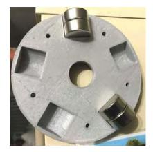
This 3D-printed rotor is made in two halves which are then bolted together.
