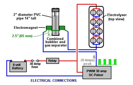
Many years of experimentation and testing have shown that 316L-grade stainless steel is the most suitable material for electrodes, but surprisingly, stainless steel is not highly electrically conductive as you would expect. Each electrode causes a voltage drop of nearly half a volt, and so careful surface
