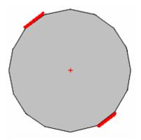
The welds can be made inside the drum if you wish. Two more circumference pieces are then measured carefully, cut and welded like this:
