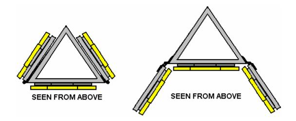
This arrangement allows two faces to be aligned with the fixed front face, giving all horizontal lighting in one direction which is a very, very bright arrangement. The two faces can be moved further around to give the wanted narrow forward beam for walking outdoors. If desired, the lighting level can be controlled by making the On/Off switch a three-pole four-way rotary switch:
