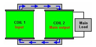
When a pulse of input power is delivered to Coil 1 (called the "Primary winding"), it creates a magnetic wave which passes around the frame or "yoke" of the transformer, passing though Coil 2 (called the "Secondary winding") and back to Coil 1 again as shown by the blue arrows. This magnetic pulse
