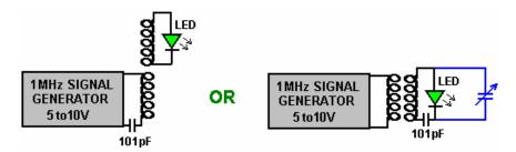
Before you buy the kit, it is not mentioned that in order to use it, you now need a signal generator capable of producing a 10-volt signal at 1 MHz. The coil has a DC resistance of just 1.9 ohms but at a 1 MHz resonant frequency, the necessary drive power is quite low.
