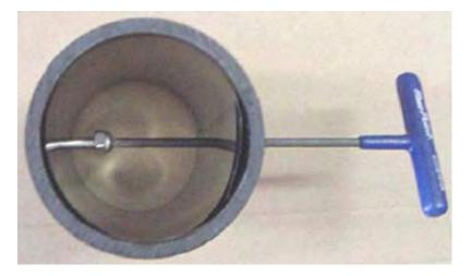
Note: This is why 2 holes are drilled (to facilitate assembly). Next, attach the electrode inside the barrel. It is **important** to us a stainless steel nut inside to seat the capscrew.
