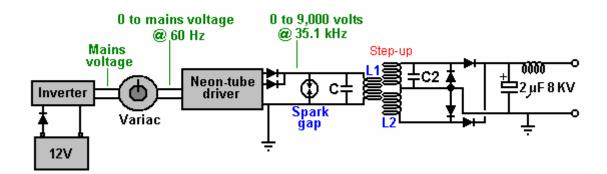
This arrangement has bothered some readers recently as they feel that the spark gap should be in series with the L1 coil, like this:
