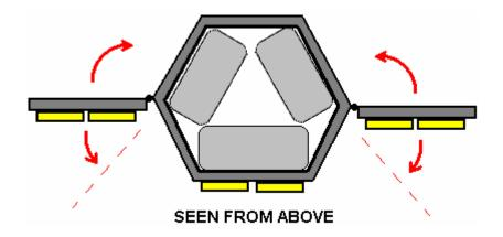
Giving a compact hexagonal shape which is strong and has the same lighting capability. The sides extend above the top and below the base so that the unit can stand on a flat surface either way up. The hinges need to be stiff so that they hold their position when set to the desired angle.
