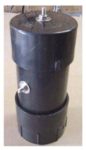
This is the finished cell shown here upside down. Assemble the unit using ABS glue.
