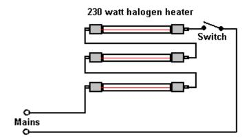
This arrangement 'under-runs' the lamps as each lamp only gets one third of the voltage which it was designed for. If the halogen heater is now connected across 700 volts and the three lamps are similar to each other, then about one third of the 700 volts will be across each bulb. This is only an untested 700 volt suggestion although a heater of this type works well at low power on 220 volts. However, should give a high voltage resistive load as a starting point for experimentation.
