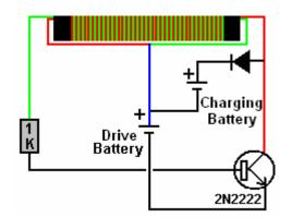
A suitable coil can be wound quite easily. A pencil makes a good former for a coil, so a 100 mm or 150 mm wide strip of paper can be wrapped around a pencil to form a cylinder several layers thick and sealed with Selotape:
