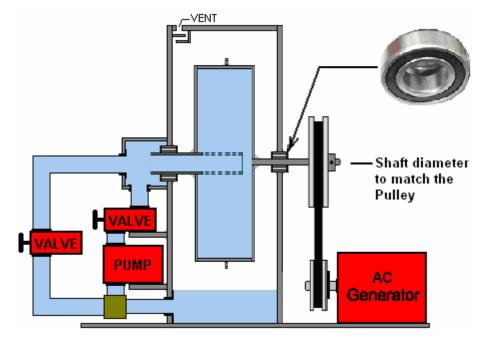
While this does require some additional piping, a valve and a T-junction for the pipe bypass, it results in a pump which can be switched off when not needed and the new valve used as the drum speed control.
