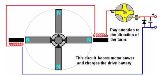
Here, two electromagnets are driven by the battery via Robert's 4-arm commutator which is mounted on the rotor shaft. Some of the recommendations given by Robert are the opposite of what you would expect. For example, he says that a single rotor construction tends to be more electrically efficient than one where several rotors are mounted on a single shaft. Robert is against the use of reed switches and he recommends making one of his commutators.
