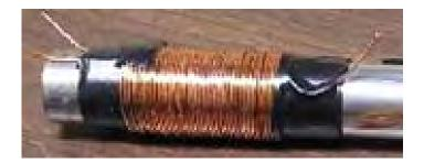
The wire for the third layer is cut to a length of 313 centimeters. Since it will be covering less length along the former, there is no need to build up the ends of the earlier layers. So, simply cover the second winding with tape, and then wind on the third layer, but this time, the coil is wound in a counter-clockwise direction and then the entire coil is covered in tape to protect it.
