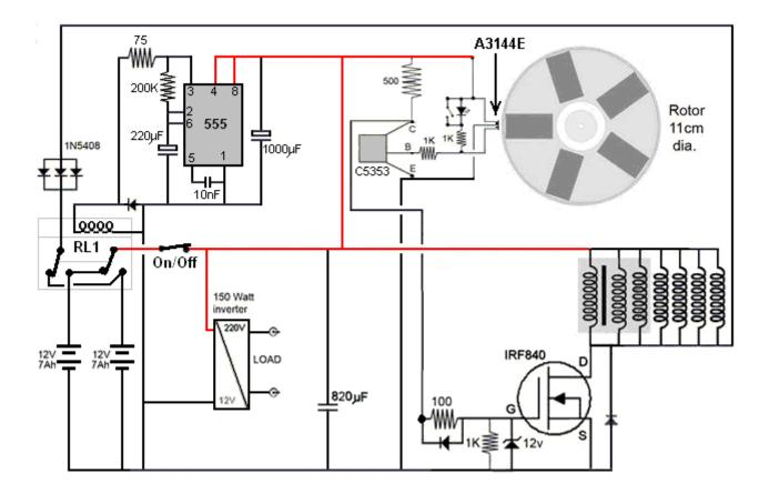
In this version of the circuit, a 12-volt non-latching relay is used. The relay normally draws 100 milliamps at 12 volts but a 75 ohm or a 100 ohm resistor in series lowers that current to about 60 milliamps. That current is only drawn for half the time as the relay is not powered up when the "normally closed" contacts are being used. The system powers itself very satisfactorily as before.
