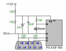
A standard 9-pin computer socket has it's pin 2 connected to the PIC's pin 2, pin 3 connected to the PIC's pin 3 via a 10K / 22K voltage divider resistor pair (which lowers the incoming signal voltage), and pin 5 is connected to the PIC's pin 5. That is all that's needed to feed information into the PIC chip.
