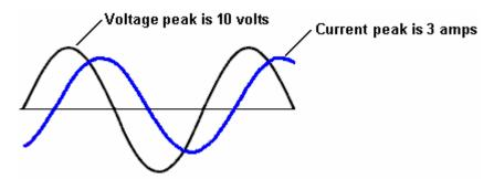
When the voltage is peaking, the current is nowhere near it's peak value of 3 amps:
