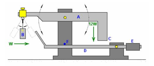
Here, the main beam **A**, is exactly balanced when weight **B** is hanging motionless in it's "at-rest" position. When weight **B** is set swinging, it causes beam **A** to oscillate, providing much greater power at point **C** due to the much greater mass of beam **A**. If an additional, lightweight beam **D** is provided and counterbalanced by weight **E**, so that it has a very light upward pressure on its movement stop **F**, then the operation should be self-sustaining.
