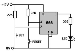
All right, suppose that we want to design and build a circuit to do the same as Bob Beck's pulser circuit mentioned in chapter 11. The requirements are to produce a square wave output pulsing four times per second using a 27 volt power supply, the circuit being powered by three small PP3 size batteries. An obvious choice for the circuit seems to be a 555 timer chip which is small, robust and cheap and a suitable circuit would appear to be:
