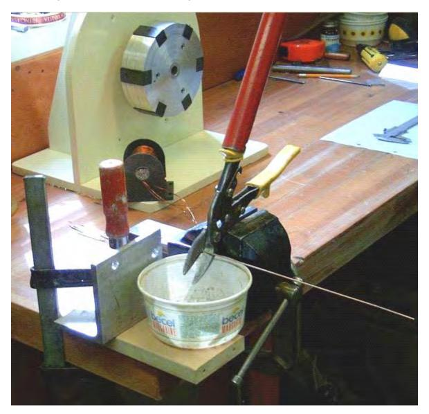
The distance between the shears and the metal angle clamped to the workbench makes each cut length of wire exactly the required size while the plastic container collects the cut pieces ready for coating with clear shellac or clear polyurethane varnish before use in the coil cores.
