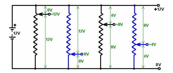
This determination of the voltage levels is the key factor to understanding electronic circuitry. The voltage levels control what currents flow and how every circuit will perform, so it is essential to understand what is happening. Stick with this section until you understand it, and if necessary, ask questions about what you find difficult.
