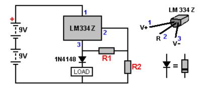
Here, the resistor **R1** controls how much current will flow in the circuit and the resistor **R2** needs to be ten times higher in value than **R1**. One snag is that the LM334Z drops about 4-volts when stabilising the current through the load. That is a lot of voltage sacrificed. An alternative arrangement is:
