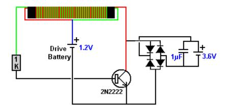
Without the charging battery connected, this circuit gives 28 volts on the capacitor and the battery charging is good, giving load testing results of 4.18, 4.16, 4.15, 4.13, 4.11, 4.10, 4.08, 4.08, 4.06, 4.05, 4.04, 4.03, 4.02, 4.00, 3.99, 3.98, 3.97, 3.96, 3.95, 3.95, 3.94, 3.94, 3.93, 3.93, and 3.93 volts after powering the load for 24 hours. This seems to be a very satisfactory result for such a minor alteration.
