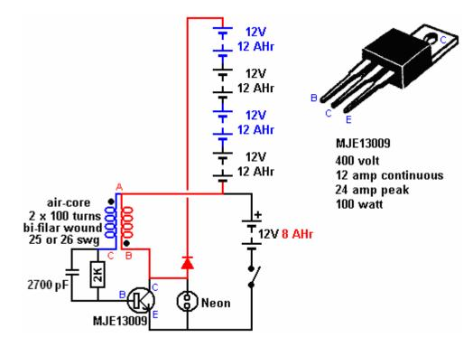
The coil is wound on a hollow former, using two separate strands of wire of 0.5 mm diameter, giving a resistance of just 2 ohms. The strands of wire are placed side by side in a single layer like this:
