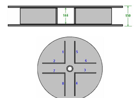
Use the magnetic clamps to hold each plate vertical when positioning and tack welding it:
