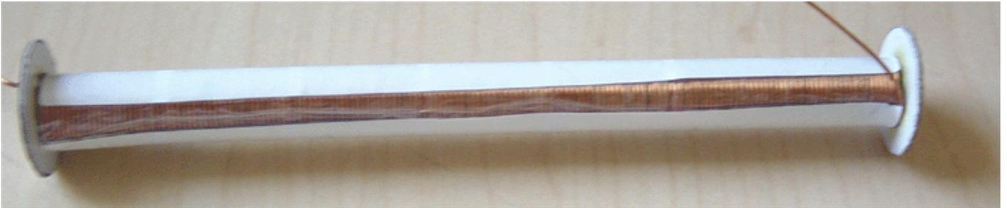
You now have a perfectly wound first layer. Before starting the second layer, cut the next strip of paper, measuring 40 mm wide. Stick a strip of Selotape along the length of the paper, again, with half of the width of the Selotape overlapping the paper and set it aside. Wind the next layer in exactly the same way, finishing by sticking and securing the paper around the core with its two layers of wire.
