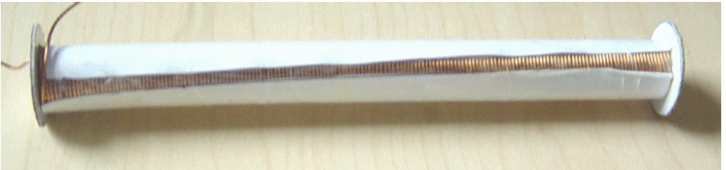
That process is repeated until all of the desired layers have been wound. Finally, the wire is cut with a few inches left for connecting the coil in the circuit, and the wire is passed through a second hole in one of the flanges:
