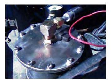
The lid can be finished off by drilling its centre to take the fitting for the aluminium pipe which will feed the output from the cell to the engine. This fitting, in common with every other fitting **must** be made of stainless steel. Video at <u>http://youtu.be/-7075bVmDQo</u>.
