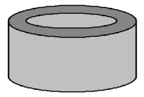
This core is then wound with thick wire - perhaps AWG #10 or 12 SWG (2.3 x 2.3 mm square wire) . The turns of wire should be tight, side by side and sit exactly flat on the top surface as the wire there will be contacted by the sliding brush:
