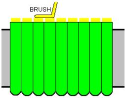
The sliding brass contact or "brush" is dimensioned so that it connects across two adjacent wires so that there is never any sparking as the brush contact slides around the circle of wires. The brush is driven by a small DC motor. In order for the sliding brush to contact the wire, the plastic insulation needs to be removed from the top half of the wire with the remaining insulation keeping the turns from
