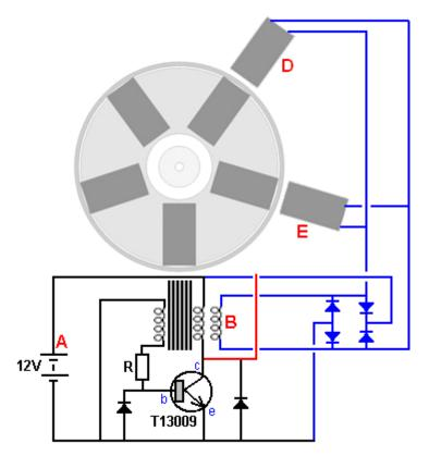
Coils "B", "D" and "E" are all triggered at the same time by three different magnets. The electrical energy produced in all three coils is passed to the four blue diodes to produce a DC power supply which is used to charge battery "A" which powers the circuit. That additional input to the drive battery caused by the addition of two more drive coils to the stator, makes the system operate securely as self-powered, maintaining the voltage of battery "A" indefinitely.
