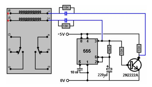
The capacitors shown in blue are chosen to operate the actual physical relay which is used in the circuit. They give the relay a brief switching pulse every five minutes or so. The 18K resistors across the capacitors are to bleed off the capacitor charge during the five minutes when the timer is in it alternative state.
