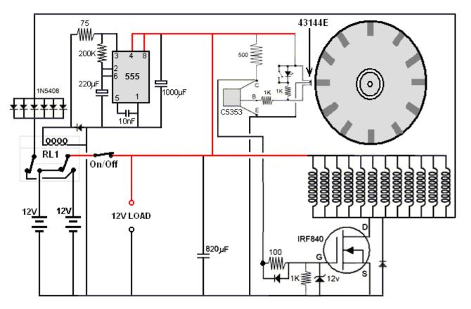
You will notice that the number of 1N5408 diodes has been doubled to allow an easier flow of increased current to the battery being charged. Please understand clearly that this last circuit is only a suggestion and has not been built and tested at the time of writing.
