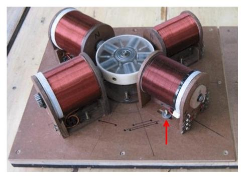
The red arrow draws your attention to the fact that the gap between the rotor and the coils can be adjusted by loosening the mounting bolts and sliding the coil along the mounting slots. The gap can be anything from 1mm to 10 mm.
