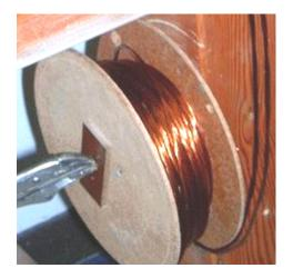
The next 3 metres of the three wires is now clamped and 80 turns applied to the central point, but this time the turns are applied in the opposite direction. Still the same 80 turns, but if the last length was 'clockwise' then this stretch of wire will be turned 'counter-clockwise'. This alternation of direction gives a finished set of twisted wires where the direction of twist reverses every 1.5 metres along the length. That is the way that commercially produced Litz wire is made.
