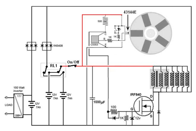
This circuit has a 150 watt continuous output and it uses three 12-volt batteries. The first two batteries are used, one to power the circuit while the second one is being recharged through three diodes wired in parallel to improve the recharging current flow. The two-pole two-way changeover switch "RL1" swaps the batteries over every few minutes using the circuit shown below. This technique keeps both batteries fully charged.
