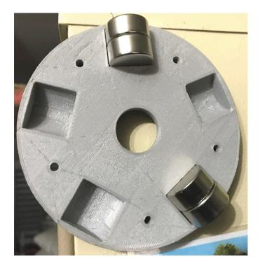
This one is made in two halves which are then bolted together.
