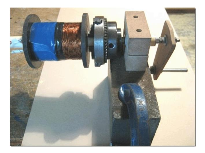
The three strands of wire which form coils "1", "2" and "3" are 0.7 mm diameter wire and they are twisted together before being wound into the coil "B". This produces a much thicker composite wire group which is easy to wind on to the spool accurately. The winder shown above uses a chuck to grip the coil core for winding, but any simple winder will work well.
