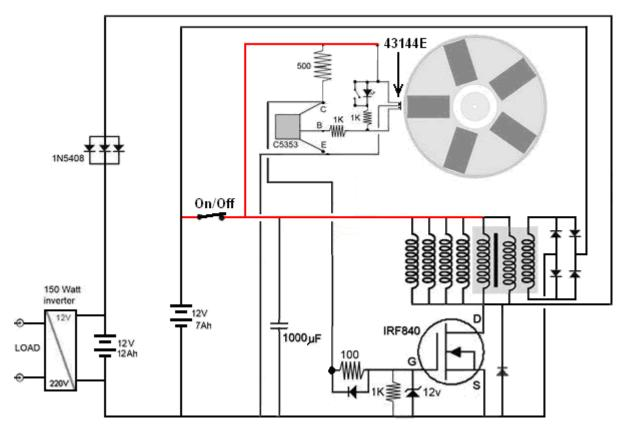
Here, the battery which powers the inverter which supplies the load is increased in capacity and while the developer used two of his 7 Amp-Hour batteries, you can use a standard 12-volt 12 Amp-Hour battery intended for a mobility scooter. All but one of the coils is used to supply current to the output battery and the one remaining coil, which is part of the three-strand main coil, is used to supply the drive battery directly.
