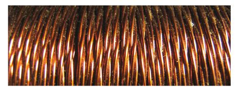
This completed coil now contains three separate coils in very close proximity to each other and that arrangement is excellent for inducing energy in the other two coils, when one of the coils is powered up. This winding now contains coils 1,2 and 3 of the circuit diagram. There is no need to concern yourself with marking the ends of each strand of wire as a simple ohmmeter will tell you which two ends have a connection between them.
