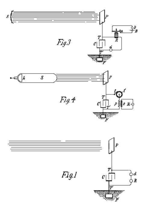
**Fig.1** shows the simplest form, in which **C** is the capacitor, **P** the insulated plate or conducting-body which is exposed to the rays, and **P'** another plate or conductor which is grounded, all being connected in series as shown. The terminals **T** and **T'** of the capacitor **C** are also connected to a circuit which contains a device **R** which is to be operated, and a circuit-controlling device **d** as described above.
