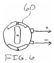
Fig.6 is a diagram of a DC motor that the pulse-charger of Fig.1 can drive according to an embodiment of the invention.
