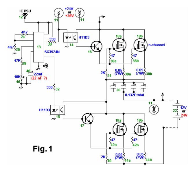
**Fig.1** is a schematic drawing of the solid-state pulse-charger according to an embodiment of the invention. As shown in **Fig.1**, the primary input energy source to the pulse-charger is a power supply **11**, examples of which are shown in **Fig.2**, **Fig.3**, and **Figs.4A-4D**. A 12-volt battery, as a low voltage energy source **12**, drives a dual switching means of control such as a logic chip or a pulse-width modulator (PWM) **13**.
