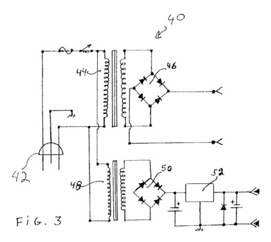
Fig.3 is a schematic drawing of a conventional AC power supply that can be used to provide power to the pulse-charger of Fig.1 according to an embodiment of the invention.
