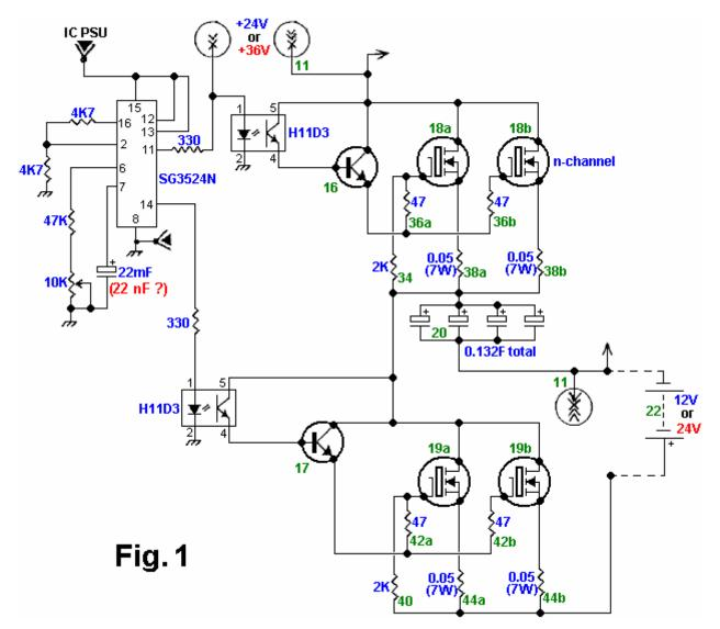
In addition to these SG3524N pin connections, it is suggested that pins 1, 4 and 5 be connected to ground instead of just pin 8, and that a 100nF capacitor be connected from pin 9 to ground. Pins 3 and 10 are left unconnected. The pinouts for the chip are:
