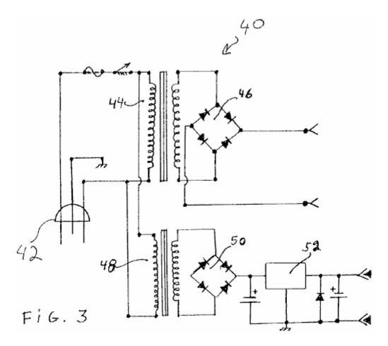
**Fig.3** is a schematic drawing of an AC power supply **40** that can be used as both the power supply **11** and the power supply **12** of **Fig.1** according to an embodiment of the invention. The power input **42** to the supply **40** is 120V AC. A first transformer **44** and full-wave rectifier **46** compose the supply **11**, and a second transformer **48**, full-wave rectifier **50**, and voltage regulator **52** compose the supply **12**.
