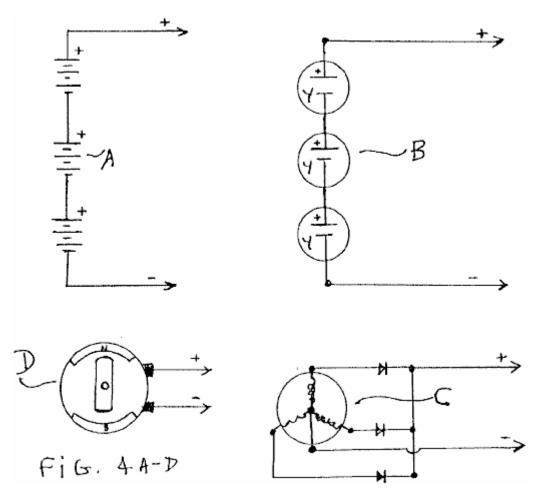
**Fig.4A to Fig.4D** are schematic drawings of other conventional power supplies that can be used to provide power to the pulse-charger of Fig.1 according to an embodiment of the invention.
