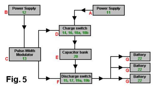
Fig.5 is a block diagram of the solid-state pulse-charger of Fig.1 according to an embodiment of the invention. Block A is the power supply 11, which can be any suitable power supply such as those shown in Fig.2, Fig.3, Figs.4A-4D. Block B is the power supply 12, which can be any suitable power supply such as
