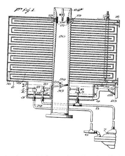
Referring now to the drawings, the numeral 1 indicates a main vaporising and atomising chamber for the liquid fuel located at the bottom of, and communicating with, a vapour heating and expanding chamber 2.
