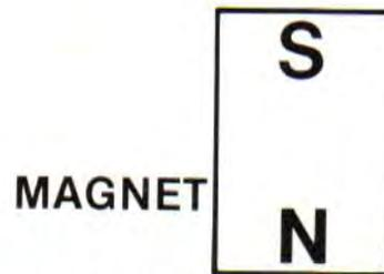
Current going one way in a conductor attracts one pole of a magnet — if current direction reverses, magnet is reversed.
