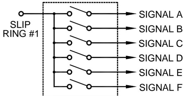
The rotary aluminum shaft wiper houses a spring loaded metallic "brush" that connects each contact to the slip ring in a sequential order. A second aluminum slip ring was installed, but was not utilized in the EMA4. If the slip ring were considered a circuit common then the timing pattern shown in Diagram 01 would be the result. Again not all of the contacts were used in either motor. This is indeed puzzling. Apparently different
