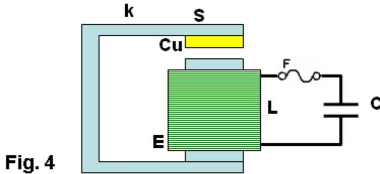
Here the spring is made of magnetic steel in the form of a U-shape. This U-shape also works as a magnetic guide.
