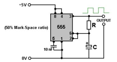
THE CAPACITOR HAS TO BE HIGH QUALITY WITH VERY LOW LEAKAGE IN ORDER TO GET THE OFF TIME TO EXACTLY MATCH THE ON TIME, AND WE WOULD LIKE THAT SO THAT THE TWO BATTERY PACKS GET IDENTICAL PERIODS OF RECHARGING.
