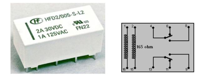
THIS IS THE ELECTRONIC VERSION OF A MECHANICAL TWO-POLE CHANGEOVER SWITCH. A BRIEF PULSE OF CURRENT THROUGH THE RELAY COIL CONNECTED BETWEEN PINS 1 AND 16 LOCKS THE SWITCH IN ONE POSITION, WHILE A BRIEF PULSE THROUGH THE COIL BETWEEN PINS 2 AND 15 LOCKS THE SWITCH IN THE OTHER POSITION. THE CURRENT DRAIN ON THE CIRCUIT WOULD BE ALMOST ZERO.
