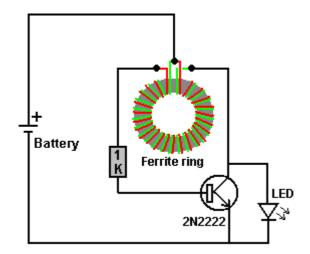
THE CIRCUIT OSCILLATES AUTOMATICALLY AND GENERATES A MUCH HIGHER VOLTAGE THAN THAT OF THE SUPPLY BATTERY, AND WHILE IT CAN MOST CERTAINLY LIGHT AN LED WHICH CAN'T BE LIT BY THE BATTERY ON ITS OWN, THE CIRCUIT CAN DO MUCH MORE THAN THAT.
