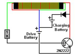
A SUITABLE COIL CAN BE WOUND QUITE EASILY. A PENCIL MAKES A GOOD FORMER FOR A COIL, SO A 100 mm WIDE STRIP OF PAPER CAN BE WRAPPED AROUND A PENCIL TO FORM A CYLINDER SEVERAL LAYERS THICK AND SEALED CLOSE WITH SELOTAPE:
