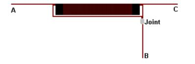
THE COIL NEEDS TO BE CHECKED CAREFULLY BEFORE USE. IDEALLY THE CENTRAL JOINT IS SOLDERED AND IF THE WIRE IS THE "SOLDERABLE" WIRE (WHICH IS THE MOST COMMON TYPE NOWADAYS) THEN THE SOLDERING IRON HEAT WILL BURN THE ENAMEL AWAY AFTER A FEW SECONDS, MAKING A GOOD QUALITY SOLDERED JOINT ON WHAT USED TO BE ENAMELLED WIRES.
