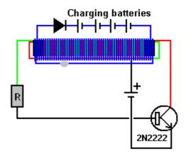
CURRENT DRAWN FROM THE SECOND WINDING DOES NOT AFFECT THE CURRENT DRAW OF THE DRIVE BATTERY WHICH IS RUNNING THE JOULE THIEF CIRCUIT.
