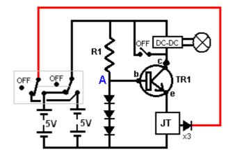
THIS CIRCUIT WORKS REALLY WELL. THE CURRENT FED TO THE DC-DC STEP-UP CONVERTER IS CONTROLLED BY THE VOLTAGE AT POINT "A" COMBINED WITH RESISTANCE OF THE JOULE THIEF CIRCUIT AS THE TRANSISTOR IS OPERATING IN EMITTER-FOLLOWER MODE. CONSEQUENTLY, THE VOLTAGE SUPPLIED TO THE JOULE THIEF CIRCUIT WILL BE ABOUT 0.7 VOLTS LOWER THAN THE VOLTAGE AT POINT "A".
