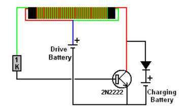
HOWEVER, THE CIRCUIT HAS A MINOR WEAKNESS IN THAT IF THE DRIVE BATTERY HAS A VOLTAGE GREATER THAN THE CHARGING BATTERY VOLTAGE PLUS THE VOLTAGE DROP ACROSS THE DIODE, THEN THE DRIVE BATTERY FEEDS CURRENT DIRECTLY TO THE CHARGING BATTERY THROUGH THE COIL WINDINGS AND WE DON'T WANT THAT TO HAPPEN AS IT JUST WASTES POWER. THAT WEAKNESS CAN BE OVERCOME BY PUTTING THE BATTERIES IN SERIES LIKE JOHN BEDINI DID:
