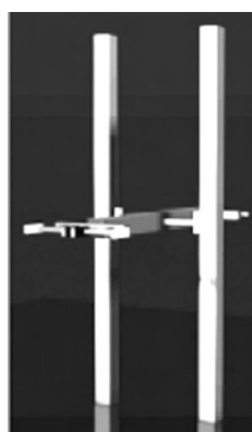
C) The A rotors have now reached their point of maximum centrifugal imbalance. The force at this point would be pulling the device to the left.
