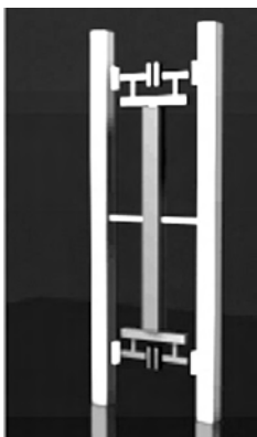
A) The upper rotors (designated from now on as the A rotors) are at the mass pickup point while lower rotors (B rotors) are at the mass drop off point. There is no shock during the weight transfer.
