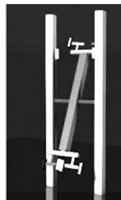
D) As the A rotors near the completion of this cycle, the B rotors are soon to begin it.
