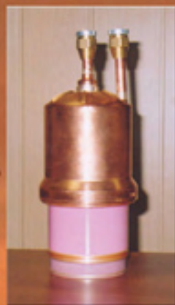
General view of a special diode produced for the present project. Its upper part is a water -cooling tank.
