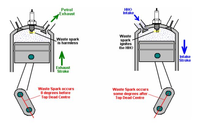
THIS LEAVES US WITH TWO ESSENTIAL ADJUSTMENTS – TIMING DELAY AND WASTE SPARK SUPPRESSION. THERE ARE VARIOUS WAYS THAT THIS CAN BE DONE BUT AS EACH ENGINE DESIGN IS DIFFERENT IT IS DIFFICULT TO COVER EVERY POSSIBILITY. HOWEVER, THERE IS A TECHNIQUE WHICH CAN BE USED WITH MANY ENGINES AND WHICH DEALS WITH BOTH ISSUES AT THE SAME TIME.
