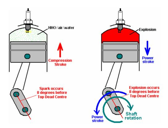
USING JUST AN HHO-AIR-WATER MIX, THE COMBUSTION WOULD OCCUR BEFORE TOP DEAD CENTRE AND MIGHT WELL BREAK THE CONNECTING ROD WHICH MOVES THE PISTON, SO WE NEED TO DELAY THE SPARK BY ABOUT TEN DEGREES.
