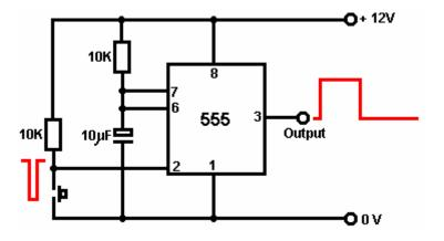
WE CAN USE TWO OF THESE CIRCUITS, THE FIRST TO GIVE THE NEEDED DELAY AND THE SECOND TO GIVE A BRIEF PULSE TO THE IGNITION CIRCUIT TO GENERATE THE SPARK :
