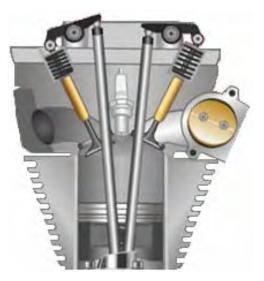
THE INTAKE VALVE (SHOWN ON THE RIGHT IN THIS ILLUSTRATION) IS PUSHED DOWN BY A CAM SHAFT, COMPRESSING THE SPRING AND OPENING THE INLET PORT. THIS ONLY TAKES PLACE EVERY SECOND REVOLUTION. IF A SWITCH IS MOUNTED SO THAT IT OPENS AND CLOSES WITH THE INTAKE VALVE (AND THE ORIGINAL SPARK TIMING WIRING REMOVED), THEN AN ADJUSTABLE ELECTRONIC CIRCUIT CAN SET THE CORRECT SPARK TIMING :
