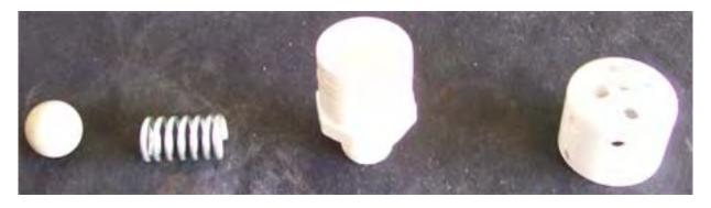
THE CAP IS DRILLED WITH HOLES AND THESE COMPONENTS ARE THEN ASSEMBLED TO PRODUCE A PRESSURE-RELEASE VALVE :
