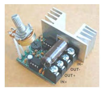
THE UNIT SHOWN HERE IS INTENDED TO PROVIDE UP TO 30 AMPS AND FANCIER UNITS ARE ALSO AVAILABLE.
