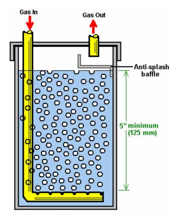
THE IDEA IS TO HAVE A WATER BLOCK TO PREVENT ANY ACCIDENTAL IGNITION OF THE GAS FROM PASSING DOWNWARDS THROUGH THE WATER. A LARGE NUMBER OF SMALL BUBBLES IS HELPFUL.
