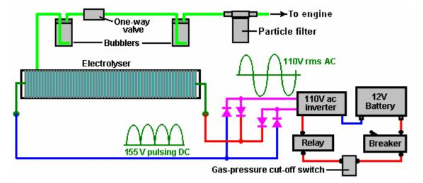
AS BOB IS AMERICAN, HIS DC INVERTER PRODUCES A NOMINAL 110-VOLTS AC WHICH RECTIFIES TO ABOUT 155 VOLTS OF PULSING DC. THIS ALLOWS AN ELECTROLYSER WITH 100 SEPARATE CELLS IN IT, (CREATED BY 101 ELECTRODE PLATES) TO BE USED. BOB'S PREFERRED PLATE SIZE IS 6-INCHES SQUARE (150 mm SQUARE). THE DC EFFICIENCY OF EACH CELL IS APPROXIMATELY 216% THAT OF MICHAEL FARADAY.
