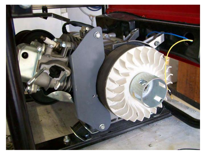
IN THIS PICTURE, THE FUEL INTAKE PORT OPENING IS OBSCURED BECAUSE IT HAS BEEN TEMPORARILY BLOCKED OFF DURING THE CONSTRUCTION.
