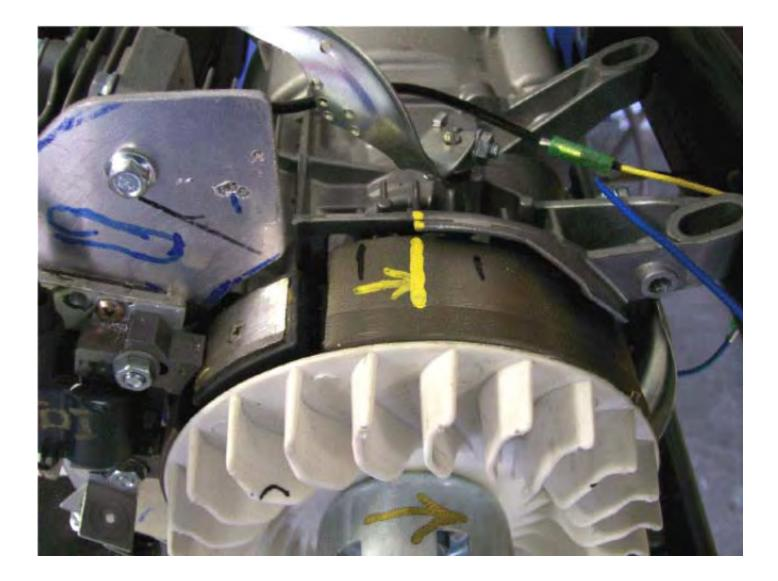
5. NEXT COMES A BIT OF ARITHMETIC. THE DIAMETER OF THE FLYWHEEL IS 180mm WHICH MEANS THAT ITS CIRCUMFERENCE IS 3.14159 x 180 = 565.5mm AND AS THERE ARE 360 DEGREES IN EACH ROTATION OF THE FLYWHEEL, THEN THE OUTSIDE EDGE OF THE FLYWHEEL WILL MOVE 1.57mm FOR EACH OF THOSE DEGREES.
