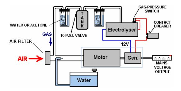
THE MAIN ADDITION IS TWO BUBBLERS BETWEEN THE ELECTROLYSER AND THE MOTOR OF THE GENERATOR. THESE ARE TO WASH OUT ANY SLIGHT TRACES OF ELECTROLYTE WHICH MAY HAVE CONTAMINATED THE HHO GAS GENERATED.
