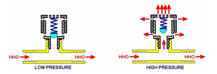
SELWYN ADDS AN ADDITIONAL SPRING-LOADED VALVE TO THE GENERATOR IN CASE THE ELECTROLYSER FAILS TO PRODUCE ENOUGH HHO GAS VOLUME. HE CALLS IT A "VACUUM RELIEF" VALVE BUT IT ACTUALLY OPERATES ON REDUCED PRESSURE RATHER THAN ON AN ACTUAL VACUUM. SELWYN USES A "HOGG" ELECTROLYSER (SHOWN IN CHAPTER 10) AND RECKONS THAT A HHO PRODUCTION RATE OF 4.5 TO 5 LITRES PER MINUTE IS SUFFICIENT TO RUN THE GENERATOR PROPERLY :
