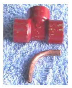
THE COPPER PIPE IS THEN HEATED WITH A PLUMBER'S GAS TORCH AND BENT VERY SLOWLY AND CAREFULLY TO THE SHAPE SHOWN ABOVE. SOME PEOPLE FIND IT HELPFUL TO INSERT A LENGTH OF SUITABLE FLEXIBLE MATERIAL, (SUCH AS THE COILED STEEL SPRING MATERIAL USED TO SUPPORT NET CURTAINS), BEFORE STARTING THE BENDING AS THAT HELPS TO KEEP THE COPPER PIPE FROM KINKING WHEN BEING BENT.
