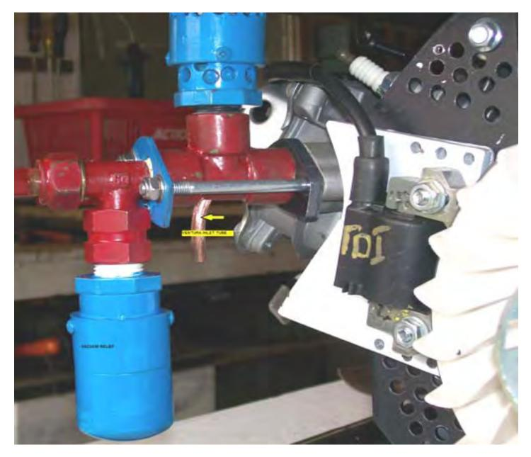
THE MANUAL PULL-START AND THE GENERATOR COVER ARE NOW REMOVED. IT IS ONLY NECESSARY TO UNDO FOUR OF THE BOLTS IN ORDER TO TAKE THE COVER OFF :
