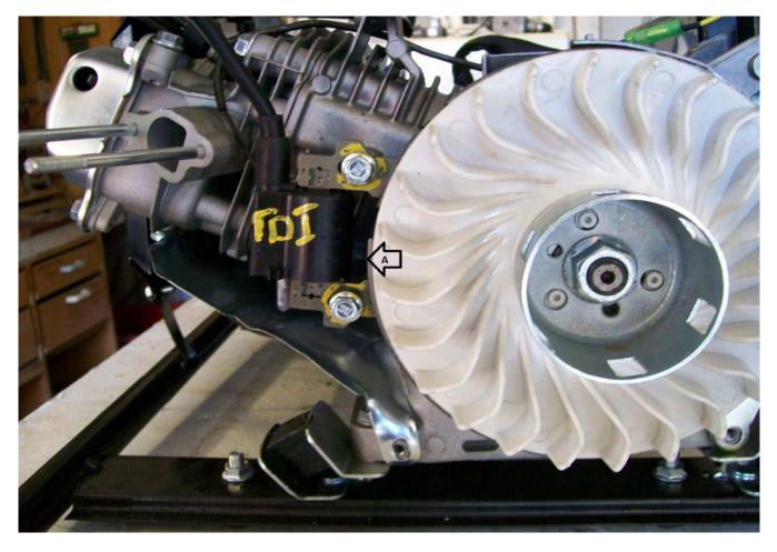
AT "A" YOU CAN SEE THE MAGNETIC PULSE TYPE TRANSISTOR DISCHARGE IGNITION ("TDI") PICK UP BOLTED IN PLACE IN ITS ORIGINAL 8-DEGREES BEFORE TOP DEAD CENTRE POSITION. THIS NEEDS TO BE REMOVED AND AN ALUMINIUM PLATE INSERTED TO ALLOW THE TDI TO BE MOUNTED IN ITS NEW POSITION. BECAUSE OF THE NEW FUEL, IT IS NECESSARY TO RETARD THE SPARK. TO MODIFY THE IGNITION TO TOP DEAD CENTRE. THIS IS SELWYN'S 2mm THICK ALUMINIUM ADAPTOR PLATE READY FOR THE TIMING CHANGE :
