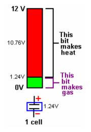
WITH 12 VOLTS APPLIED, 10.76 VOLTS DO NOT MAKE HHO GAS AND SO THE PROCESS IS ONLY ABOUT 10 PER CENT EFFICIENT AND 90 PER CENT OF THE POWER SUPPLIED ONLY HEATS THE WATER.
