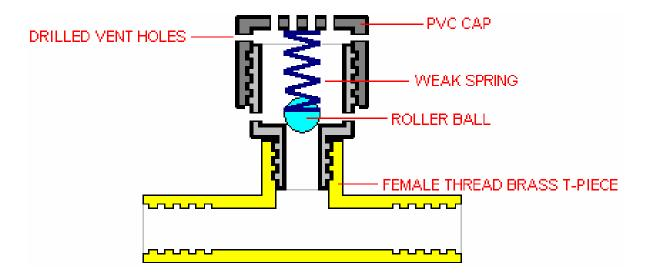
THE BALL IS HELD IN PLACE BY THE SPRING ALLOWING HHO TO FLOW PAST IT, BUT IF A SUDDEN INCREASE IN PRESSURE OCCURS THEN THE BALL IS FORCED UPWARDS, OPENING AN ESCAPE PATH THROUGH THE MANY HOLES DRILLED IN THE PLASTIC FITTINGS :
