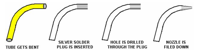
THIS VENTURI TUBE IS TO BE INSERTED INTO THE LAST BRASS FITTING BEFORE THE ENGINE, SO A 6mm DIAMETER HOLE IS DRILLED THROUGH THE BRASS AND THEN THE DRILL IS REMOVED VERY SLOWLY AT A SLIGHT ANGLE – THE ANGLE OF DRAG IS ALONG THE AXIS OF THE BRASS FITTING. THE COPPER VENTURI TUBE IS INSERTED THROUGH THE HOLE AND POSITIONED SO THAT THE VENTURI HOLE IS EXACTLY ON THE CENTRAL AXIS OF THE BRASS FITTING AND THEN SOLDERED IN PLACE.
