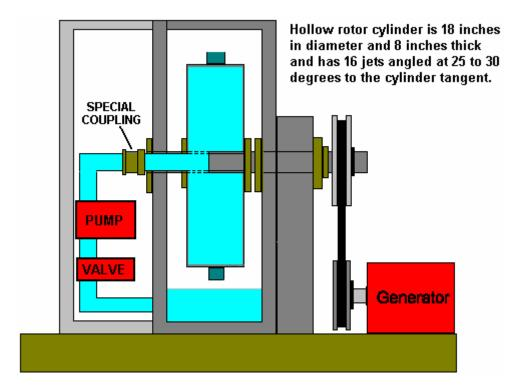
MOST GENERATORS NEED TO BE SPUN AT 3000 RPM OR SLIGHTLY FASTER. THAT SPEED CAN BE ACHIEVED BY BELT GEARING BETWEEN THE MOTOR'S OUTPUT SHAFT AND THE GENERATOR'S INPUT SHAFT. A GENERATOR OF THAT GENERAL TYPE COULD LOOK LIKE THIS 6.5 KVA UNIT COSTING £325 IN 2017:
