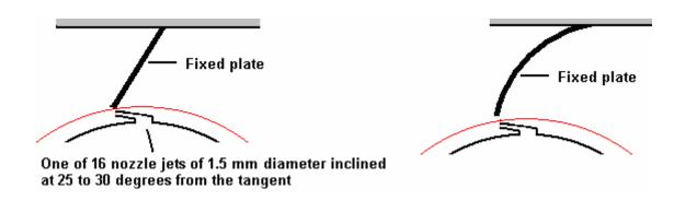
THE CURVED PLATE VERSION IS THEORETICALLY MORE EFFICIENT BUT THE DIFFERENCE IS SO SLIGHT THAT FLAT PLATES ARE OFTEN USED. THE MOTOR CAN BE BUILT IN VARIOUS CONFIGURATIONS:
