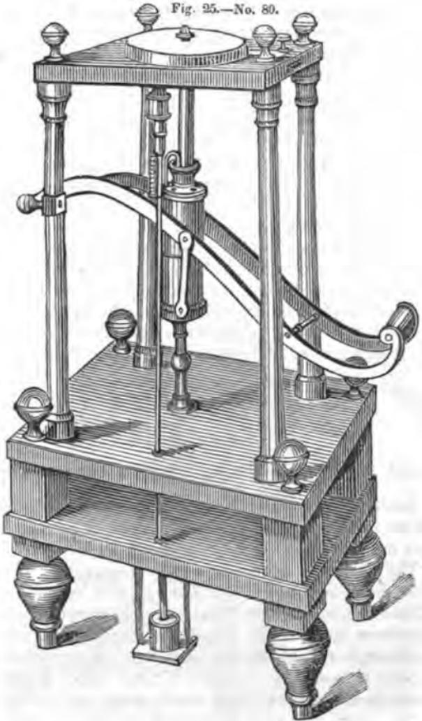
This Pump not only exhausts the Air, but from its peculiar construction, combines both the power of condensing and transferring Air or Gas, while at the same time, the accuracy of exhaustion and ease of operation is increased. This is produced
