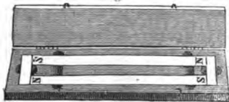
Fig. 1 represents a small case containing two bar magnets, with two short pieces of soft iron connecting their poles: these act as *armatures* (see § 9), and serve to preserve the power of the magnets. The magnets, when
