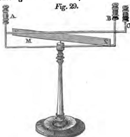
in fig. 29, it might be supposed that as the electricity which flows from C to A in the upper part of the wire, must pass in a contrary direction, in returning from A to B, below (the cup C being connected with the positive
