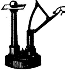
At Fig. 1 is shown a neat method of illustrating Inertia; a stiff card being projected by the spring without the Ball being removed from the Pillar.
