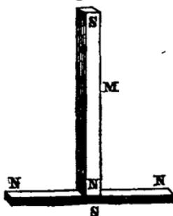
in the last experiment, and may be able to lift several iron screws or nails; the letters in the cut indicate the position of the poles.
