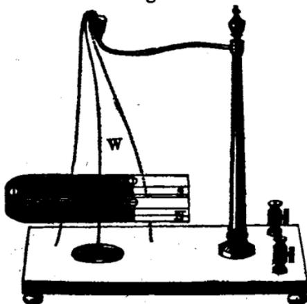
over a small basin for containing mercury excavated in the stand, by means of a brass arm supporting a mercury cup, in which the upper end of the wire rests: this mode of suspension allows it to vibrate freely, if its upper end is properly
