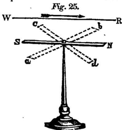
wire passing directly over and parallel to it. Of course, the direction of the wire must be north and south, as the needle will necessarily assume that direction, on account of the influence of the earth. If now the extremities of the wire are put in connection with the poles of a galvanic battery, in such a manner as to cause a current of electricity to pass through it, the needle N S will
