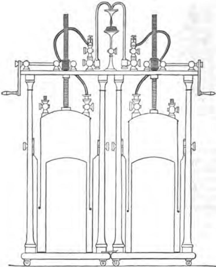
The above is a beautiful Oxy-Hydrogen Blow Pipe, on Hare's construction, made by me under the direction of Prof. B. SILLIMAN, for the Lowell Institute. The vessels are of copper, and the pressure is communicated by rack work, thus avoiding the trouble of heavy weights. The fixtures are of brass, and have every motion which may be required, and the whole operation
