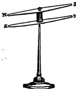
exerted upon the upper needle, will be counteracted by equal forces exerted in reverse directions upon the lower. It would be the same, indeed, with the influence exerted by the current of electricity, if the wire were to be placed in such a position as to act equally on both needles.
