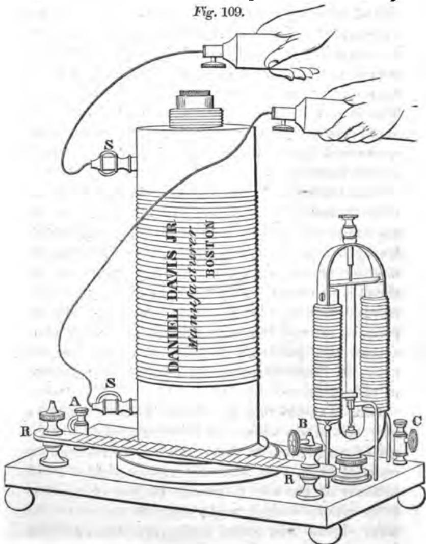
resented in fig. 109. When the battery wires are connected with the cups A and C, the current flows through the coarse wire coil, and also through Page's
