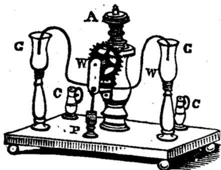
The glass cups are open at the bottom to allow the mercury to come in contact with the brass pillars into which they are cemented. These pillars are both connected with one of the binding screw cups C
