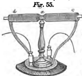
Fig. 55. polarity opposite to that of the ends. By reversing the direction of the current, all the poles will be reversed. The arrangement of the poles may be shown by passing a magnetic needle along the bar, or by small iron tacks, a large number of which will adhere to its extremities and to its middle.
