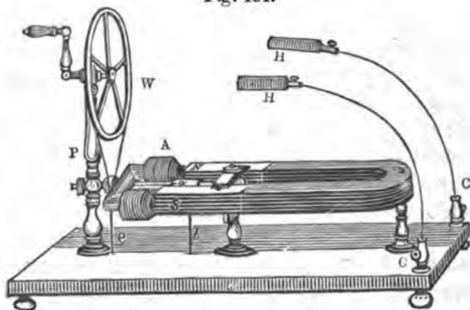
the iron instead of being curved is bent at right angles. It is a solid bar and not a bundle of iron wires as in the last described instrument. Around each pole of this armature is wound a coil of fine insulated wire; the two coils are connected so as to act as a single one. The armature does not quite touch the magnetic poles, and is mounted on an axis of rotation extending from the post P to the central support of the magnet. The upper
