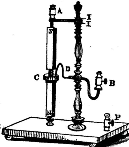
To the middle of the magnet is fixed a small ivory cistern C, for containing mercury, into which dips the end of the wire D. Thus the magnet is supported with its north pole downwards, and is free to
