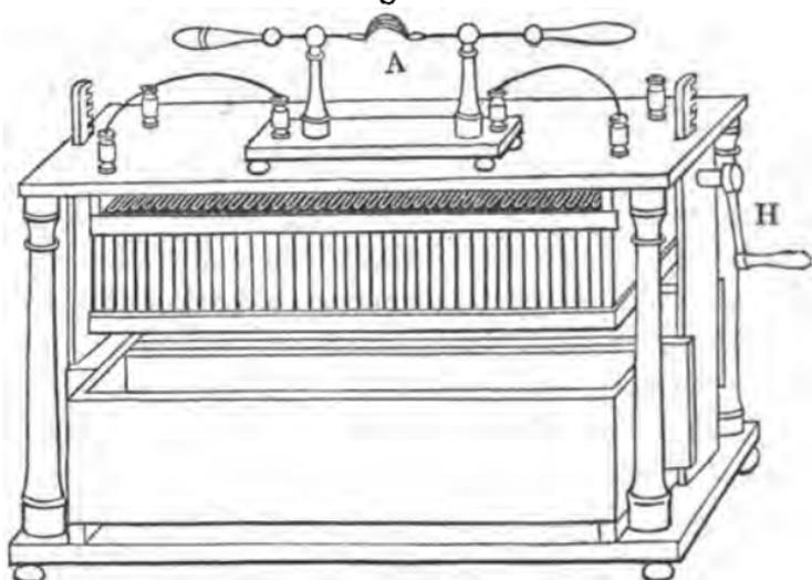
each having a separate trough to contain the acid. The plates are stationary, and the troughs are raised up to them by means of two racks moved by the crank and handle H, which lift the platform on which the troughs stand: either trough may be removed from the platform at pleasure, when it is wished to use only half of the battery.
