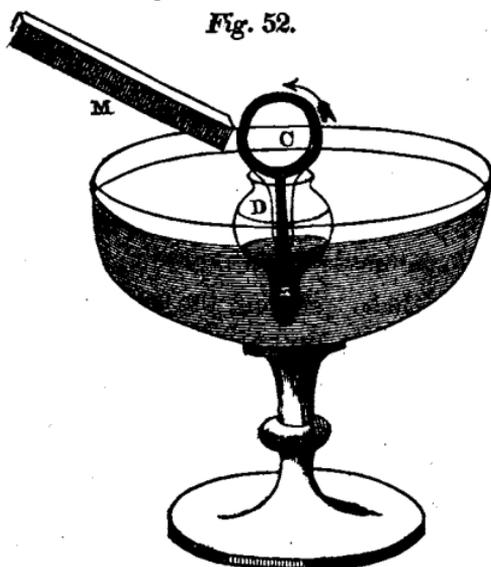
of communicating magnetism to iron or steel placed within it, but itself possesses magnetic polarity. This fact may be shown by means of the apparatus figured in the adjoining cut. One end of the wire forming the coil C is soldered to a very small plate of cop-
