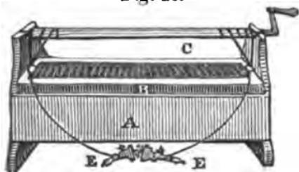
the surrounding copper by slips of wood at the edges, and connected by a strip of copper soldered to it, with the case belonging to the
