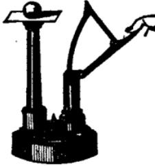
At Fig. 1 is shown a neat method of illustrating Inertia; a stiff card being projected by the spring without the Ball being removed from the Pillar.
