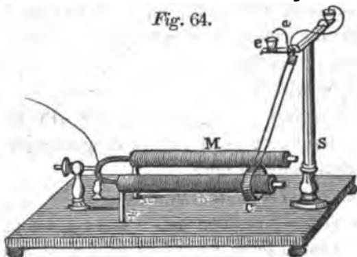
arm of the upright post S in such a manner as to allow it to pass along one of the poles of the magnet, the ring encircling the pole. On making communication with the battery, the coil will move over the pole towards the middle
