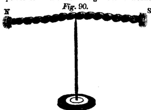
turn itself north and south, when balanced upon a pivot, as shown in fig. 90; the end which was downwards being its north pole.
