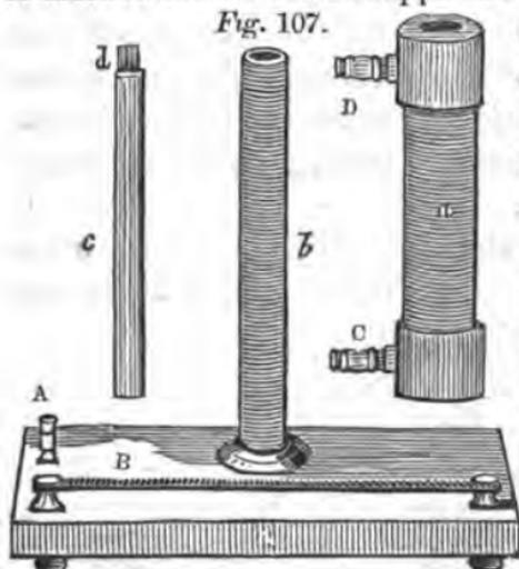
five feet long. The similar extremities of these wires are connected at one end with the cup A, and at the other with the steel rasp or break-piece B. If one wire of a galvanic battery be fixed in the cup A, and the other be drawn over the rasp, sparks will be seen ;
