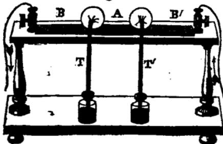
consists of three bars, two of bismuth and one of antimony, arranged as seen in the figure, where the antimony is shown at A, and the two bars of bismuth at B B', the bars being soldered together under the bulbs of two air thermometers, T and T'; a little cavity being made to receive the bulb of each thermometer; a drop of water is put in each cavity, in order to facilitate the conduction of heat from the metals to the thermometers.
