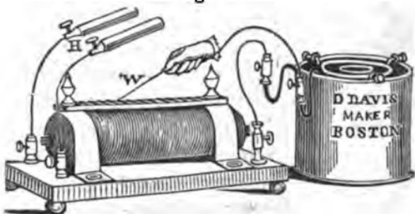
purpose is that represented in fig. 114. It consists of a double helix into which a bundle of iron wires can be inserted. The inner helix is composed of two or more
