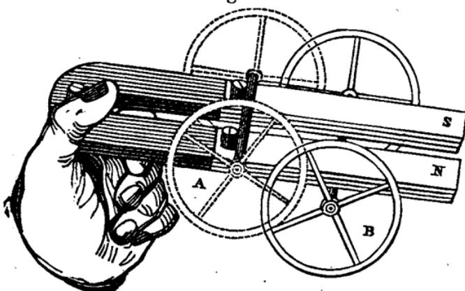
the breadth of the magnet, so that when applied to it the extremities may project a little beyond its sides. To each of these extremities a small fly-wheel is attached.
