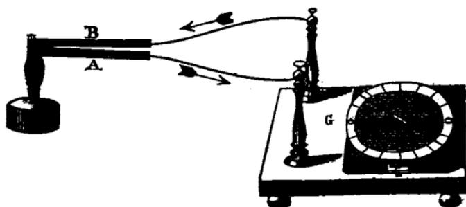
close proximity to a coil of wire, above which is fixed a graduated circle, the direction of an electrical current made to pass through the wire is indicated by the deflection of the needle from the north and south line, in one direction or the other, and its strength is measured by the number of degrees to which it is deflected. The *deflection of the needle* will be frequently
