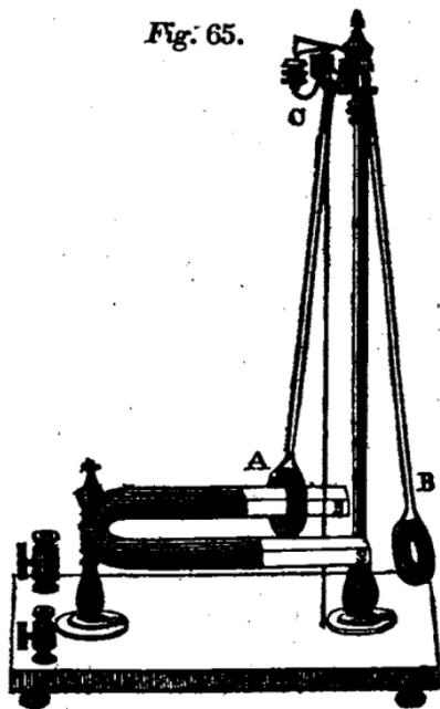
instrument represented in fig. 65 two coils *A* and *B* are employed, with a steel magnet. One end of the wire forming each coil is so bent as to dip into mercury contained in the cup *C*, when the ring hangs freely; and to be raised out of the mercury when it moves over the pole. The double wire, by which one of the coils is suspended, is somewhat longer than that which sustains the other, its axis of motion being higher in
