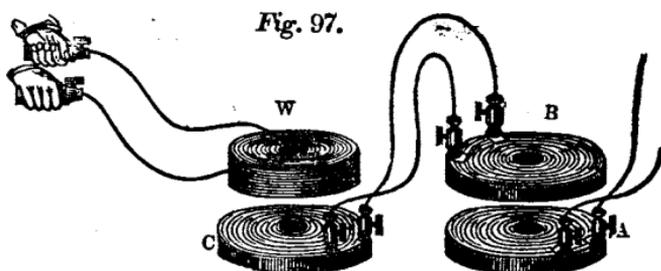
A. The secondary current induced in B will now flow through C, and if a fine wire coil W is laid on C, strong shocks may be obtained. If W be raised up, the shocks will still be felt when it is at a considerable height above C.
