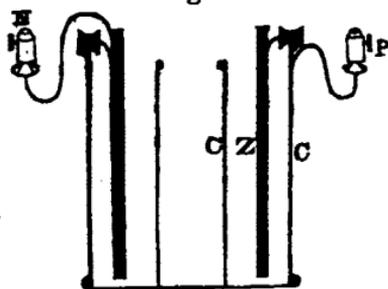
This battery, a vertical section of which is represented in fig. 7, consists of a double cylinder of copper, C C, with a bottom of the same metal; which answers the purpose both of a galvanic plate and of a vessel to
