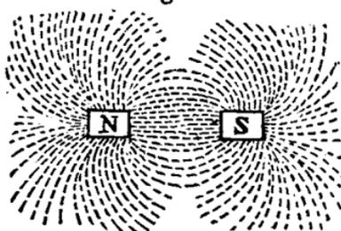
sand over a sheet of paper, and place a powerful horse-shoe magnet vertically beneath it, with the poles very near to the paper. The dotted lines in the cut (fig. 24) show the arrangement which the particles of iron will assume. Each one
