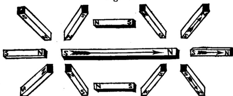
By passing such a needle carefully around a bar magnet it will be found that it will assume positions in relation to it, as represented in the above cut, fig. 23.
