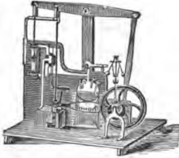
Fig. 15 represents a Section Model of the Steam Engine, as made by Watt. All the internal structure is shown, and the parts put in motion by turning the crank of the Fly wheel. It also illustrates the high and low pressure principles. This has been much preferred by teachers to a working model, not only on account of its low price, but perfect illustration. Prices \$12.00 to \$25.00.
