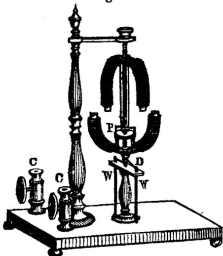
freedom of motion. The lower semicircle is supported by a pivot entering the upright pillar below it; its own axis is hollowed to receive the pivot on which the upper semicircle revolves. At D, in the figure, is seen a contrivance for conveying the current in a constant direction, of the same
