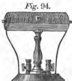
consist of a single length of wire, but wound so as to form six or eight layers of coils, to enable it to be used for examining currents of considerable intensity. Its power will be greater if its internal diameter is very small. In the cut, the helix C is mounted upon a stand, with a small piece of steel wire within it.
