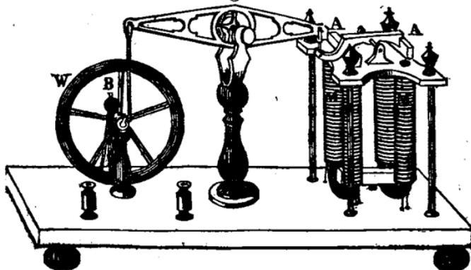
shaped electro-magnets, M M, fig. 79, are firmly secured in a vertical position on a stand, the four poles appearing just above a small wooden table. The two armatures,
