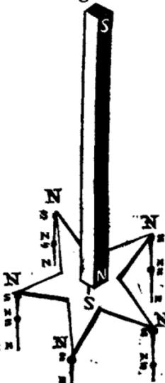
Exp. 17.—Place the north pole of a bar magnet M (fig. 42) on the centre of a circular plate of iron; it will now induce south polarity in the part immediately beneath it, and a weak north polarity in the whole circumference, so that it will sustain iron filings as shown in the cut.
