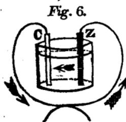
the zinc, through the liquid between them; as is shown in the adjoining cut, fig. 6, which represents a vessel of some non-conducting substance, as glass, partly filled with the fluid, and containing a zinc plate marked Z, and one of copper, C. Now the supposed motion of the electric current within the vessel is from Z to C;
