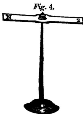
10. **MAGNETIC NEEDLE.** A light and slender magnet, mounted upon a centre of motion, as in fig. 4, so as to allow it to traverse freely in certain directions, is called a *magnetic needle*.
