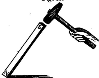
circumstances. Now strike the end of the bar with a hammer, as represented in fig. 89, and the pole will be instantly repelled. The polarity thus induced will not be reversed by merely inverting the rod, but the aid of percussion will also be required, in order to remove or reverse the magnetism.
