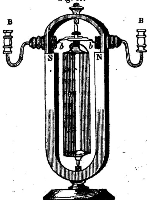
of wire C, fig. 69, being substituted for the ring. The rotation is much more rapid in consequence of the proximity of the rectangle to the magnet, not only near
