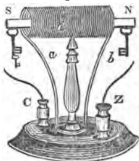
120. **HELIX, ON STAND.** The magnetizing power will be greatly increased if the wire be coiled in the manner of a cork-screw, so as to form a hollow cylinder into which the body to be magnetized can be inserted. Such a coil is denominated a *Helix*; and is represented at *d*, fig. 48, mounted upon a stand.
