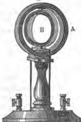
be made to produce a revolution analogous to some of those strictly called electro-magnetic; as in the instrument represented in fig. 92, which consists of a coil of insulated wire B fitted to rotate on a vertical axis within a larger one A, mounted on a brass pillar. The inner coil has a pole-changer fixed to its axis of motion for the purpose of reversing the current twice in each revolution.
