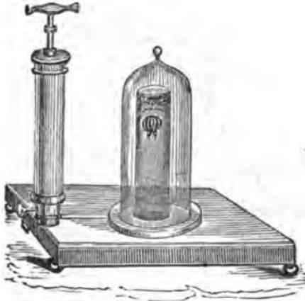
The Air Pump in this Set will exhaust or condense the air; the Barrel is  $1\frac{1}{4}$  inches in diameter, and mounted on a neat mahogany base, with brass clamp to secure it to the table. A great number of this Set have been sold, and in all cases given entire satisfaction for neatness and efficiency. The apparatus consists of
