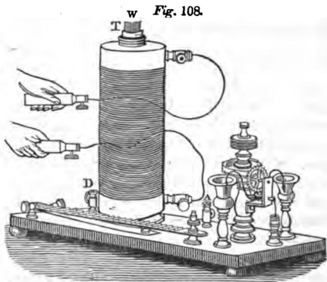
similar to that described in § 229, fixed on the same stand, in addition to the steel rasp. There are two cups A and D for the battery wires; these are connected through the electrotome with the inner coil. When the electrotome is made to vibrate, the curved wire dips its ends alternately into the cups of mercury, and rapidly breaks the circuit. One end of the coarse wire coil is also connected with the steel rasp, so that
