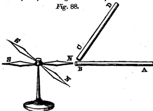
the needle, and which is the cause of its attraction. In fig. 88, A B represents an iron bar presented in this manner to the north pole of the needle. Now keeping the end B in the same place, raise the end A so as to bring the bar into the position C D. The north pole N will recede from C, as the bar is raised, as indicated by the dotted lines in the cut. The upper end of the bar D, on the contrary, will be found to attract N, and repel S. These
