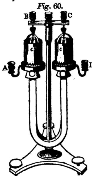
145. REVOLVING CYLINDER. This instrument is on the same principle as that last described, and the motion takes place in the same manner: the only difference being that two light copper cylinders *c c*, fig. 60, are substituted for the wire frames. These cylinders are serrated at their lower edge, as shown in the figure, to lessen the friction which they experience in moving through the mercury. The cups for battery connections are lettered in correspondence with
