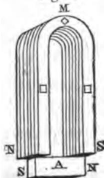
**COMPOUND HORSE-SHOE MAGNET.** A magnet composed of several horse-shoe magnets joined together, side by side, as in fig. 3, for the purpose of increasing the power, is called a *compound horse-shoe magnet or magnetic battery*. These magnets are charged separately, and are put together with all the similar poles in the same direction.
