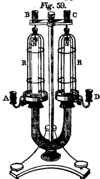
Fig. 59. The lower extremities of the wires dip into mercury contained in two circular cisterns sliding on the arms of the magnet. Bent wires passing from the interior of the cells support the cups A and D; and the cisterns themselves are fixed at any required height by means of binding screws attached to them. Each of the wire frames
