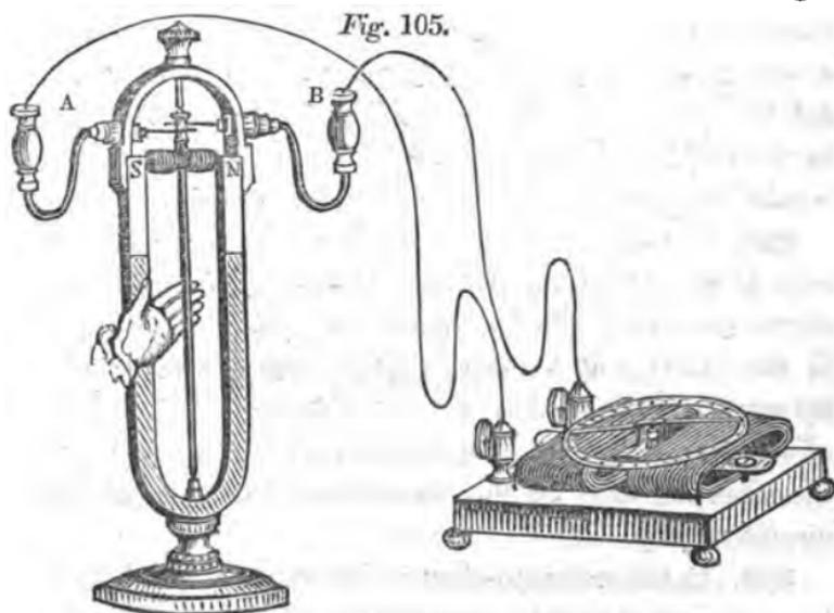
neto-electric machine in its most simple form. A soft iron bar capable of revolving between the poles N S of
