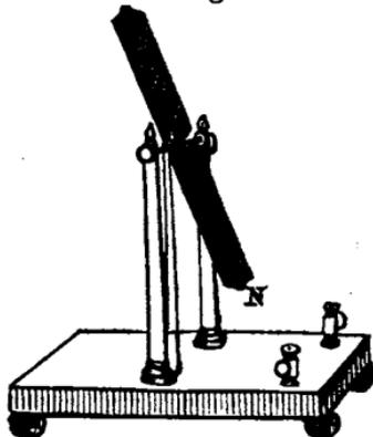
178. MAGNET REVOLVING BY THE EARTH'S ACTION. As the earth itself exhibits magnetic polarity, an electro-magnet may be made to revolve by its influence; though, in consequence of the feebleness of the action, the instrument must be constructed with some delicacy. A small electro-magnet N S, fig. 76, is so
