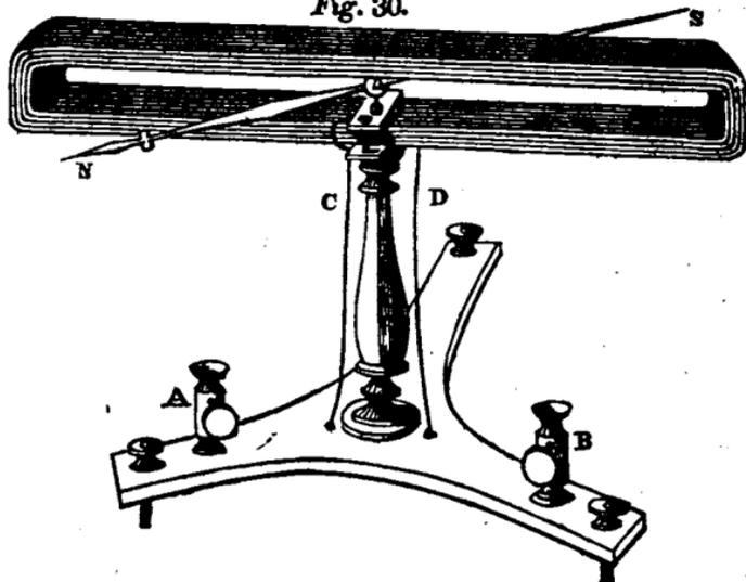
on a tripod stand, with leveling screws; the ends C and D of the wires being connected with the binding screw cups A and B.
