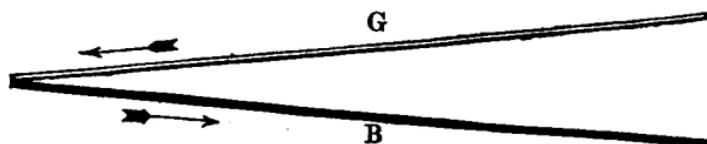
poles of the battery. In the cut, fig. 12, G represents the German silver, and B the brass; the direction of the current being indicated by the arrows.
