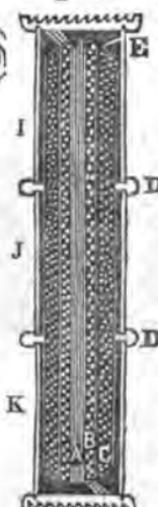
into three bands, insulated from each other by rings of ivory. At each end there is a circular rasp of steel attached to the metallic band nearest it. Fig. 113 represents a section of the instrument: A is the bundle of wires, B the battery coil, C the secondary coil, and DD the insulating rings of ivory. The similar strands of the battery coil are connected at one end with the
