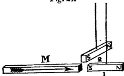
that the extremity *S* will be attracted by the north pole of the magnet, and the extremity *N* will be repelled by it, as has already been explained. Both these forces will conspire to retain the body in the direction represented in the drawing;
