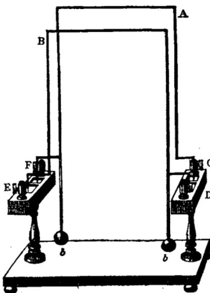
two oblong cells by a partition in the middle. Each of the four portions of mercury thus insulated, is connected by means of a wire projecting into the cell, with one of the binding screw cups fixed at the ends of the troughs. The points of two rectangular wires A and B rest in the opposite compartments of the troughs ; this mode of
