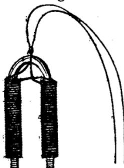
made in the U form, as shown in fig. 53, the bar being from six to eighteen inches in length before being bent. These, when connected with a medium size cylindrical battery, will sustain from a few pounds to fifty or a hundred pounds. A current from the thermo-electric battery (fig. 15), when transmitted through the wires of an electro-magnet, induces a considerable charge of magnetism.
