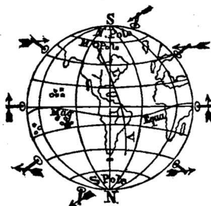
latitudes the directions exhibited in the annexed diagram, fig. 34, where the point of the arrow indicates the north pole and the feather the south pole of the needles placed around the globe. The angle which the needle makes with the horizon at any place is
