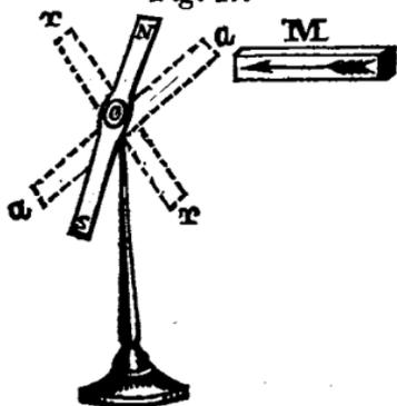
to its north pole the north pole of the bar magnet M. The north pole of the needle will be repelled, causing the needle to assume the position *r r*. If now the magnet M is reversed, so that its south pole is made to approach the north pole of the needle, the latter will be attracted, and the needle will be drawn to the position *a a*. The
