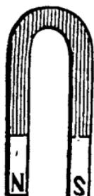
**8. HORSE-SHOE OR U MAGNET.** A magnet which is bent into such a form as to bring the two opposite poles near together, so that they may act simultaneously upon the same body, is called a *horse-shoe or U magnet*.
