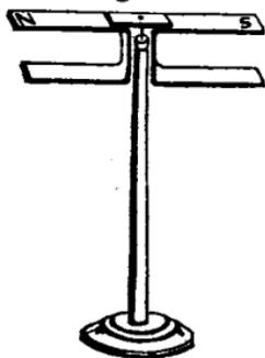
82. Fig. 28 represents another astatic needle, similar to the above, but consisting of two horse-shoe or U magnets united at the bend, so as to have their opposite poles in the same line, and delicately supported upon an agate cup. These needles need not be perfectly *astatic*, nor is it easy to make them so.
