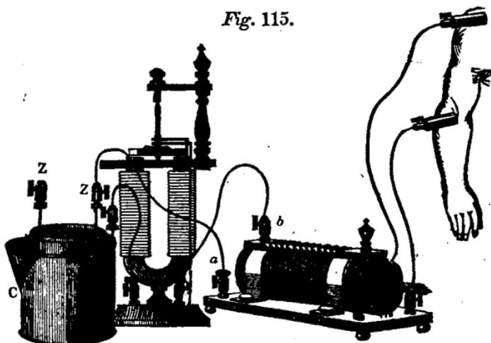
best instrument for the purpose, is seen in connection with the Double Helix. The galvanic current is transmitted through the two instruments in succession, by uniting one of the battery cups with one of those belonging to the Revolving Armature, whose other cup is connected with a cup *b* surmounting the Double Helix. The cup *a* on the stand is to be connected with the other plate of the battery.
