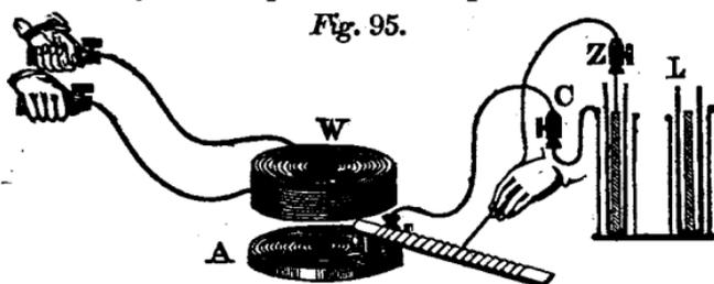
copper plate of a *sustaining battery*. A wire from the cup *Z*, belonging to the zinc plate, is drawn over a steel rasp resting on the other cup of the flat spiral, for the purpose of breaking the circuit rapidly.
