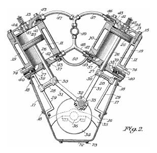
is a vertical transverse cross-section view through the compressor part of the engine. In his patent, Bob has avoided any direct mention of the fact that his engine design is fuel-less. That sort of statement is not popular with Patent Examiners even if it is perfectly true.
