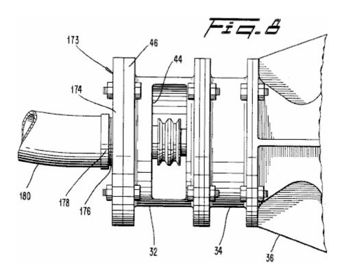
Fig.8 is a partial side view of the supercharger of Fig.1 with an adaptor .
