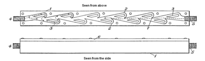
This arrangement is very clever as flow from right to left is free while flow from left to right results in a collision for every loop in the flow path. That is like this:
