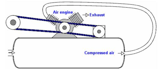
First, you have an ordinary air engine, supplied with compressed air from a pressure tank. This engine exhausts its (cold, expanded) air to the atmosphere. The engine powers two compressors which between them keep the tank full of compressed air.
