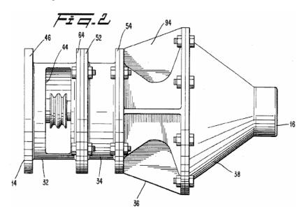
The front housing section 32 is a hollow cylinder which extends forward of a front bearing support 40. The front housing section 32 encloses the forward end 30 of the shaft 18 and the associated pulley wheel 28. At its forward end, the front housing section 32 defines the inlet 14 for receiving air from an external source (not shown).
