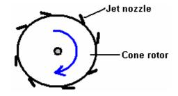
The operating pressure produced by the pump is 300 to 500 psi. Richard did not attempt to patent his engine as US Patent 3,697,190 "Truncated Conical Drag Pump" granted in 1972 as a liquid-asphalt pump is so close in detail that Richard felt that there was insufficient difference for him to be granted a patent:
