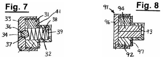
Fig.7 and Fig.8 are enlarged centreline sectional views of valve and plug assemblies for the gas loading port in the embodiments of Fig.1 and Fig.5.
