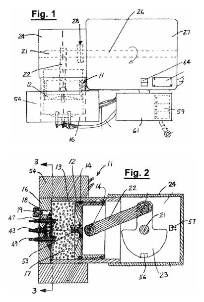
As illustrated in **Fig.1** to **Fig.3**, the engine **11** includes a piston **12** in a cylinder **13**, with rings **14** providing a seal between the piston and the inner wall of the cylinder. The upper or outer end of the cylinder is sealed by an end plate or head **16**, and an explosion chamber **17** is formed between the cylinder head and the piston. An inlet port **18** is formed in the cylinder head for introducing a charge of gas into the explosion chamber,
