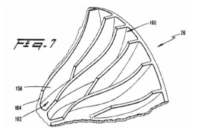
Fig.7 is a perspective view of a segment of the impeller of the supercharger of Fig.1; and
