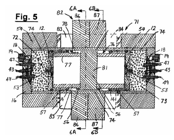
Fig.5 is a centreline sectional view of another embodiment of an internal explosion engine and generator incorporating the invention.
