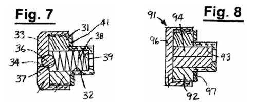
With the gas hermetically sealed within the engine, it is not necessary to replenish the gas as often as it would be if the engine were not sealed, and inlet port 18 can be closed with the plug assembly 91 of Fig.8 rather than the valve assembly 19 of Fig.7, if desired. Alternatively, a source of gas can be connected to the
