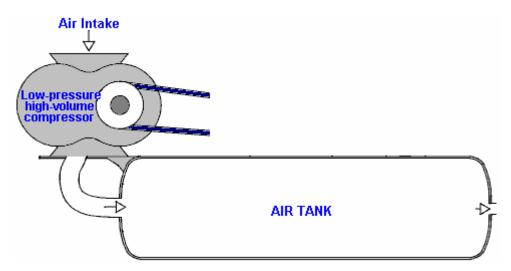
The first compressor is a simple 'leaf-blower' type which produces a large volume of low-pressure air. The big question is "how do you get this large volume of low-pressure air into a tank which has high-pressure compressed air inside it?". Well this seemingly impossible task is performed by the second compressor aided by a cunning, ultra-simple design:
