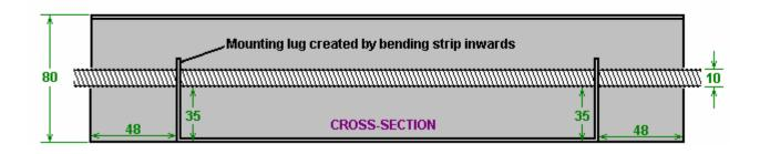
The inner cylinder is secured in position by two bolts as shown here:
