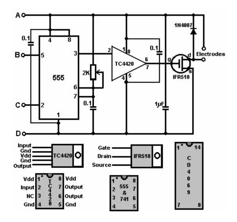
The output of the 741 integrated circuit is adjusted via its 2K variable resistor, to give an output voltage (at point 'B' in the circuit diagram) of 1 Volt when the car throttle is fully up, and 4 Volts when the throttle is fully down.
