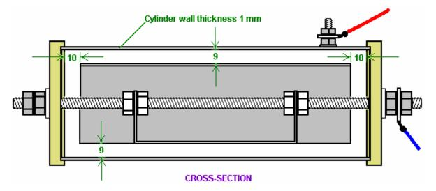
This gives a 9 mm clearance between the two cylinders and this gap stretches 360 degrees around the cylinders. The inner cylinder is located 10 mm clear of the Lexan end discs.
