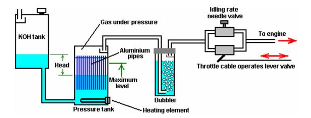
Here, there is a header tank containing a 25% mixture of Potassium Hydroxide (KOH) in water. This tank is positioned higher than the pressure tank where the hydrogen gas is generated and the venting pipe is protected by a baffle. The venting pipe should provide an outlet to the air outside the vehicle or building which contains the system.
