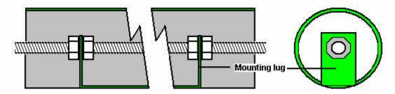
The inner nuts are manoeuvred on inside on of the lugs by hand and then the threaded rod is rotated to move one nut to the inside of the other lug, while the nearer nut is held to prevent it rotating. When the rod is positioned correctly and the inner nuts are pressed up hard against the lugs, then a box spanner is used to lock the outer nuts tightly against the lugs, forming a strong mounting lock.
