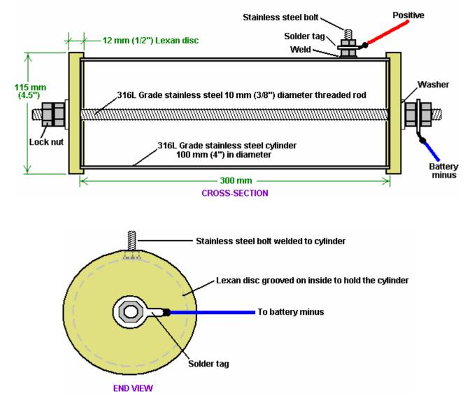
This basic container is modified in a number of ways. Firstly, a small 3 mm (1/8 inch) diameter air intake pipe is provided in one of the Lexan discs. This air intake is provided with a needle-valve which is screwed tightly shut for the early stages of testing and only eased slightly open when the engine is actually running.
