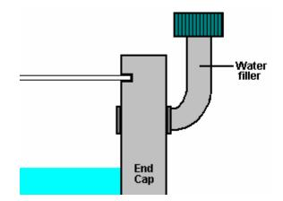
This arrangement has the advantage that it does not require a filler hole to be drilled through the steel cylinder.
