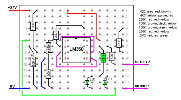
The 4.7K resistor and LEDs are only on the board for testing purposes and when the circuit is built in permanent form, then the LED chain connects to pin 1 of the jack socket so that the LEDs are disconnected during the two hours of daily treatment recommended when using the device.
