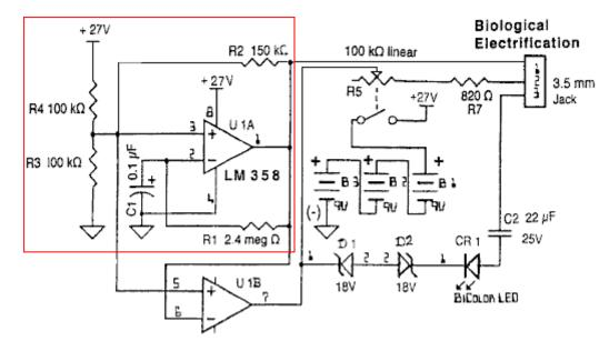
Bob states that the first section acts as a 4Hz square-wave signal generator, the frequency being controlled by the 2.4M resistor "R1" and the 100nF capacitor "C1". The data sheet for the LM358 states that the output voltage swing is between zero volts and 1.5V less than the supply voltage "Vcc" (which is +27V in this case). That implies that, as would be expected, the pin 1 output voltage from the first stage will switch sharply from 0V to +25.5V and sharply back again, four times per second.
